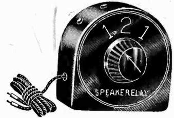
In home or store you often want to operate two speakers together, or each separately, and this speaker switch, the Speakerelay, does the trick! Connect the cord to the set and the speakers to the jacks in the switch. Turn knob at No. 1 at left to operate one speaker alone, to No. 2 to operate both speakers together, and to No. 1 at right to operate the other speaker alone. Enclosed in moulded Bakelite case. (Cat. No. 121).....\$2.00
