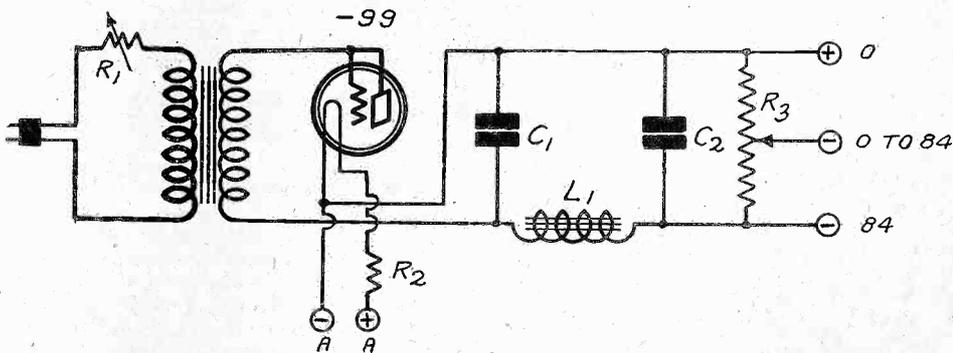
THE DIAGRAM OF A SIMPLE C BATTERY ELIMINATOR WHICH WILL SUPPLY THE HIGH BIAS REQUIRED FOR A -50 TUBE. THIS MAY BE BUILT INTO THE RECEIVER.
