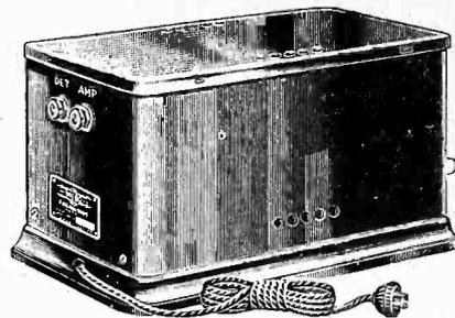
No. B16—"B" Eliminator for 50 to 60 cycle, 105 to 125-volt AC house current. Max. voltage, 180, with one variable detector and one variable intermediate voltage. Weight 16 lbs. Size, 6 x 6 1/2 x 11 1/2. Quiet, economical. Requires no attention. Sold only with Raytheon tube. Price, including Raytheon BH125 mil. tube and built in connector cord and plug.
