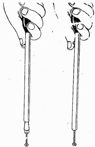
Push out the control lever with knob (as at left) and put wrench on nut. Push down on handle only (at right), then turn nut left or right.
