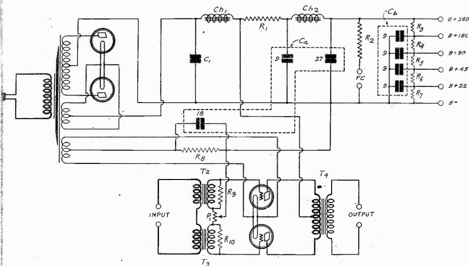
FULL-WAVE RECTIFICATION, WITH A PUSH-PULL AUDIO OUTPUT. THE TOTAL VOLTAGE ACROSS THE HIGH-VOLTAGE SECONDARY IS HALVED, BY USE OF CENTER TAP AS THE NEGATIVE LEAD. IN THESE SYSTEMS, FULL-WAVE RECTIFICATION AND PUSH-PULL AUDIO AMPLIFICATION, THERE IS CONSTANT ACTIVITY OF AT LEAST ONE TUBE. PUSH-PULL TUBES ARE ACTIVE ALL THE TIME.
