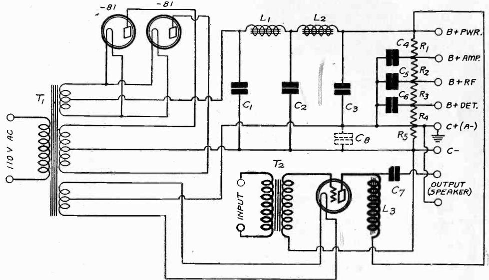
THE bleeder current is that current which flows independent of any plate current drawn by the tubes of a receiver. Thus any resistor across a potential difference will draw current, and this bleeder current exists whether the B supply consists of batteries or an eliminator. However, a bleeder across a battery is a sheer waste and useless. How about a bleeder across an AC B eliminator
