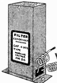
In B supplies, AC or DC eliminators, where there are several B voltage taps, by-pass each one with a 4 mfd. filter condenser and reduce ripple and common coupling of circuits. Connect one condenser from each B plus post to B minus or C minus. This done, you won't need any by-pass condensers in the radio receiver. The large filter condenser does all that a group of small by-pass condensers would do, and more!
