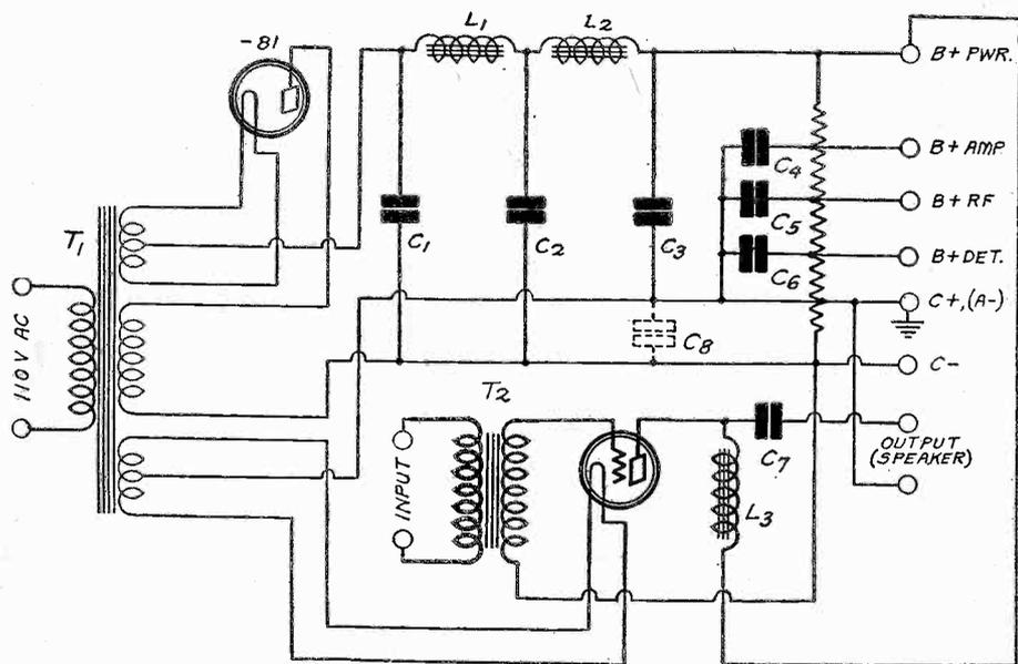
A HALF-WAVE RECTIFIER TUBE IS INACTIVE FOR EACH ALTERNATION (HALF CYCLE) AND ACTIVE DURING THE OTHER ALTERNATION. IT IS ACTIVE WHENEVER THE PLATE IS POSITIVE IN RESPECT TO THE FILAMENT, WHEN THE VOLTAGES ARE VIEWED IN VACUOUS SPACE. IN EXTERNAL PERFORMANCE THE PLATE IS ALWAYS NEGATIVE IN RESPECT TO THE FILAMENT. A SINGLE-SIDED AUDIO OUTPUT IS SHOWN
