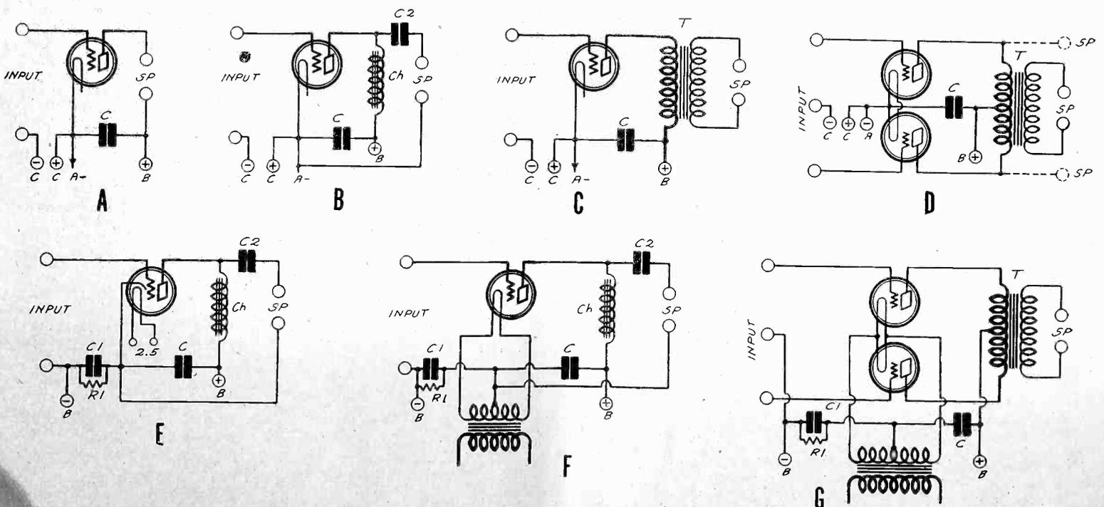
FIG. 9. THE THREE TYPES OF COUPLING BETWEEN THE POWER TUBE AND THE LOUDSPEAKER AS APPLIED TO DC AND AC TUBES. A—SPEAKER CONNECTED DIRECTLY IN THE PLATE CIRCUIT; B—THE OUTPUT FILTER WITH DC TUBE; C—OUTPUT TRANSFORMER WITH DC TUBE; D—PUSH-PULL OUTPUT TRANSFORMER WITH AC TUBES, AND THE PLATE-TO-PLATE CONNECTION; E—OUTPUT FILTER WITH HEATER TUBE; F—OUTPUT FILTER WITH AC FILAMENT TUBE; G—PUSH-PULL WITH AC FILAMENT TUBES.
