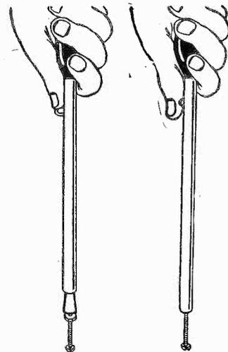
Push out control lever with knob (as at left) and put wrench on nut. Push down on handle only (at right), then turn nut left or right.
