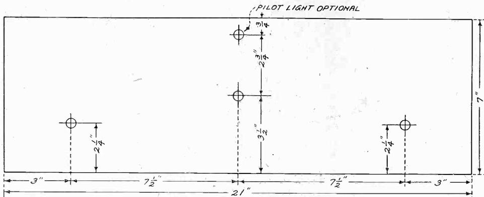
**DIMENSIONS FOR THE 7 X 21" FRONT PANEL USED FOR THE PUSH-PULL DIAMOND OF THE AIR. THE VOLUME CONTROL R1 AND SWITCH SW, CONSISTING OF A SINGLE COMPOSITE INSTRUMENT, ARE MOUNTED AT LEFT. THE TUNING CONDENSER IS AT CENTER, 3 1/2" UP. THE PILOT LIGHT, IF USED, IS ABOVE THE CONDENSER. AT RIGHT THE THREE CIRCUIT TUNER IS MOUNTED UPSIDE DOWN, THAT IS, WITH TICKLER COIL TOWARD THE SUBPANEL. THREE HOLES EQUIDISTANT AT BOTTOM MAY BE USED FOR ANCHORAGE TO THE SUBPANEL.**
