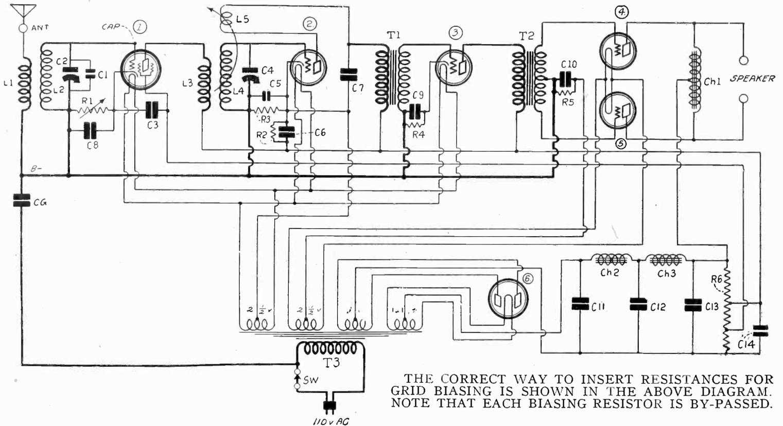
THE CORRECT WAY TO INSERT RESISTANCES FOR GRID BIASING IS SHOWN IN THE ABOVE DIAGRAM. NOTE THAT EACH BIASING RESISTOR IS BY-PASSED.
