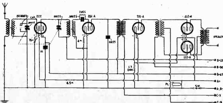
CIRCUIT DIAGRAM OF THE HB 22 FOR USING THE OPEN CONSTRUCTION TUNING UNITS. BOTH THE TUNING CONDENSER ROTOR AND THE PRIMARY IN THE PLATE OF THE RF TUBE ARE RETURNED TO B PLUS, UNDER THIS SYSTEM, BECAUSE THE CONDENSER ROTOR IS INSULATED FROM THE GROUNDED POTENTIAL BY USE OF A SMALL INSULATED SHAFT.
