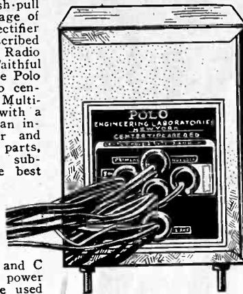
Polo 245 Filament Plate Supply (less chokes) has four windings, all save primary center-tapped (red), is 4 1/2" wide, 5" high, 4" front to back. Weight, 9 lbs. Filament windings, 2.5 v. at 12 amps., 2.5 v. at 3 amps. (for 245 filaments), 5 v. at 2 amps. for 280 rectifier, and 724 v. @ 100 m.a., center-tapped. Order Cat. PFPS @ \$7.50. [For 25 cycles order Cat. PFPS-25 @ \$12.00.] [For 40 cycles order Cat. PFPS-40 @ \$10.00.]
