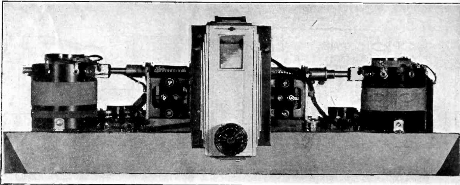
FRONT VIEW, SHOWS THE NATIONAL MODERNIST IC DIAL, WITH PEARL-LIKE SCREEN ON WHICH THE NUMBERS ARE READ. AT LEFT IS THE ANTENNA STAGE TUNING CIRCUIT. THE COILS USED ARE THE BERNARD TUNERS.
