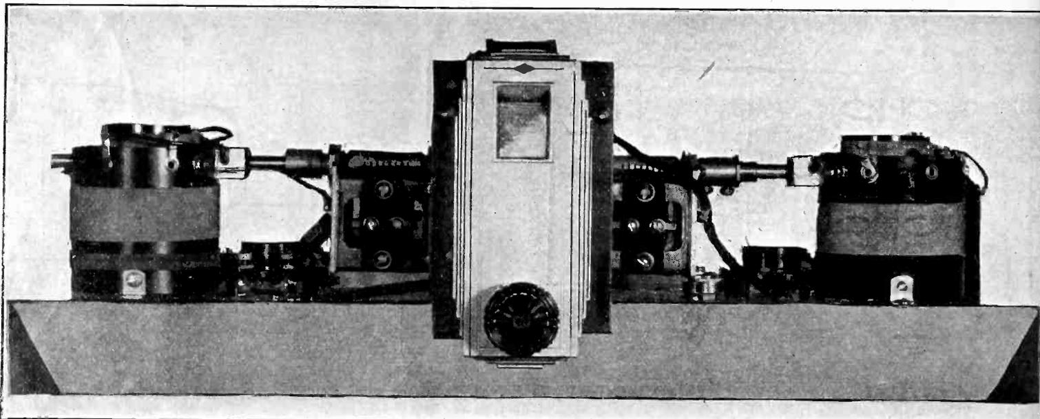
FRONT VIEW, SHOWS THE NATIONAL MODERNIST IC DIAL, WITH PEARL-LIKE SCREEN ON WHICH THE NUMBERS ARE READ. AT LEFT IS THE ANTENNA STAGE TUNING ARRANGEMENT, AT RIGHT THE INTER STAGE TUNING CIRCUIT. THE COILS USED ARE THE BERNARD TUNERS.
