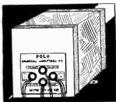
Polo Filament Transformer Only, four windings, consists of 50-60 cycles 110 v. winding, 2 1/2 v. at 12 amps., 2 1/2 v. at 3 amps., 5 v. at 2 amps. All windings, save primary, are center-tapped (red). Size, 4 1/2" high x 3 3/4" wide x 3" front to back. Weight, 6 lbs. Order Cat. PFT @ \$4.25. [For 25 cycles order PFT-25 @ \$7.00; for 40 cycles order PFT-40 @ \$6.25.]
