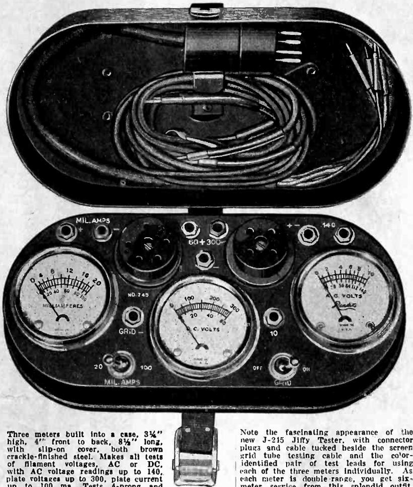
Three meters built into a case, 3 1/4" high, 4" front to back, 8 1/2" long, with slip-on cover, both brown crackle-finished steel. Makes all tests of filament voltages, AC or DC, with AC voltage readings up to 140, plate voltages up to 300, plate current up to 100 ma. Tests 4-prong and 5-prong tubes, including screen grid tubes. Test leads and instruction sheet included.
