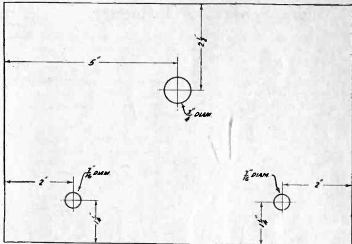
FIG. 4 FRONT PANEL, 7 x 10'', WITH HOLES MARKED
