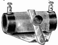
Remove aerial lead from set. Connect aerial instead to one of the binding posts of the Aerial Tuner. Connect the other binding post of the Aerial Tuner to antenna post of your set. Then move the lever of the Aerial Tuner until any weak station comes in loudest. The lever need not be moved for every different frequency tuned in. The Aerial Tuner acts as an antenna loading soil and puts the antenna's frequency at any requency in the broadcast band that you desire to build up. Price, 85c.
