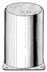
RF transformer in aluminum shield 2%" square at bottom, 3%" high. If metal subpanel is used no extra base is needed. Colls have brackets on. You must assemble in shield yourself and solder winding terminals to built-in lugs. For all circuits and stages, including screen grid tubes.
