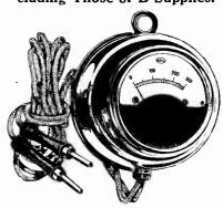
0-300 volts, at 200 ohms resistance per volt, 5 ma. drain at full-scale deflection. Accuracy, 2%. Case is full nickel finish. Long connecting cords have especially ornamental tip holders. Meter should be read in perpendicular position. Five-day money-back guaranty. Order Cat. F-300 @ \$2.59.
