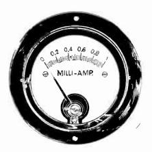
Here is a 0-1 milliammeter, accurate to plus or minus 1% clearly legible to two-one hundredths of a milliampere at any reading (20 microamperes). This expertly made precision instrument is offered at the lowest price so far for a 0-1 ma. Order Cat. FO-1 at \$5.95. C. O. D.
