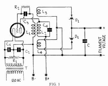
THE CIRCUIT OF THE OSCILLATOR, RECTIFIER, AND THE FILTER OF THE 25-KC RECTIFIED FILAMENT SUPPLY DEVISED BY HUGH A. BROWN AND LLOYD P. MORRIS.
