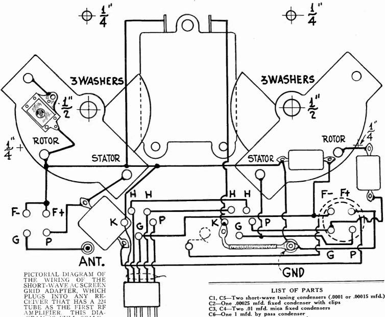
down when the correct relative position of the rotor is established. At rear is a bushing with set-screw built in, a butterfly lockwasher, a thumbscrew and a tightening nut. By adjusting the thumbscrew and tightening down the nut, then restoring the butterfly and set-screw device, the adjustment will be completed. The plates should
