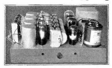
The H844, assembled, presents in compact form, on a  $17/2 \times 11/2$ " steel chassis, a completely AC operated shielded receiver, using four 224 screen grid tubes, one 227, two 245s in push-pull, and a 280 receifior, eight tubes all told. Here is the circuit that will bring 'em in from all over the country—and at a price you can 545.59. This price includes EVERYTHING except speaker, cabinet and tubes.
