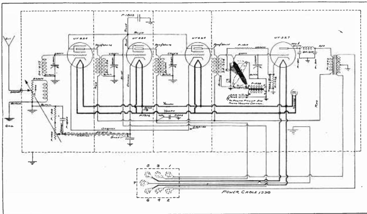
A transformer is supposed to be used between the phonograph pick-up unit and the terminals provided for the pick-up in the grid circuit of the detector tube.
