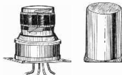
HIGH-GAIN shielded radio frequency transformers for screen grid circuits using 222, 224 or 232 tubes for RF, and any kind of detector. The primary has a high impedance—45 turns—and is closely coupled to the secondary over which it is wound, with an insulating wrapper in between, 42/10,000 inch thick. The diameter of the bakelite tubing is 1 1/4 inches.
