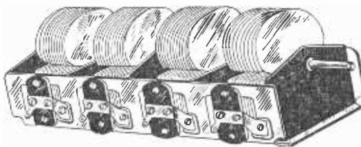
This condenser, each of four sections .00035 mfd., has aluminum plates that are removable and adjustable, also a 1/4" diameter steel shaft that is removable. It is sturdy and is suitable for popular four-circuit screen grid tuners. Trimming condensers are built in. The condenser may be mounted on its bottom or side. Total overall length, including shaft, 1 1/2". Overall width, 4". The frame is steel Order Cat. 4-G @.....
