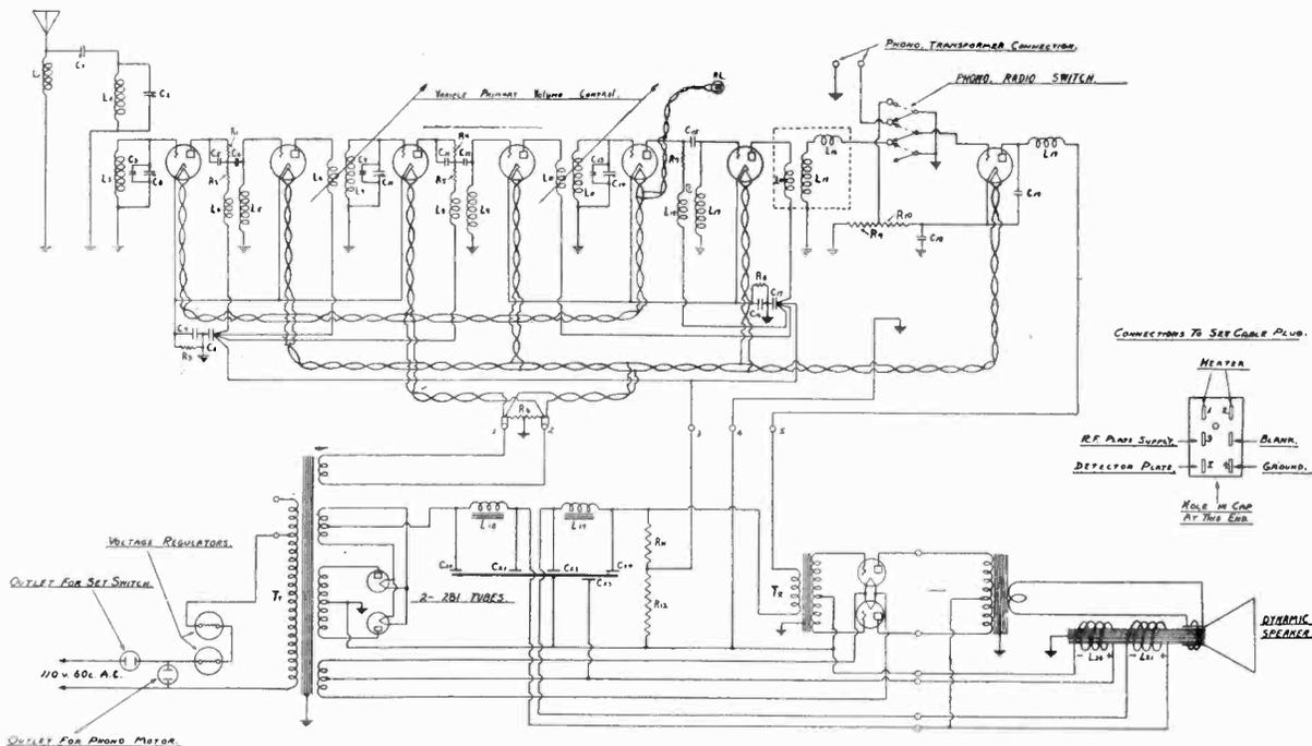
THE circuit diagram of Models R-20, R-25, R-30, and RP-40 "Star-Raider" of the Continental Radio Corporation is reproduced in Fig. 1 herewith. This circuit contains several features not contained in many other modern receivers.
