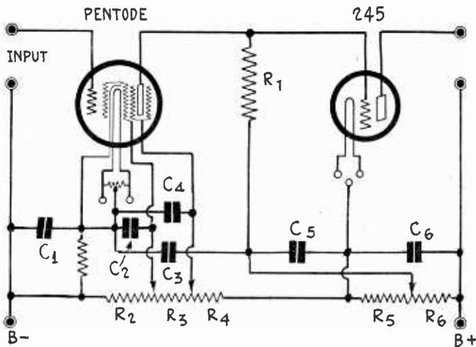
FIG. 868. THE PENTODE TUBE CAN BE USED IN THE LOFTIN-WHITE TYPE OF AMPLIFIER IN THE MANNER SHOWN IN THIS DIAGRAM.
