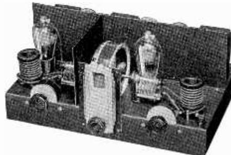
NATIONAL 5-TUBE THRILL BOX—A remarkably sensitive short-wave outfit, noted for reception of foreign stations. Uses 224 RF, 224 detector, 227 first audio, 227 push-pull second audio. A separate A and B supply is required. See below. Standard set of four pairs of coils included (21.2 to 2.61 megacycles). Humless operation, even on earphones. Single tuning control. No grunting, no backlash, no hand capacity. Order Cat. AC-SW-5, list price, less tubes, less B supply, \$79.50; net price \$46.74.
