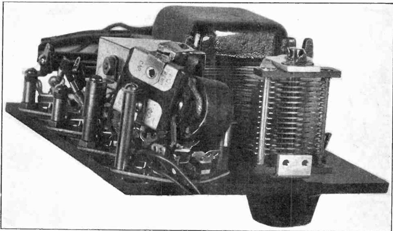
View of a short-wave converter with filament supply,
