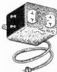
Connect relay's cable plug to 105-125 volt AC line. Connect B eliminator cable plug to relay socket so marked; connect trickle or other charger's plug to relay socket so marked; connect one side of A battery to binding post, other side to A set. Then turning on your set twins on B eliminator and turns off charger, turning off set turns on charger and turns off B eliminator.
