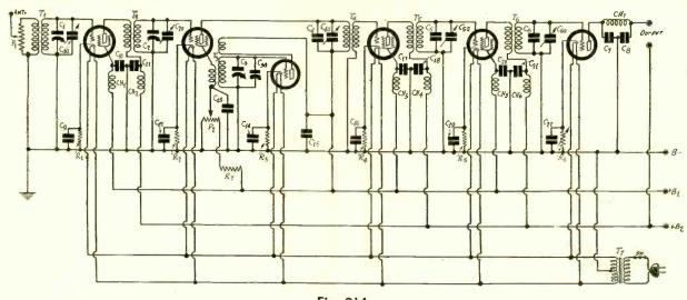
Fig. 914 A five-tube superheterodyne tuner and detector in which there is high selectivity in both the RF and IF frequency levels
