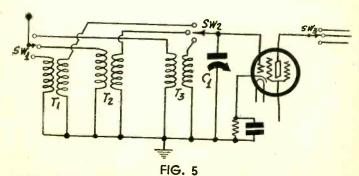
In this short-wave circuit coils of fixed inductance are used with switches provided so that any coil may be selected in the circuit. This is a good method.
