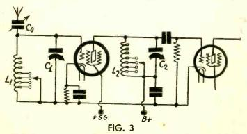
In this short-wave circuit tapped coils are used but turns are only shorted out of the tuning coils to increase the frequency range of the circuit.
