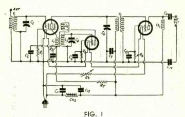
The circuit of a short-wave converter utilizing the new 6.3 volt heater tubes and deriving all its voltages from a DC line.
