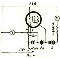
This is the circuit used in taking the curves in Figs. 1 and 2 on the sample 236 screen grid tube. When the curves in Fig. I were taken the 100,000 ohm resistance was short-
