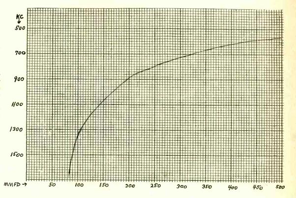
A curve showing the relationship between capacity and frequency, using a given precision type radio frequency transformer in a stated aluminum shield. The resultant inductance of the shielded coil was 160 microhenries
