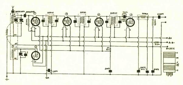
[Here is the diagram of the battery-operated counterpart of the AC short-wave tuner described last week, issue of April 25th... The coil data are completed and apply to both models.—Editor.]
