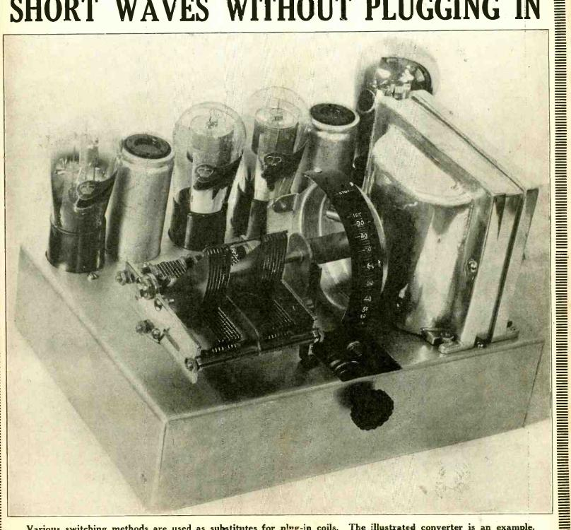
Various switching methods are used as substitutes for plug-in coils. The illustrated converter is an example. See pages 5, 6, 7 and 8. See pages 5, 6, 7 and 8.
