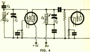
The tuning range of a short-wave receiver or converter may be extended by the use of variometers as in this circuit.
