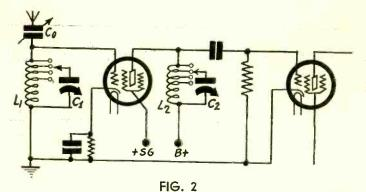
Tapped coils are used in this short-wave circuit for changing the wave-length range and the condenser is so connected that the part of the coil not tuned is used to step up the voltage.
