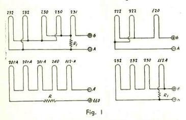
Four different combinations of filaments arranged to make the filament circuit in each case as efficient as possible
