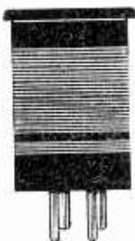
WOUND on 1.25 inch diameter finest bakelite forms, with flange for gripping, these short-wave plug-in coils afford high efficiency. Tube sockets serve as receptacles for these coils. The coverage with four coils is 13 to 200 meters with 0.00014 mfd. capacity. Also 0.00015 mfd. may be used without change. The coils may be used for any of the popular short-wave circuits.
