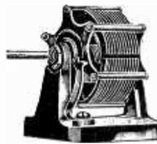
20 to 375 mmfd. capacity variation, effected over full 360 degrees, affords wide spreadout, better dial legibility. Great for test oscillators and all-wave tuning.
