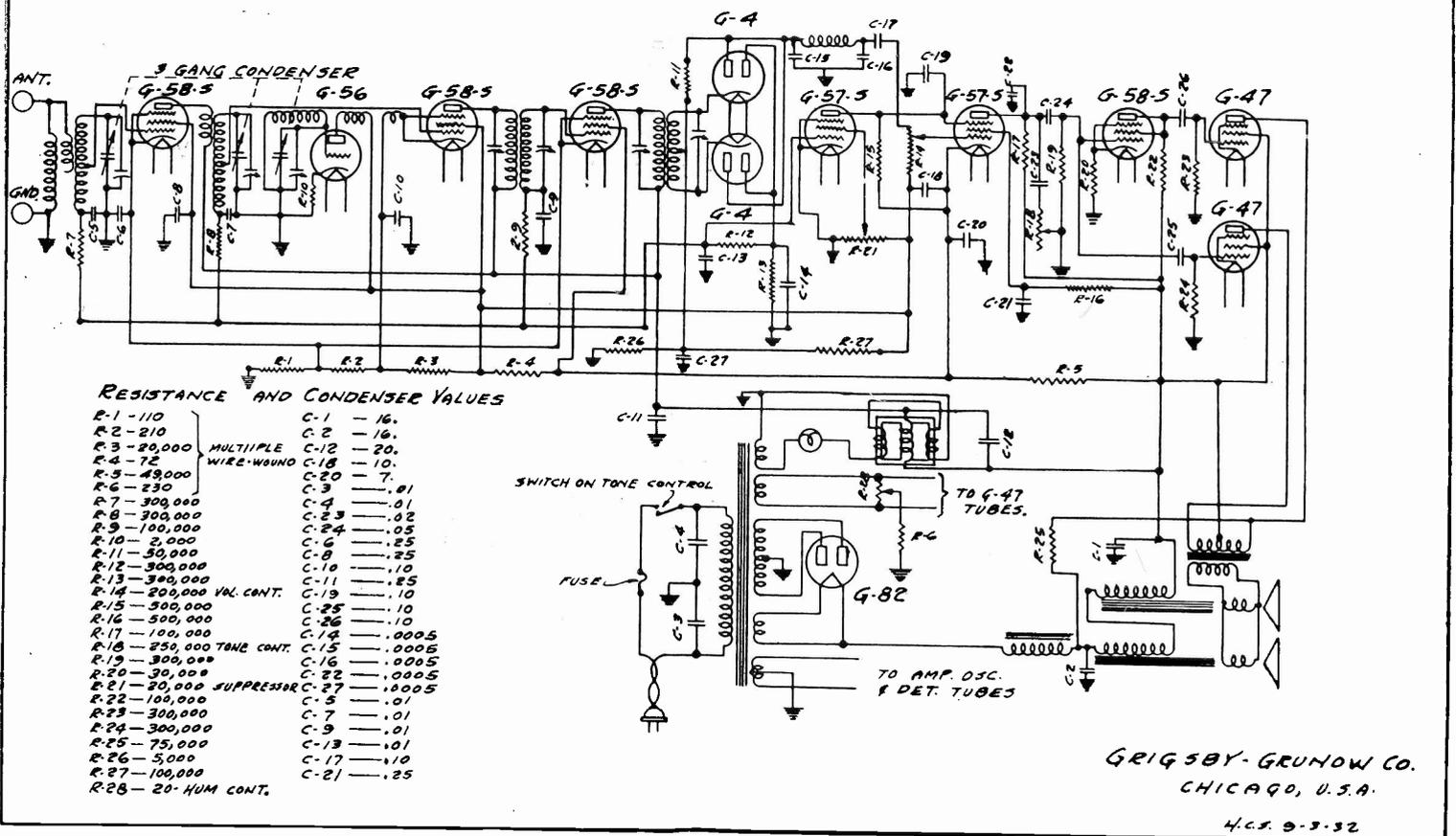
The model 320 Majestic chassis, diagram above, is used in the model 324 receivers. Model 320 circuit is identical with model 300 circuit except that 324 has delayed a-v-c.
