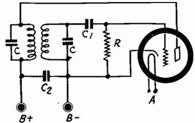
Top row, left to right: Fig. 1, a tuned grid oscillator circuit. This type is used in a large number of superheterodynes; Fig. 2, a tuned plate oscillator which is sometimes used in superheterodynes; Fig. 3, a simple modified Hartley oscillator that may be used when the oscillator is a heater type tube.
