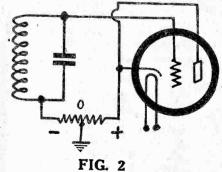
The direct current through the load resistor is pulsating, so if the center of the resistor is taken as the reference point, at any instant the extremes have equal but opposite signs.
