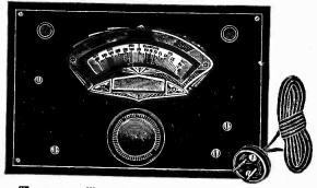
The test oscillator has a frequency-calibrated dial, 150 to 50 kc, with 1 kc separation between 50 and 80 kc and 2 kc separation between 80 and 150 kc. Intermediate frequencies are imprinted on the upper tier. Broadcast frequencies are obtainable on tenth harmonics (500 to
