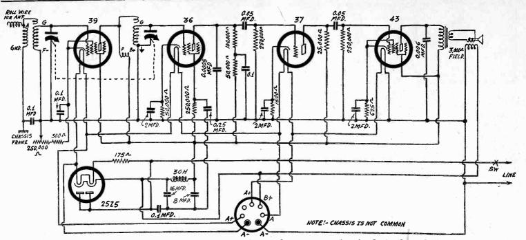
A five-tube universal receiver, using the 25Z5 as rectifier when a-c service is desired, and floating that tube on the line when d.c. is used. A precaution that should be taken is to observe polarity of connection to the outlet, so mark outlet and set plug, and warn the family to plug in the right way.
