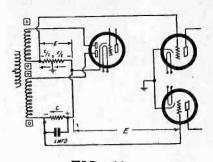
**FIG. 10** A true push-pull resistance-coupled circuit. The d-c voltage across the load resistor (upper diode) is divided, center of the resistor grounded, and when negative signal cycles are applied to the upper driven grid positive ones, with bias suitably bucked, are applied to the lower driven grid.
