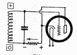
FIG. 1 The 56 used as a diode will stand 40 volts rms input. Diagram shows anode positive to a-c (sign in square), while direction of d-c current flow and d-c polarities of load resistor are designated.
