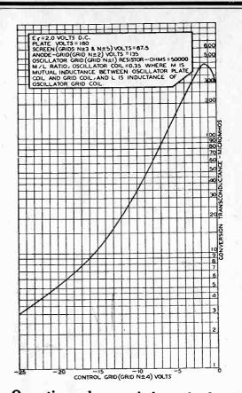
Operation characteristics of the 1A6. The control grid voltages are plotted against conversion transconductance in micromhos.
