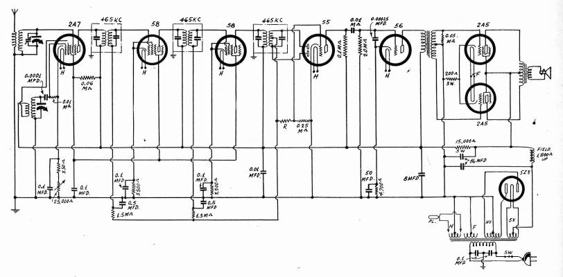
The eight-tube short-wave superheterodyne from which hum has been eliminated. The two condensers across the same potentials, low side of 15,000-ohm series resistor and ground, are 0.01 mfd. and 8 mfd. Of these the 8 mfd. reduces hum and the 0.01 mfd. bypasses radio frequencies. Otherwise for the higher radio frequencies the impedance of the intended bypassing might be entirely too large. Plug-in coils are used.
