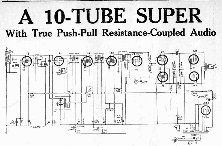
One of the anodes of the 55 is used as the separate rectifier to supply a bucking bias to the lower driven 58, the grid of which otherwise would run positive. The grid and plate of the 55 triode are not used because the cathode has to be "left in the air" to support the push-pull circuit.
