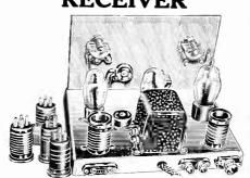
Made famous by its consistent reception. Will tune stations from every corner of the globe-from 15 to 200 meters with Powertone plug-in coils. Two sets of coils are used with the Dictator of the Air for clearer and more decisive reception. Uses 1-234 and 2-230 tubes.
