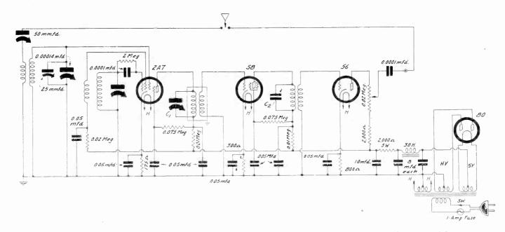
After some experimenting with converters it is well to build one like this, a real performer, with two stages of low radio-frequency amplification built in.
