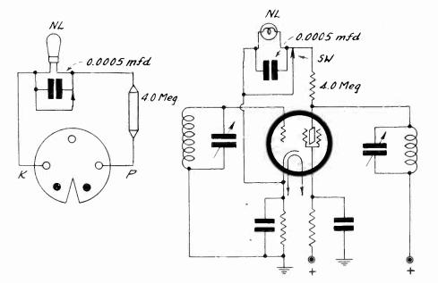
The same principle of a neon-tube audio oscillator, used for station-siren purposes, applied to a tube having a five-pin base. The control grids in
