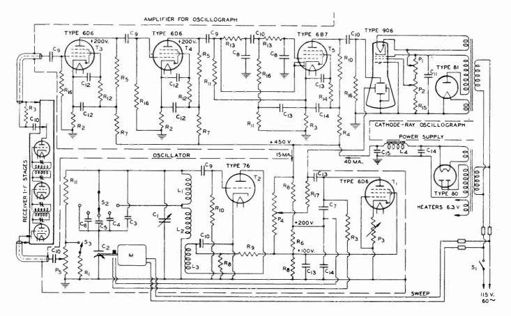
FIG. 1 Curve-tracing circuit using cathode-ray oscillograph tube.
