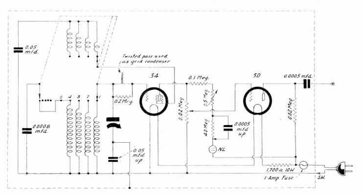
The 333-AB Signal Generator, covering the following on fundamentals: 83 to 99.9 kc; 140 to 500 kc; 540 to 1,600 kc; 1,400 to 5,000 kc; 5,400 to 16,000 kc. This device can be used by an infallible harmonic system for measurements up to ultra frequencies. There is an amplifier stage to provide plenty of kick.
