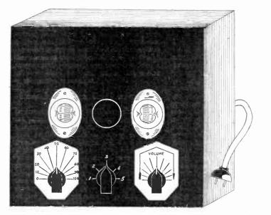
Front view of the 333-AB signal generator. The combination percentage modulation control and modulation on-off switch, applicable only to d-c use, is at left. The coil switch is at center. At right is the combination attenuator and a-c switch.
