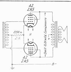
For triode connection screen and plate are tied together and the biasing resistor is raised to 850 ohms.
