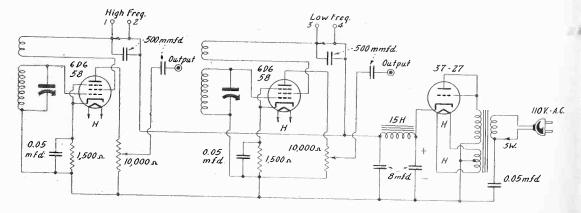
Put earphones between jacks 1 and 2 to listen to short waves or measure the frequencies of short waves when the broadcast oscillator at right is going. Put earphones at 3 and 4 to hear broadcasts, or to measure frequencies of still lower frequency oscillators.
