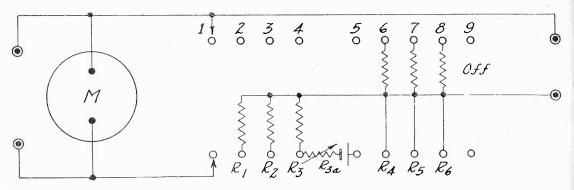
Direct access to the meter is at posts at left, for 0-1 milliampere, or for low resistance measurement when the switch is at position 5 and the right hand posts shorted for full scale deflection.
