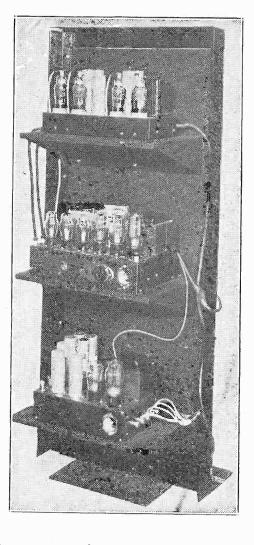
Many persons, after getting hookups to work swell, like to set up their rigs in suitable containers. The rack and panel method of construction is growing in its popularity because of its professional appearance as well as all-around suitability, except for parlor, bedroom and bath. A microphone pre-amplifier, a power amplifier and a speaker field exciter are shown (top to bottom).
