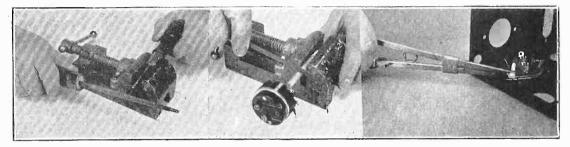
Sides of screw driver are filed so as to be at right angles with the flat tip, and "business edge" filed blunter, to give driver more strength. Next, small saw blade held only in hand will cut shaft of latest volume controls. Ant eater pliers grip things even when you remove hand, but not if you remove the spring.
