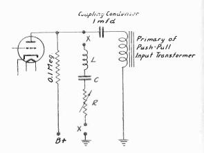
L, C and R are connected between X and X for compensating filter.
