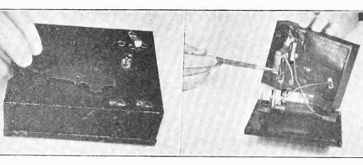
Upper left, completed apparatus in small metal box, with fingers properly placed on key knob for sending a practice signal. The little switch at rear of panel is used to change over circuit from buzzer to small flash lamp, thus giving visual signal, and no buzz. Pencil (right) points to "works" inside can and flashlight cells for supplying necessary electricity.
