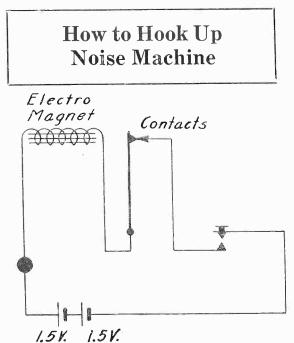
Circuit diagram of the buzzer and standard flashlight dry cells. Two cells used to supply the necessary energy. Depressing the key closes the circuit electrically, causing the electro magnet to become energized, which in turn pulls over the armature which breaks contact, thus opening the circuit again and armature returns to normal position, closing contacts. The cycle is repeated rapidly, thus resulting in the familiar buzzing sound.
