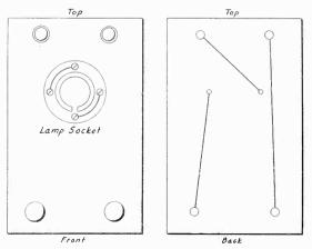
Diagram and top view. Condenser test post shorted, lamp is output meter.
