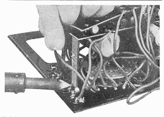
The final joint is being soldered at a binding post. The s
