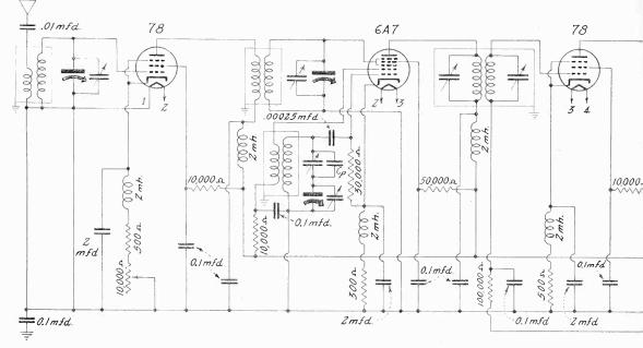
IR dielectric condensers are as important A as anything else in making a superhetero-dyne outperforming. I live in a district where the line is 110 volts direct current. Despite this limitation I built a receiver, the one shown in the diagram, that brings in all the channels at night. At present there are 102 channels, including five in the high-fidelity band, 1,500 to 1,600 kc, and a Canadian station added at the other end, 530 kc.
