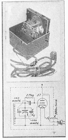
The box and the simple signal generator it contains. This generator works on a.c. or d.c. but has no modulation on d.c.
