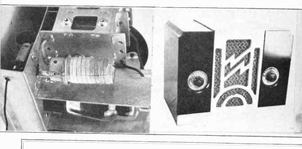
I N both the antenna and the interstage coil a high impedance primary is used in this five tube tuned radio frequency design. The results are excellent. In fact, the receiver works well enough to avoid trouble from WOR (now 50,000 watts) even in New York City, if a short antenna is used. Besides, the receiver does not oscillate even when a short antenna is used, which is an oddity, for it seems that most t.r.f sets suffer from this nuisance, which must be associated with poor design.
