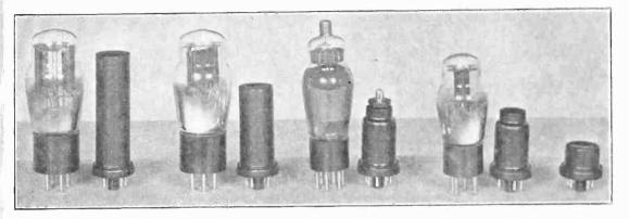
Contrast between the new metal radio tubes and glass-enclosed tubes of corresponding ratings. Left to right: rectifiers, power tubes, radio frequency tubes, small triodes, and, alone, the new duodiode, available only as a metal tube.
