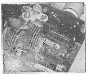
Tuning condenser, grid condenser, series condenser.
