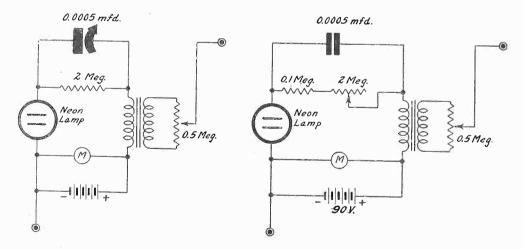
Variable frequency neon audio oscillators, with attenuation. The resistor is fixed, the condenser variable, at left, while at right the condenser is fixed and the resistor is variable. The meter should be left in circuit during operation of the oscillator, as any calibration would be upset by a small change in the applied voltage. One side of the output transformer may be grounded.
