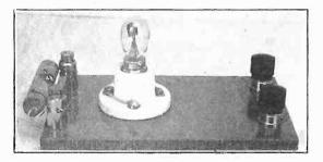
Condenser at left is being tested. A.C. posts at top. Neon lamp lights brighten on short.
