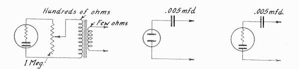
Lamp with built-in resistor has potentiometer across it, resistance rheostat further to limit current, so the lamp may be operated at normal current despite source voltage. A 0.005 mfd. condenser may supplant limiting resistor (center) or be used additional to such resistor.
