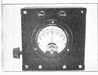
o that the shunts will be correct. The manuacturer will give the approximate resistance of the meter. However, one may measure this himself without danger to the meter.
