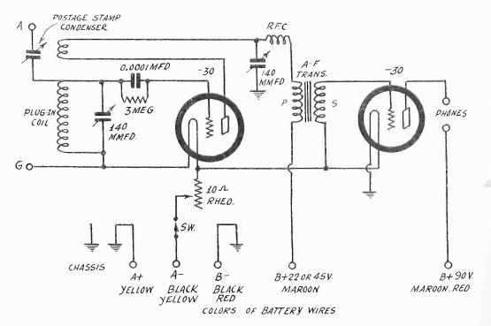
The tapering parallel lines used as ground symbol also are used as chassis symbol under conditions where chassis may or may not be grounded. To avoid any confusion the meaning of the symbol as used in a particular diagram is given, thus symbol above means chassis. That chassis in above example is not grounded is evidenced by negative filment going to G (ground).
