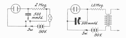
Intensity control is exercised at left by flipping the switch. The frequency remains practically unchanged. At right a variable condenser is used, for wide frequency change. The tubes must be of the type without limiting resistor built in.
