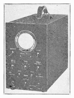
Type of instrument used for flat top alignment of intermediate channels. The more usual type of alignment also may be accomplished with the cathode ray oscilloscope shown. A signal generator is always necessary.
