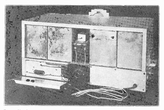
Swell tuner like this requires very close alignment, especially as a.v.c. is present. Weak output from generator must be used to do job well.
