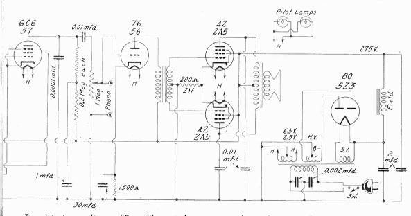
The detector, audio amplifier with pentode output, and rectifier, are shown above.
