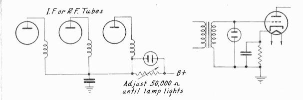
The resistor is adjusted until lamp is comfortably bright as tuning meter. Level indicator at right.
