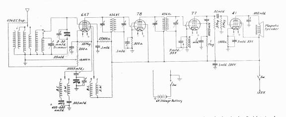
The battery version, in four tubes, of the midget superheterodyne with which Jack Goldstein has been amazing the wiseacres of Cortlandt Street. The demonstrations given in Radio World's laboratories certainly proved Goldstein's circuits outstanding.
