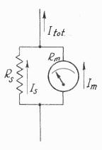
by  $R_m$ . The current through the meter is  $I_m$ . If the meter resistance, the meter sensitivity, and the current through the meter are known, the value of the unknown shunt across the meter may be computed. It is equal to the product of the meter resistance and the meter current, divided by the difference between full scale meter deflection and the current actually flowing through the meter. See article, page 48.
