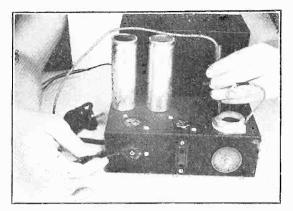
Electrolytics in cylindrical cans look like smokestacks, but that's not the point. Test leads applied to chassis check against shorts before turning on fatal juice.
