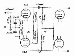
A phase inverter circuit using two tubes. P is used for balancing the inputs to the push-pull amplifier. The larger C is, the better the balance on low notes.
