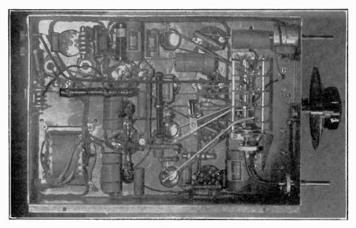
The fact that many parts have to be accommodated underneath, and therefore one is pressed for room, is confirmed by a glimpse of the under side of the chassis of the de luxe superheterodyne tuner. The flexible shaft is shown at lower right, enabling actuation of the switch from the usual front panel position, although the switch runs parallel to the front, instead of in the more usual right angle direction.
