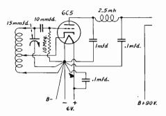
Circuit used for the five meter oscillator built in the black metal cabinet. The object is to study the presence of oscillation, make the amplitude about the same for the tuning range, by noting plate current meter needle, and later on select a suitable output coupling method. The choke coil, if provided with inductive or capacitative coupling, offers one solution, since there is a pronounced field.
