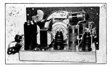
Switch type coils may be used in a small tuned radio frequency receiver of the regenerative type. The trick is so to place the coils that there will be no resultant dead spots. The trick was accomplished by one constructor in this manner.
