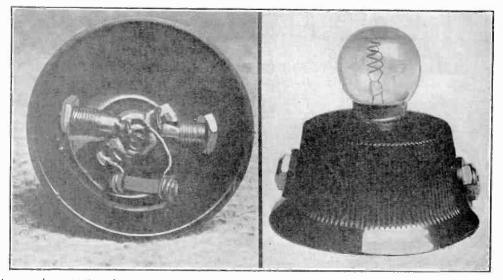
A neon lamp testing device was made in a panel knob shown slightly larger than actual size. A lamp without limiting resistor in it was used, the resistor being provided separately, .1 meg.
