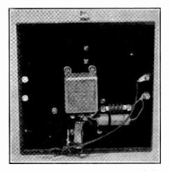
Parts wired underneath the platform of the five meter oscillator, using National Company parts.
