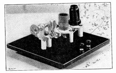
The metal tube is the 6C5, the small triode, which performed well as an oscillator on waves to ono meter, using the form of the series Hartley circuit, which, however, behaved as a Colpitts oscillator when the waves generated were low enough, say, below a couple of meters. The use of high grade sockets is of paramount importance to reduce leakage and other losses.
