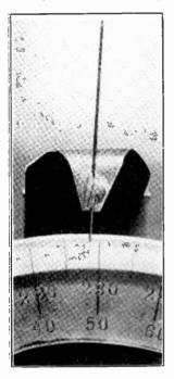
How a needle is used as a pointer. The indicator should be just a bit higher than the top of the calibration bars. The needle or other indicator should be as close to the scale as pos-sible, without without actually graz-ing, to avoid parallax.
