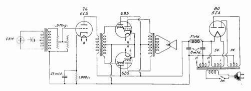
A small amplifier, using a 76 or 6C6 driver ahead of a push-pull 6B5 output, for double button microphone input.
