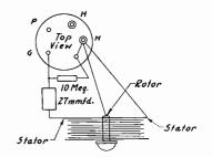
The completing condenser of .05 mfd. improved the oscillation, as did bypassing the resistor in the heater circuit, which resistor was built into the line cord. Application of 120 volts d.c., replacing a.c., enabled going down to 1 meter. At right is a top view, socket above the tuning condenser, showing the V inductance used around 1 meter.
