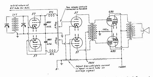
A transformer is included in this version of the LaFrance circuit. The results in the LaFrance circuit are somewhat dependent on the percentage modulation of the broadcasting stations, but the bias adjustment noted on the diagram takes care of this satisfactorily, provided the 37's are not worked near their full input voltage capability.
