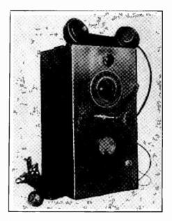
The French type earphones are plugged into a front panel jack when the dual switch is at "Receive" position.
