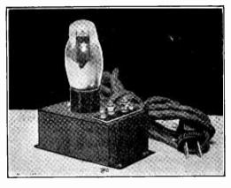
When an extra dynamic speaker is to be connected to a receiver the problem of supplying the field current must be solved. The new Radio Design Company field supply meets the situation admirably. It supplies up to 100 milliamperes at 100 volts. It can be used with most dynamic speakers having a field resistance of 1,000 ohms or over.
