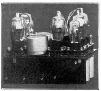
The i.f. transformers shown are of an old style and were replaced with new style transformers, whereupon results were strikingly better. Rear view of the chassis is shown. A glimpse of two r.f. coil shields is visible at lower right.
