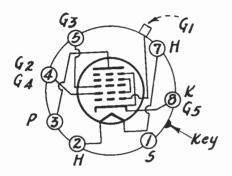
The internal arrangement of the elements of the 6L7 and the connections to the pins on the base.
