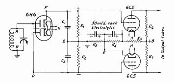
ences in capacities in the tubes, but this disappears when Cl and C2 are equal in fact. The two condensers placed in these two positions are then not necessarily exactly equal, but the capacity to ground in each leg should be equal.
