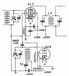
This mixer circuit is similar to that in the preceding figure but the oscillator voltage is obtained by connecting Grid No. 3 to the grid of the oscillator. This also provides the needed bias,
