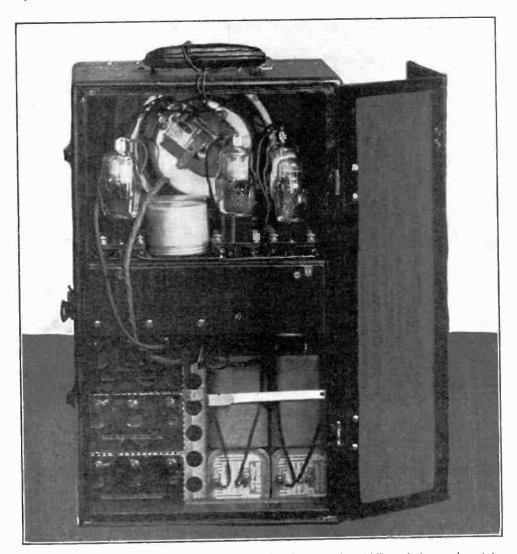
Rear view. The power supply is at the bottom, the chassis in the middle and the speaker at top.
