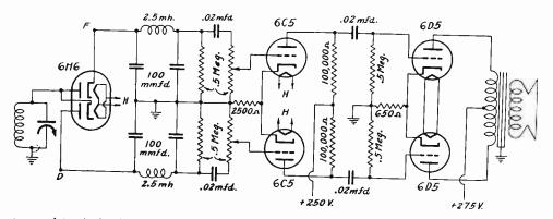
A complete diode detector and audio amplifier in which resistance-capacity coupling is used between the detector and the push-pull circuit. This is not strictly nonreactive, but can be made symmetricai.
