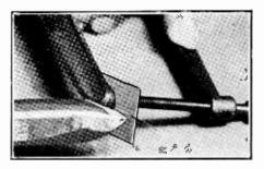
A needle may be used as pointer. The bracket is held in a C clamp and the needle is soldered to the bracket.
