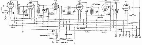
The circuit of the portable superheterodyne.
