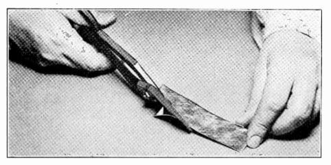
The tin pointer shown in the first illustration, front view of rotary protractor, is made by using tinsmith shears, cutting away from the intended point. The index should be very sharp and several cutting attempts may be necessary to accomplish this.
