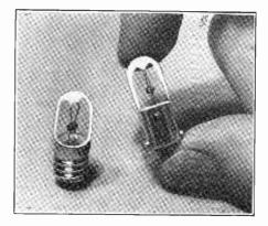
Two types of panel bulbs are shown, at left the screw type, which may have a tendency to work its way partly loose from the socket due to local vibration and create static-like interference by make and break contact, and at right the new bayonet type, which stays put, and gets rid of the interference. The studs at diametrically opposite positions on the bayonet base catch tightly into two keyways of a socket.
