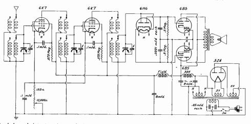
The balanced detector idea applied to a nonreactive circuit, using 6B5's in push pull output. The 6H6 detector arrangement is the one devised by Orval LaFrance, who comments, however, that oppositely polarized biasing batteries might well be included in the grid leads to the 6B5 to overcome the rectified voltage present due to the carrier when unmodulated, or due to position of a prior volume control at or near minimum value.
