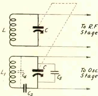
In order to establish tracking in a superheterodyne it is necessary to pad the oscillator circuit with a series and sometimes a shunt capacity.
