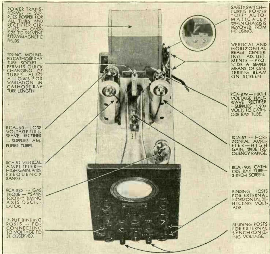
The "works" slid out of the cabinet, with parts identified. The safety switch is in inset.
