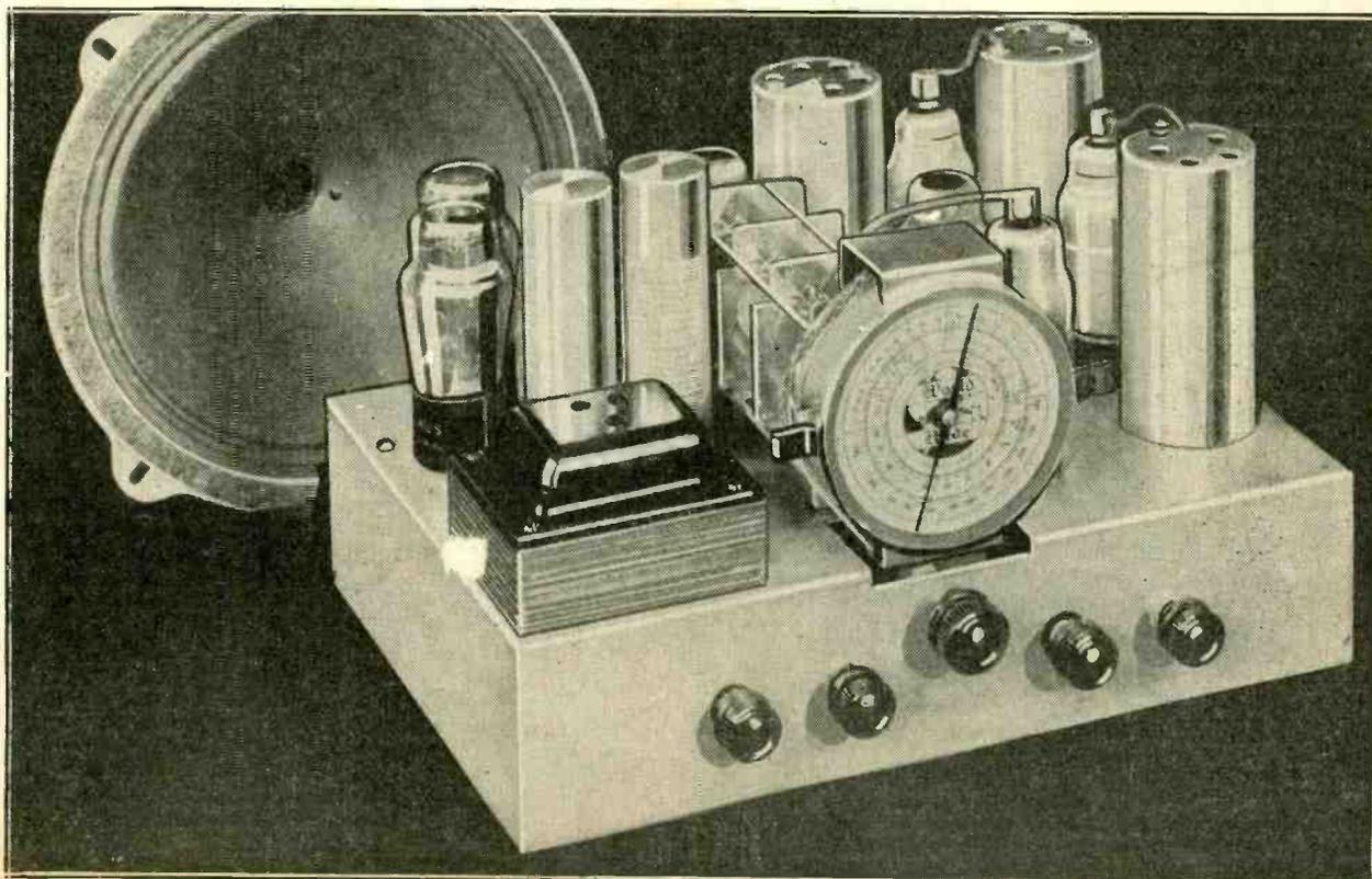
A finely developed coil system for switch type band changing, plus selection of finest parts, marks the new Postal All-Wave Receiver. See pages 12 and 13.
