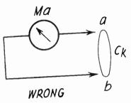
For current measurements the meter Ma serves to close the open. The points a and b therefore represent a discontinuity in the setup to be examined. It is wrong to put a current meter across a closed circuit, for that is a voltmeter connection, and the meter needs protection it lacks (series resistor).
