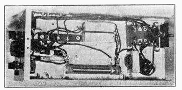
FIG. 7 Underneath view of the wiring of the ray-indicating
