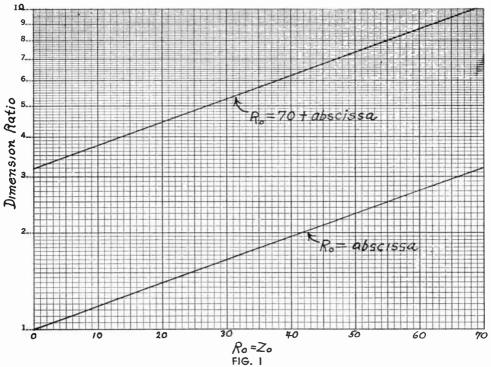
Graph for finding the characteristic resistance of transmission lines. Abscissas give resistance directly for concentric lines. Double abscissa readings for parallel wire lines. Dimension ratio for concentric R<sub>a</sub> ÷ R<sub>s</sub>, for parallel wire 2a ÷ d.
