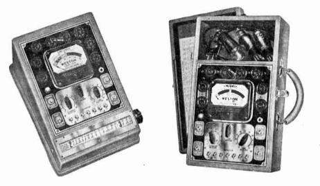
Model 773, at left, for combination with 772 Analyzer, or, at right, as individual portable unit.
