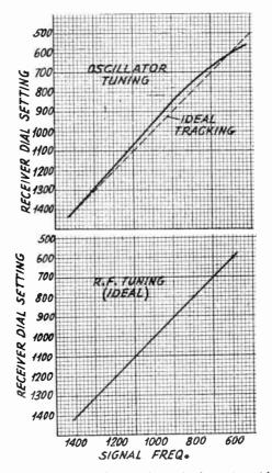
Graphs showing ideal tracking of r-f circuits, with respect to a frequency-calibrated receiver dial. Oscillator tracking is off 50 kc at 900 kc, due to use of too large inductance, with tiedown effected at 1,400 and 600 kc by adjustment of trimmer and padder. In practice it is usually feasible, by using a large enough sheet of paper, to put both curves on the same chart.
