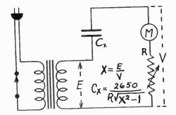
An ohmmeter method applied to measurement of capacity C<sub>x</sub>, using the power line a.c. (60 cycles). X is the voltage read with C<sub>x</sub> shorted, V the voltage read with C<sub>x</sub> inserted. C<sub>x</sub> is solved by the formula at lower right.
