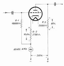
FIG. 1 Type 56 tube as an amplifier.
