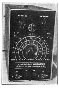
FIG. I The instrument panel as built by the author.
