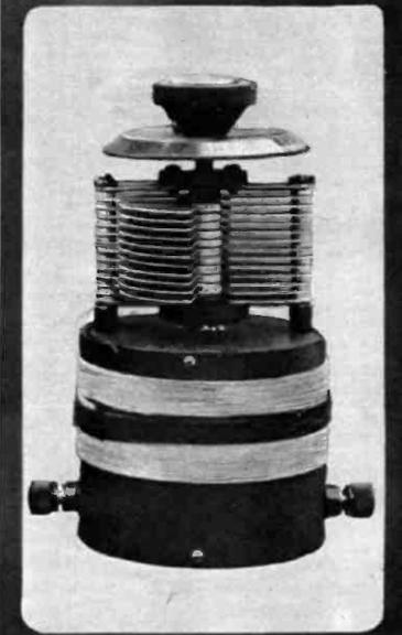
*Another form of the wave trap spoken of in this article. Here the variable condenser is mounted high above the coil so as to be kept away from the magnetic fields.*
