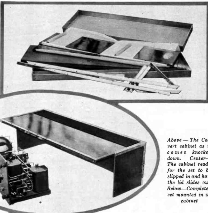
Above—The Calvert cabinet as it comes knocked down. Center—The cabinet ready for the set to be slipped in and how the lid slides out. Below—Completed set mounted in its cabinet
