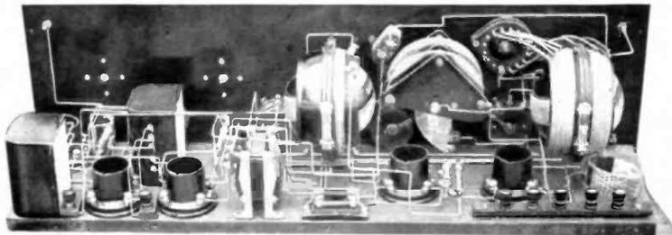
Looking at the Langbein & Kaufman set directly from the rear showing the placing of the apparatus on both baseboard and panel
