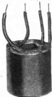
The winding that Kellogg developed, was found to be most efficient for audio frequency transformers. Its problems involved the finding of the proper thickness of paper, the proper kind of insulated wire to provide the proper number of ampere turns, and impedance.
