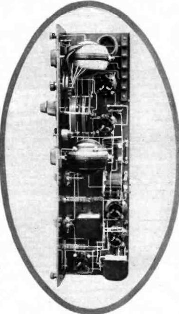
of straight audio frequency amplification and one stage of push-pull amplification.
