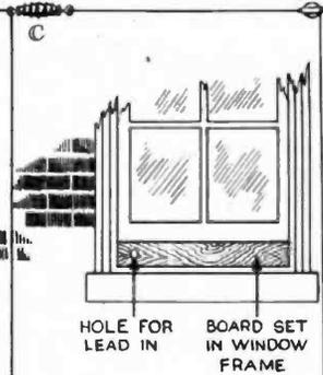
HOLE FOR LEAD IN BOARD SET IN WINDOW FRAME
