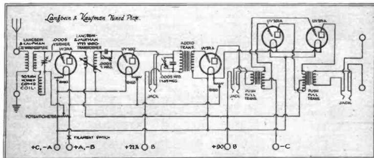
plate circuit of the radio frequency amplifying tube and really becomes a tuned circuit because it is so closely coupled to the variometer that the tuning of the variometer really tunes the plate circuit also.
