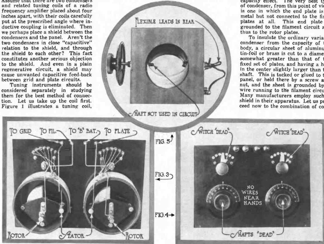
Rear view of the tuning circuits of a tuned plate receiver made for short wave lengths, where hand capacity is a serious objection. Note that all the "sensitive" points are at a distance from the panel
