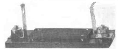
Mica Grid Condenser and Grid Leak Mountings
