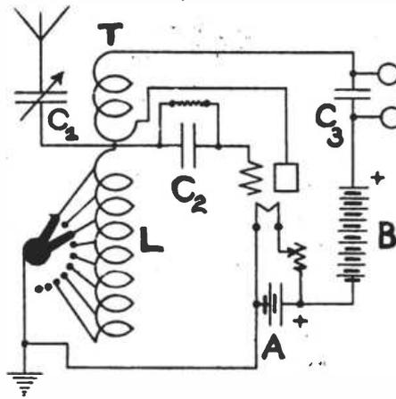
Fig. 1. Receiver Circuit
