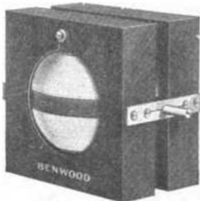
These variometers cover a wave length range of 150 to 650 meters when used in conjunction with the average variocoupler. The features are, minimum distributed capacity, minimum distance between stator and rotor, large size wire on both coils, positive contact bearings and properly designed mechanically as well as electrically.
