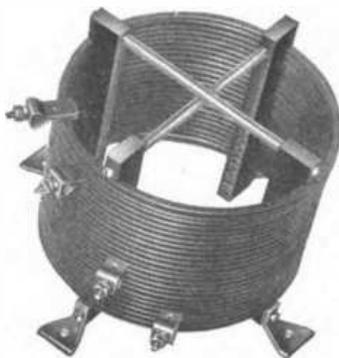
Standard size as shown consists of 25 turns of edgewise wound soft drawn copper ribbon 3/8 inch in width, 1/16 inch in thickness and the turns are SEVEN INCHES in diameter.
