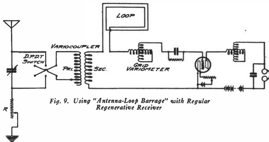
Fig. 9. Using "Antenna-Loop Barrage" with Regular Regenerative Receiver
