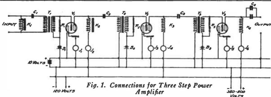
Fig. 1. Connections for Three Step Power Amplifier
