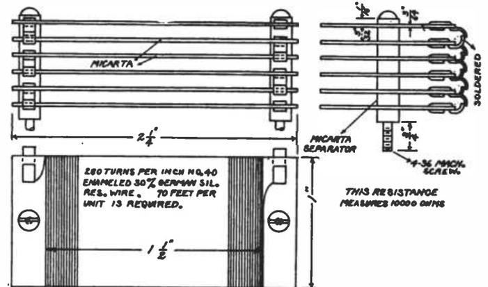
Fig. 27. Details of 10,000 Ohm Grid Leak
