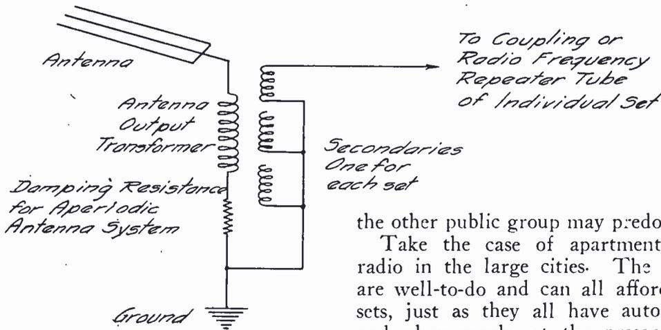
Plan 2. Common Antenna with Radio Frequency Distribution.
