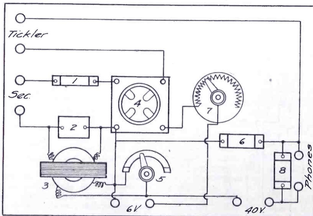
Fig. 3. Suggested Layout for Hookup on Fig. 2.
