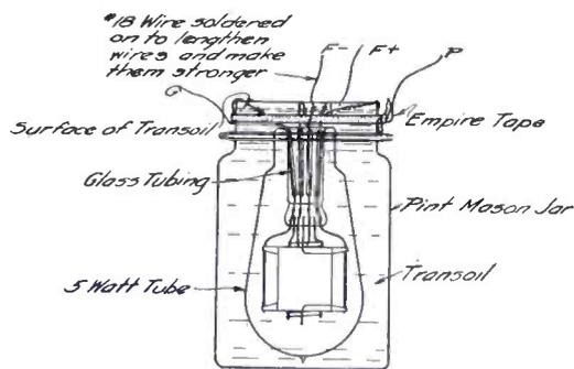
Fig. 1. Section showing 5-Watt Tube in Oil
