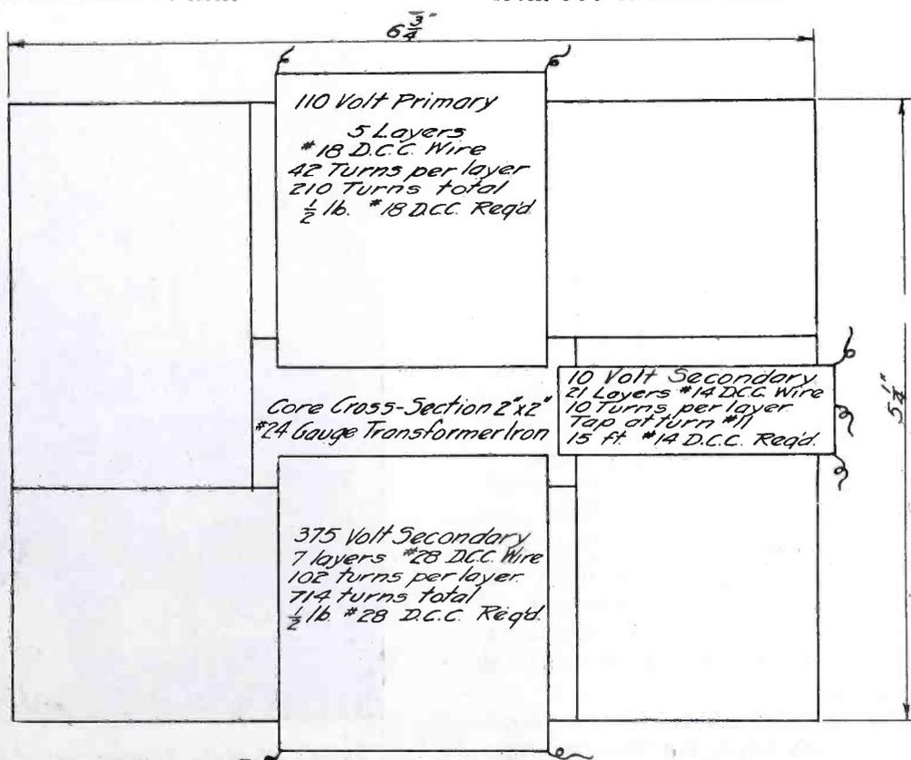
Fig. 2. Design for Power Transformer.
