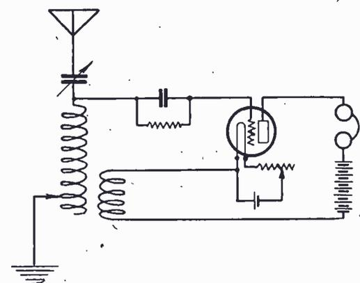
Fig. 1. Single Circuit Receiver Employing Tickler Regeneration. This circuit should show ground connection for the filament.
