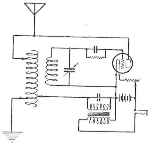
Fig. 1. Circuit Diagram for I. C. W. Transmitter
