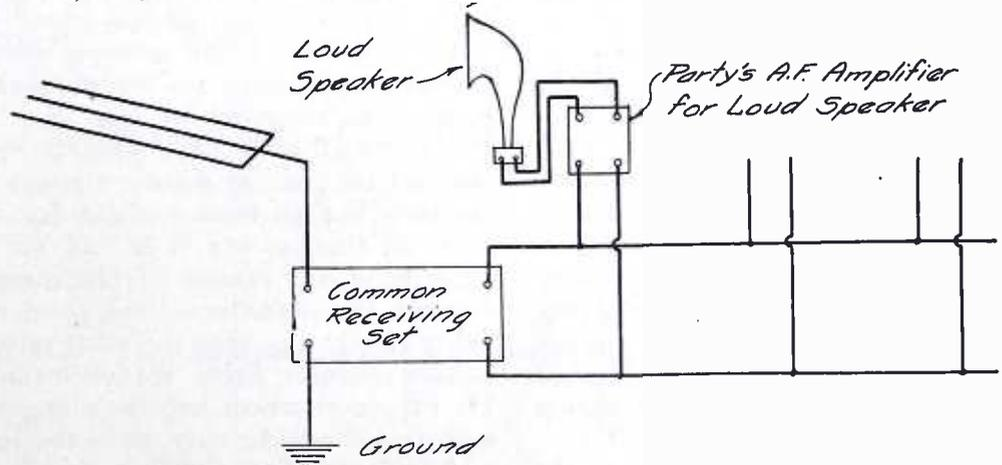
Plan 3. Common Antenna with Audio Frequency Distribution.
