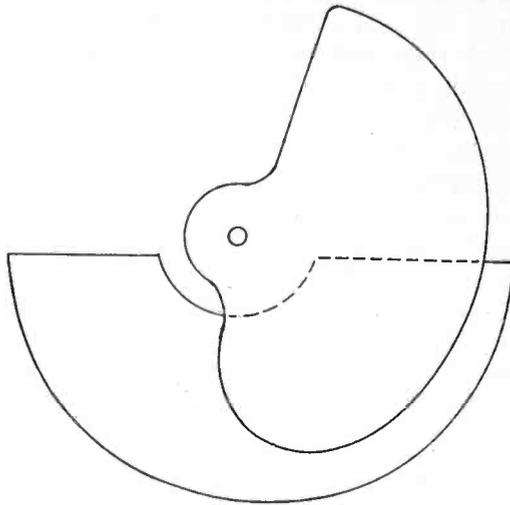
Fig. 6. Shape to Give Uniform Capacity
