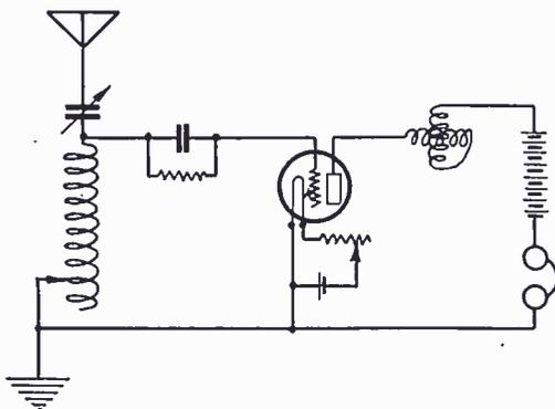
Fig. 1. Single Circuit Receiver Employing Tickler Regeneration.
