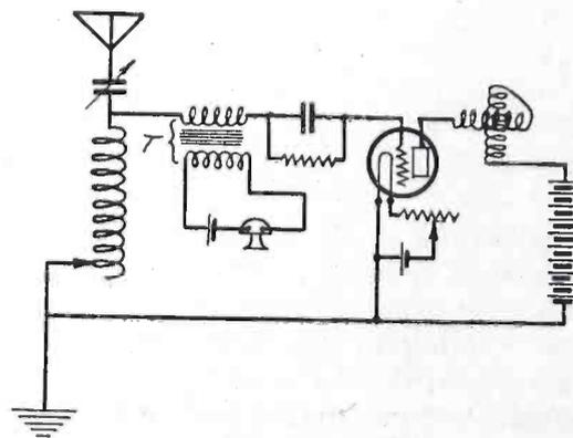
Fig. 9. Microphone in Grid Circuit through Transformer.
