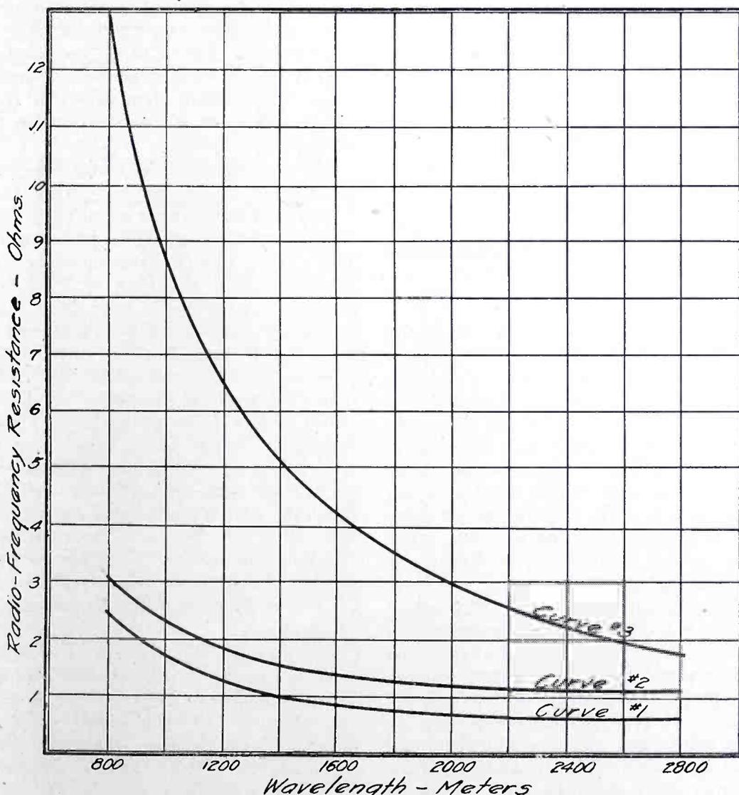
Fig. 1. Radio Frequency Resistance of Bank Wound Litz Coils.
