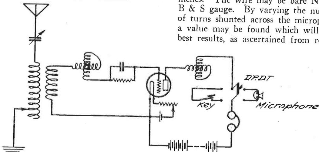
Fig. 6. Two Circuit Variometer-Coupled Set with Key and Microphone in Plate Lead.
