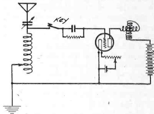
Fig. 8. Key in Grid Lead.
