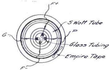
Fig. 2. Plan of Connections.
