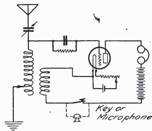
Fig. 4. Two Circuit Receiver Employing Plate Variometer Regeneration.
