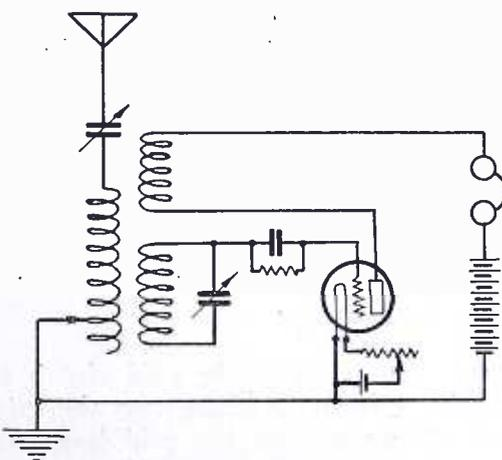
Fig. 2. Single Circuit Receiver Employing Plate Variometer Regeneration.
