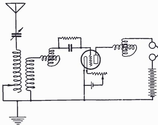
Fig. 3. Two Circuit Receiver Employing Plate Variometer Regeneration.
