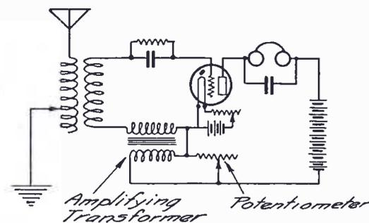
Fig. 1. Hookup for Audio Frequency Amplification.
