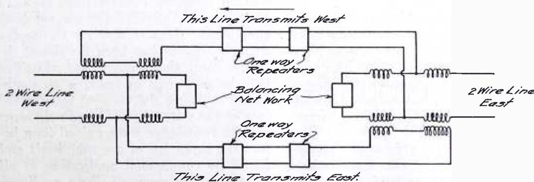
Fig. 3. Four-wire Line with One-way Repeaters.
