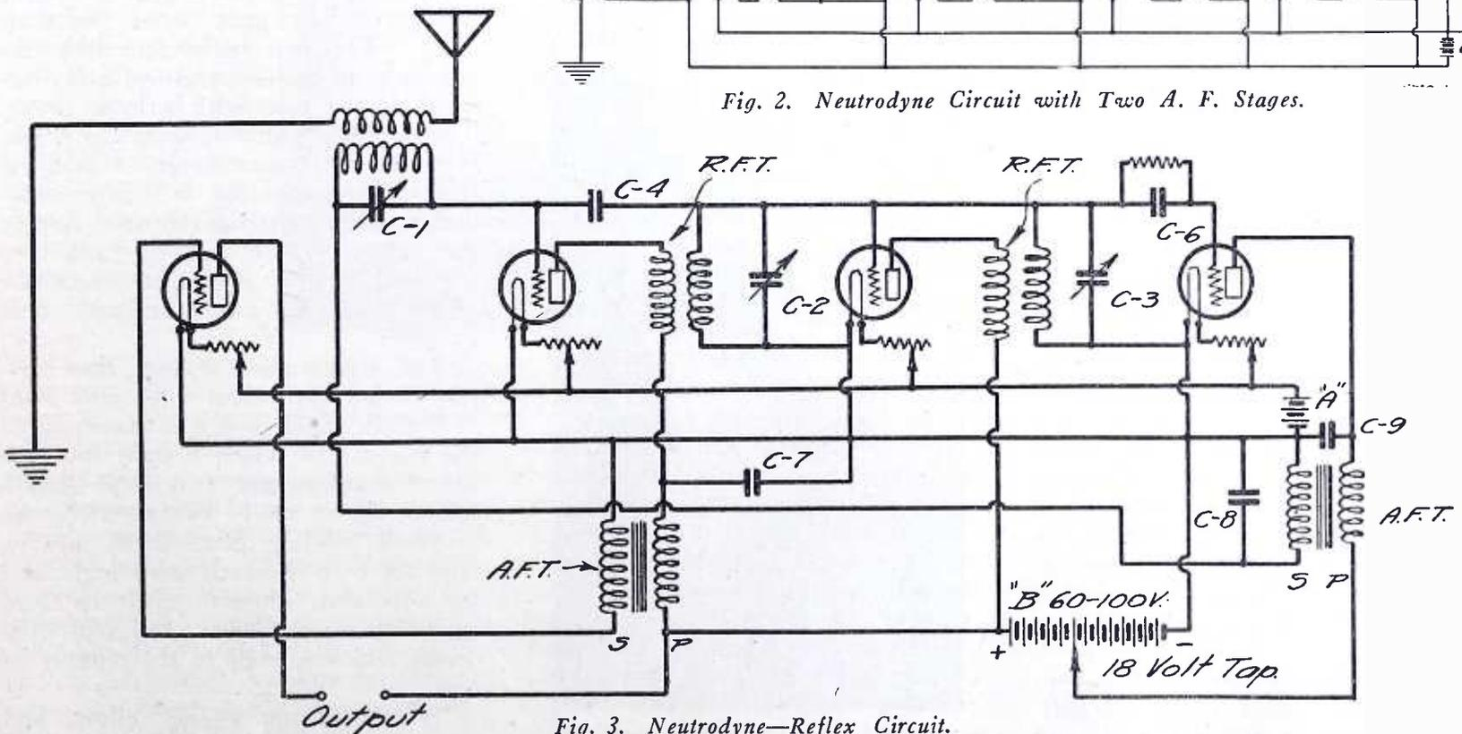
Fig. 3. Neutrodyne—Reflex Circuit.
