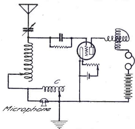
Fig. 7. Key or Microphone in Antenna Lead
