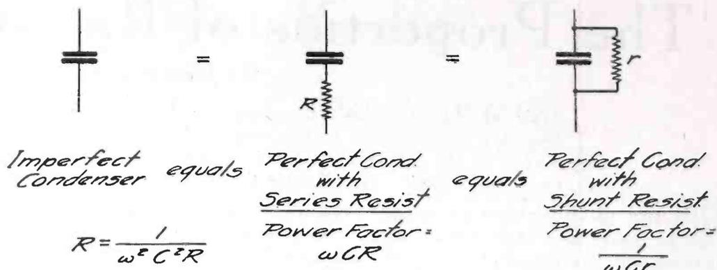
Fig. 1. Power Factors of Condensers
