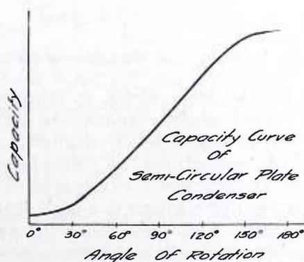
Fig. 3. Variation of Capacity with Rotation
