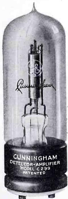
The filament current should be supplied from three standard No. 6 dry cells in series, with a suitable rheostat. From three to five tubes may be operated in parallel from a single set of three batteries in series. Six dry batteries connected in series parallel will prove more economical when more than three tubes are used.
