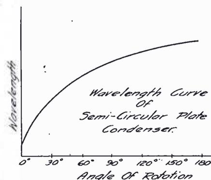
Fig. 4. Variation of Wavelength with Rotation
