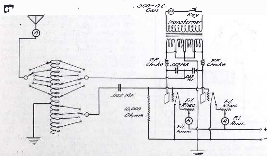
Fig. 1. Wiring Diagram of ½ K. W. Navy Spark Set Converted into 100 Watt Tube Set.
