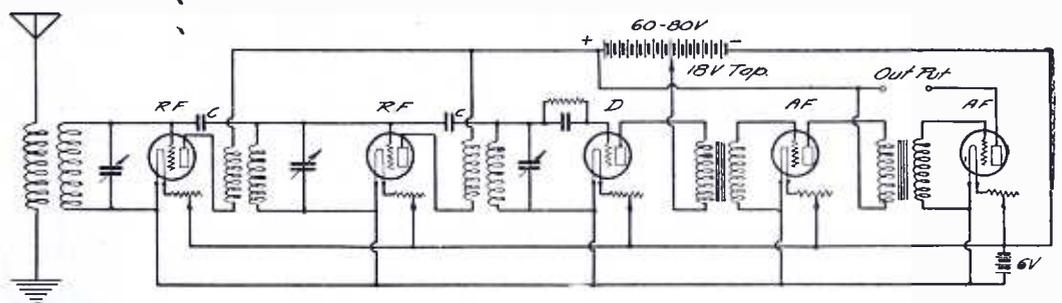
Fig. 2. Neutrodyne Circuit with Two A. F. Stages.
