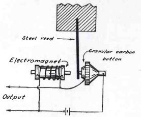
Fig. 2. Voice-Frequency Generator, 800 to 1000 Cycles per Second
