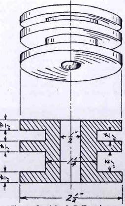
Fig. 4. Spool for I. F. Transformer
