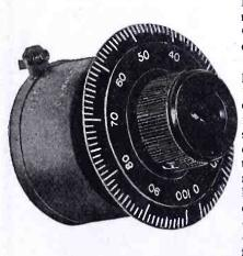
By a simple change in terminal connections the type D-19 Connecticut T r i p le Range condenser gives the capacity range equivalent to an 11plate, 23-plate or 43-plate variable condenser. Only one panel hole is needed for mounting, it is completely shielded against body capacity and its dial rotates through 346 degrees, thus making closer tuning possible. Behind the panel it occupies a space 2 in. in diameter by 1 5/16 in. deep. Its effective resistance to radiofrequency currents is low.
