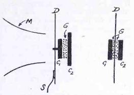
Fig. 1. Commercial Telephone Transmitter Fig. 2. High Quality Telephone Transmitter
