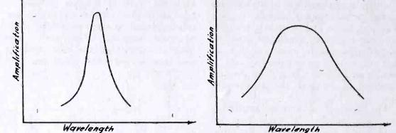
Fig. 5. Amplification Curves, (a) with Ordinary R. F. Transformers, (b) with Transformers Wound with Resistance Wire or Having Iron Cores
