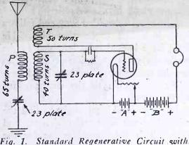
Standard Regenerative Circuit with Three Spiderweb Coils
