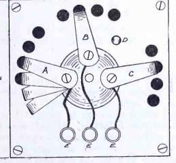
Fig. 2. Method of Fastening Switch Points A filament control for switch, B stage-to-stage switch, C detector plate voltage and amplifier plate voltage control, D stop, E binding posts.
