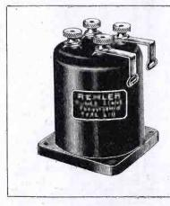
Remler Type 610 tuned stage transformer is designed to work between the last intermediate frequency stage and the detector tube of a superheterodyne receiver. With a .00025 mfd. condenser it gives maximum amplification at 45,000 cycles and fairly uniform amplification over a range of 3000 cycles on either side thereof. It is made with an air core and primary impedance to match that of a standard dry battery tube.
