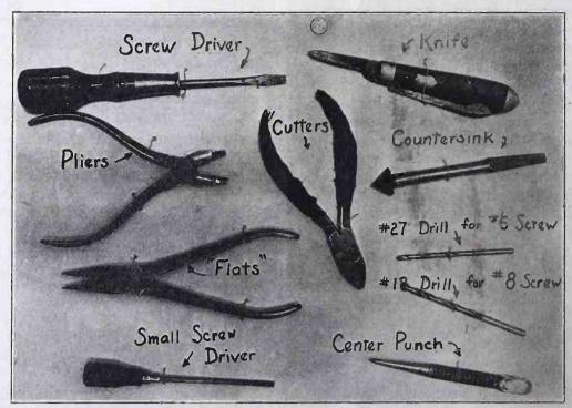
Fig. 4. Tools Needed for Panel Drilling
