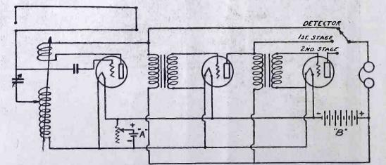
Circuit Diagram for Compact Single-Circuit Receiver Without Ground Connection
