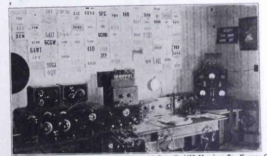
Radio Station 988, Owned and Operated by E. B. McDowell, 4419 Harrison St., Kansas City, Mo. 100 Watts Modified Hartley, 1500 Volts on Plate, 2 Amps Radiation, 100 Ft. Steel Tower Aerial with Cage Lead-in and 14-wire Radial Counterpoise.
