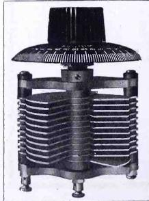
Losses have been reduced to a negligible quantity in the new Cruver condenser designed by G. M. Proudfoot. The stator plates are mounted on two instead of the usual three plates so as to give a loss of but .007 per cent at a capacity of .001 mfd. By means of two scales the coarse adjustment is made by turning the knob to the right on the large scale and the fine adjustment by turning to the left on the small scale. Body capacity effects are eliminated by grounding the rotor plates.
