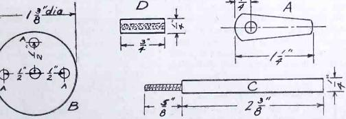
Fig. 3. Details of Combination Switch
