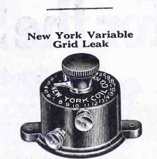
This instrument is small and compact. It gives an unbroken, gradual resistance variation of from 1/4 to 6 meg. ohms. A permanent resistance element is employed; a roller arranged to travel over same thus avoiding wear on the resistance element. It avoids the necessity of buying three or four various sized Fixed Grid Leaks, and is a quality product throughout.
