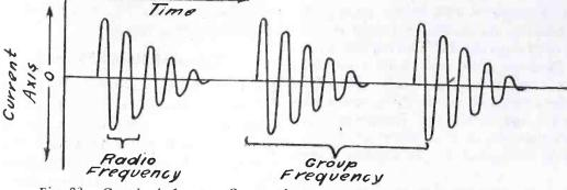
Fig. 23. Graph of Antenna Current from Damped Wave Transmitting Set
