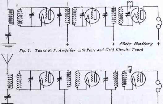
Fig. 2. Tuned R. F. Amplifier with Plate Circuit Tuned
