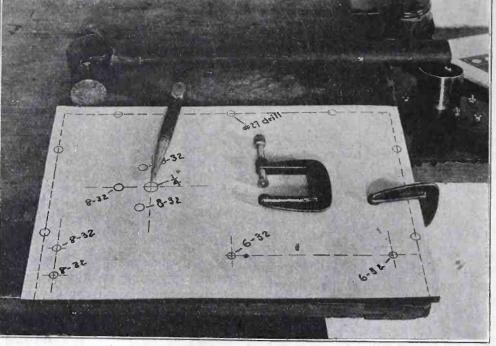
Fig. 2. Panel and Template Ready for Punching
