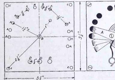
Fig. 1. Drilling Layout for Base
