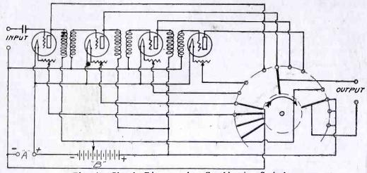
Fig. 4. Circuit Diagram for Combination Switch
