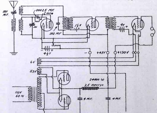
Fig. 5. Receiving Circuit with Plate Current Supply for 3 Tubes and Filament Supply from Transformer for 1 Tube
