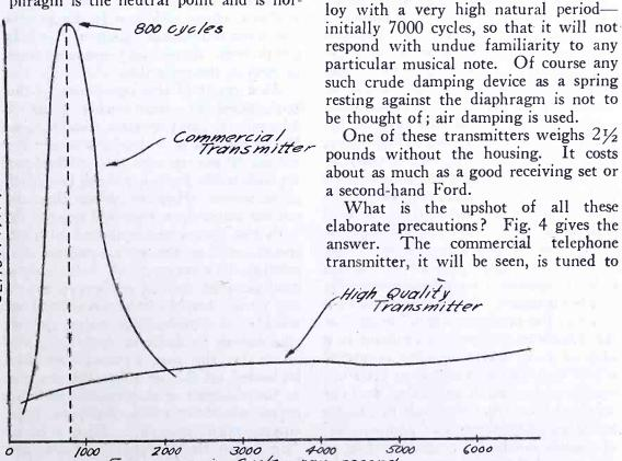
Frequency in Cycles per second Fig. 4. Frequency Characteristics of Commercial and High Quality Transmitters
