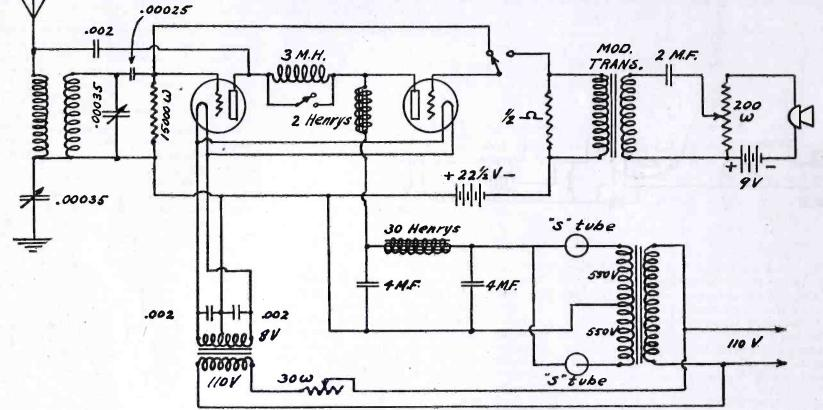
Fig. 1. 10-Watt C. W. Transmitter
