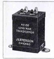
The new Jefferson long wave transformer is built with a laminated silicon steel core and impregnated coils assembled in a sealed metal case. It is designed to give maximum amplification at 6600 meters (45,454 cycles), and thus is particularly adapted for use as an intermediate frequency amplifier in a super-heterodyne receiver. Due to its construction, it is claimed to be sensitive and uniform in operation under all conditions.
