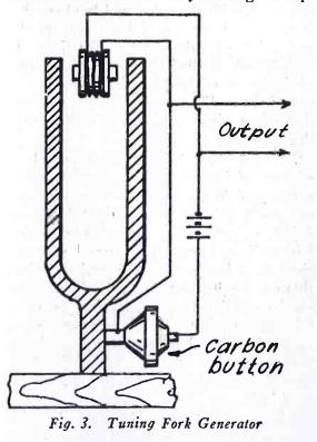
from each side of the electromagnet winding, pulsating current can be had of the pitch of the reed, and this may be made alternating by passing it through an audio-frequency transformer.
