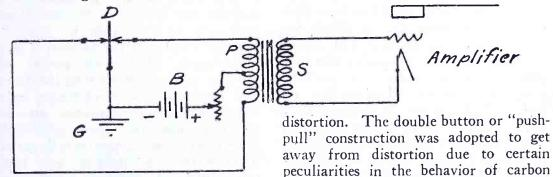
Fig. 3. Electrical Connections of Microphone
