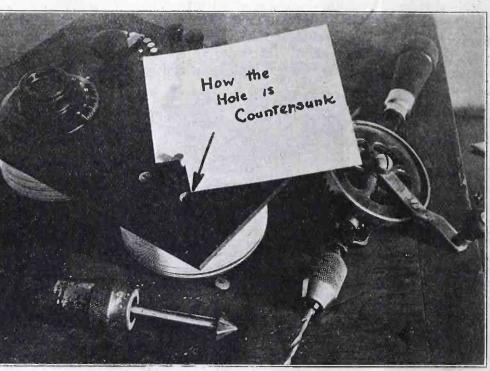
Fig. 3. Counter-Sinking Holes
