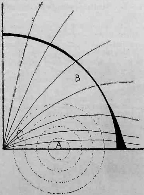
Fig. 6. Illustration of How Fading May Be Produced.
