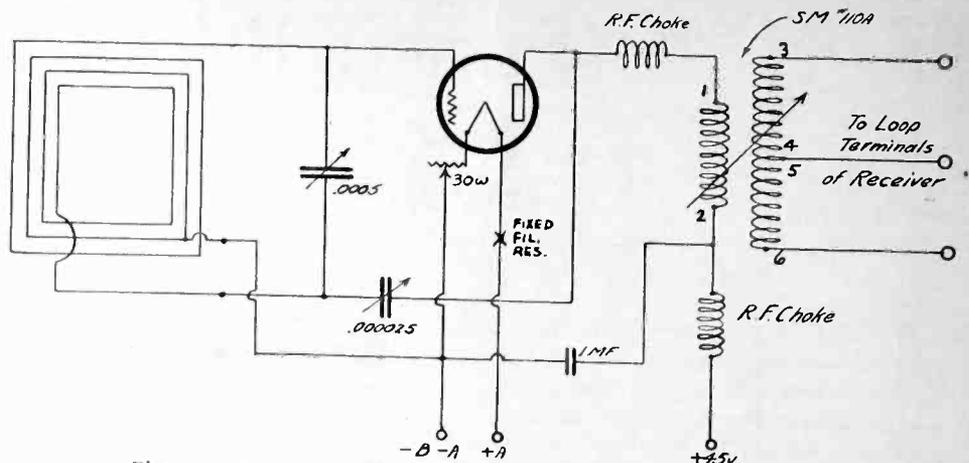
Fig. 2. Arrangement of Amplifier for Use With Loop Antenna.
