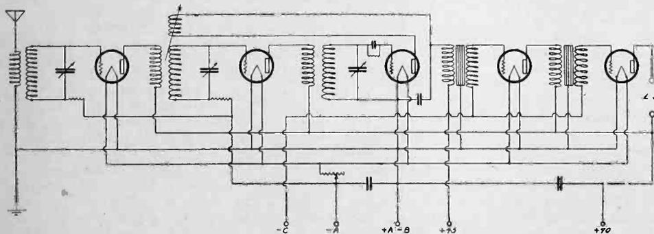
Fig. 1. Wiring Diagram of Crosley 5-38 Receiver.
