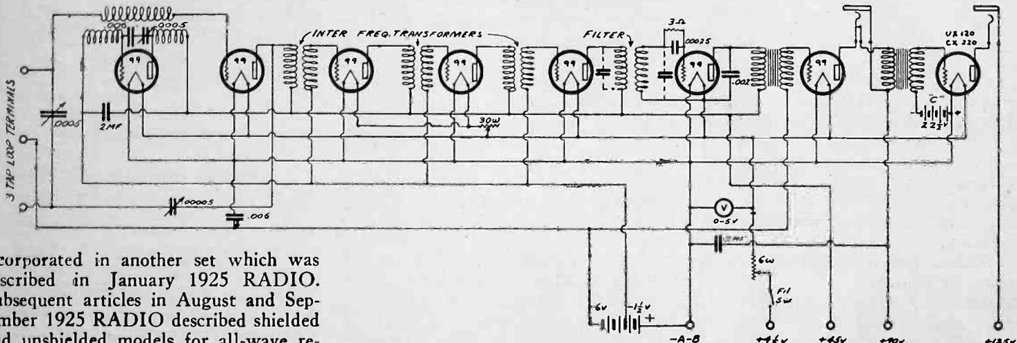
Fig. 1. Best Superheterodyne, using all dry cell tubes, as published in May 1924 RADIO.
