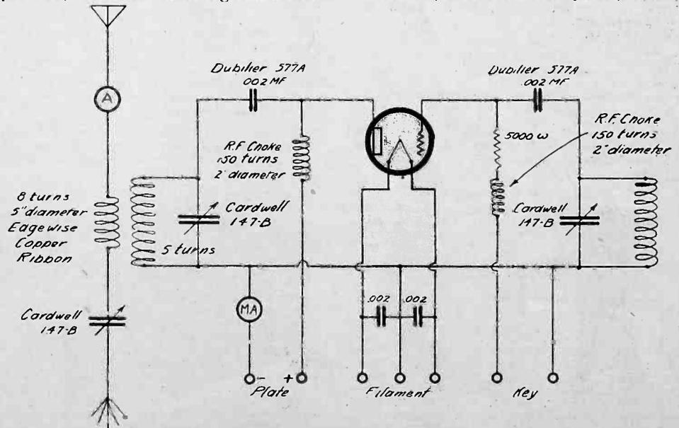
Circuit Diagram for Transmitter at 2QA.
