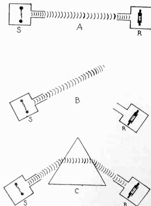
Fig. 1. Refraction of Radio Waves.
