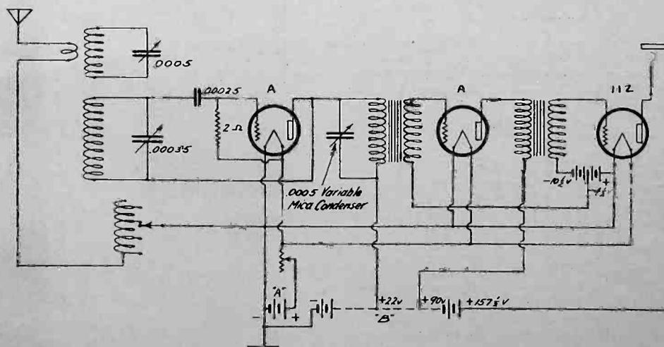
Fig. 2. Three Tube Cockaday Circuit.
