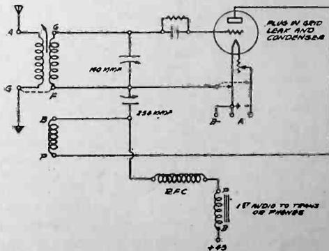
Fig. 3. Corrected Arrangement of Aero Coil Tuner.
