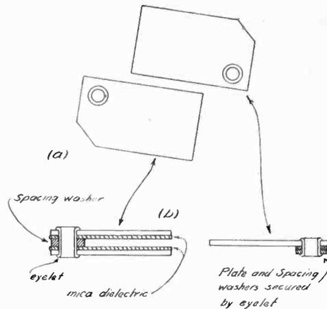
Fig. 4. Method of Adjusting Capacities.
