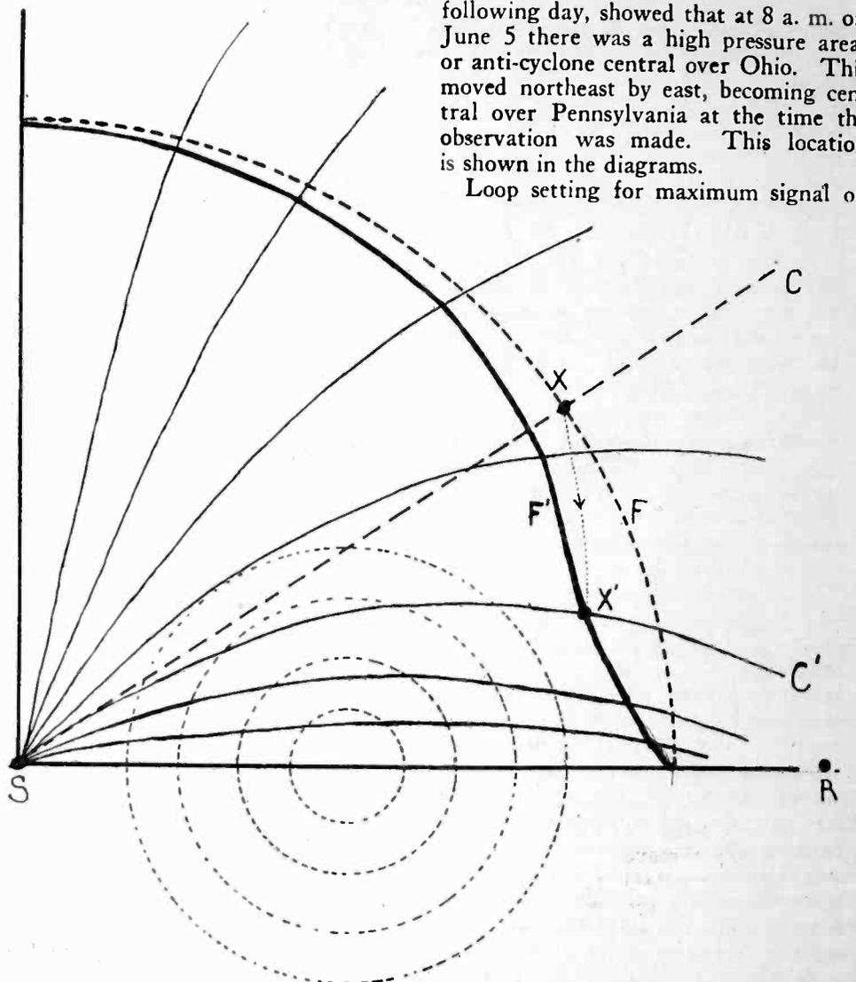
Fig. 5. Effect of Refracting Atmospheric Structure.
