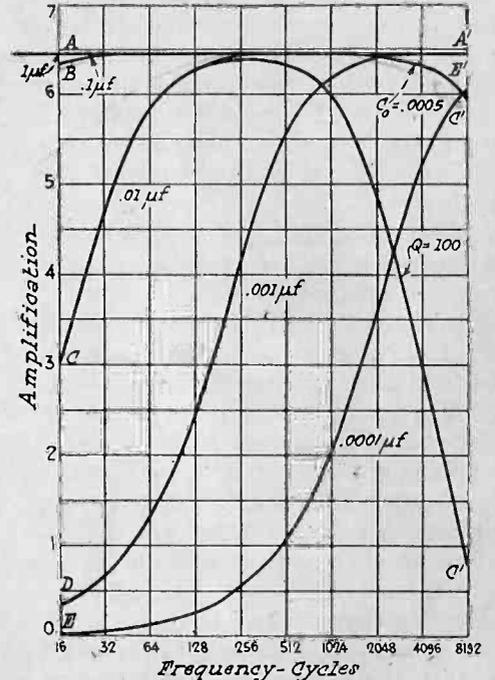
Fig. 3. Distorting Effect of Various Stopping Condensers.
