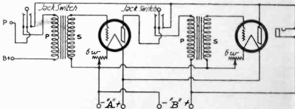
Fig. 3. A.F. Amplifier Circuit.
