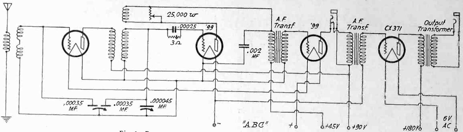
Fig. 3. Rearrangement of S-C Circuit for Batteryless Operation.
