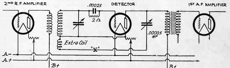
Fig. 3. Regeneration Control for Detector in Tuned R. F. Circuit.
