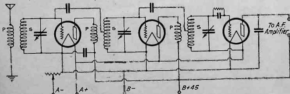
Fig. 2. Conventional Neutrodyne Circuit.
