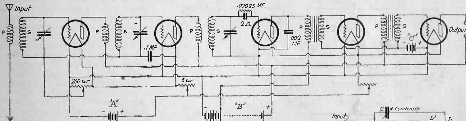
Fig. 1. Basic Tuned R.F. Circuit with Potentiometer Control.
