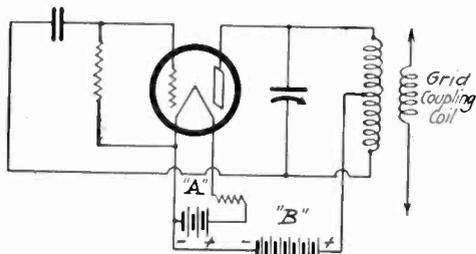
Fig. 4. Oscillator with Tuned Plate Circuit.
