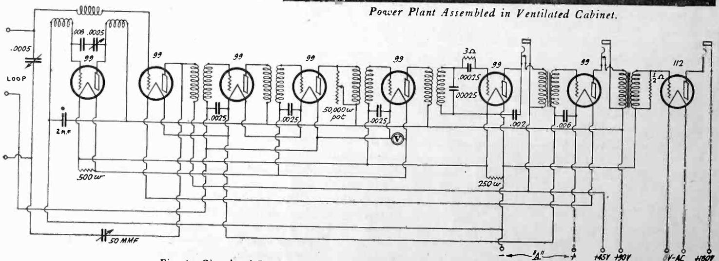
Fig. 4. Circuit of Best Superheterodyne, Wired for Use With Power Plant.
