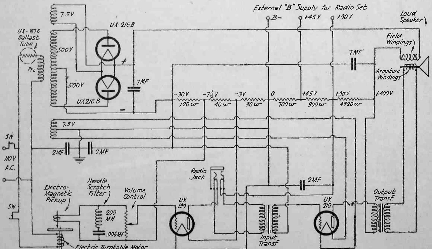
Fig. 1. Schematic Wiring Diagram of Panatrope.
