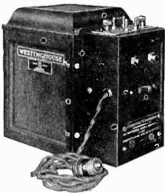
years without deterioration. The charging rate can be varied from  $\frac{1}{10}$  to  $\frac{1}{2}$  ampere, with two intermediate steps, by simply changing the position of a connecting link between the four contacts. The unit is made in four models, 4 volt 60 cycle, and 6 volt 65, 50 and 25 cycle.
