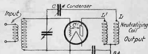
Fig. 3a. Hazeltine Method of Control.
