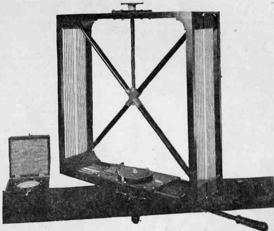
*Kolster Loop Developed as Direction Finder for Radio Supervisor's Truck.*
