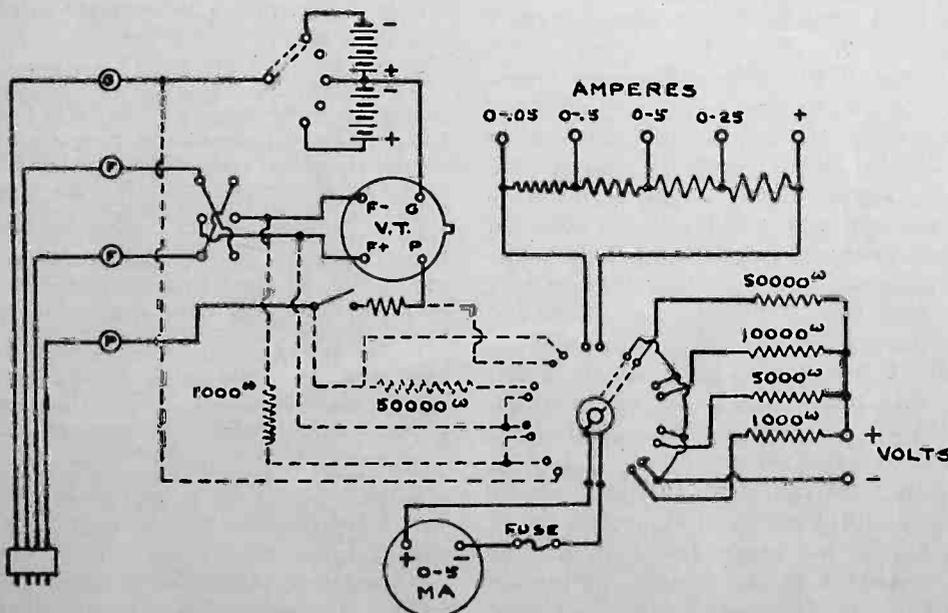
Fig. 2. Circuit Diagram of Testing Instrument.
