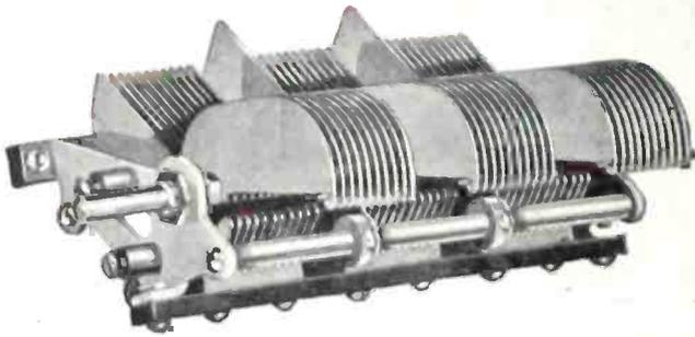
**T**HIS Continental special triple condenser was designed by Mr. E. M. Sargent for use in the Infra-Dyne Circuit.
