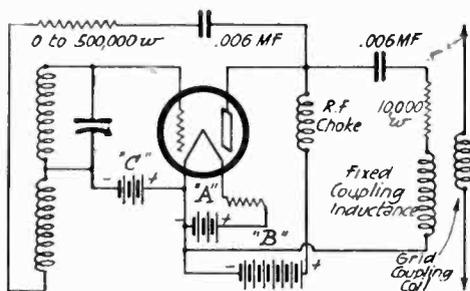
Fig. 5. Stabilized Oscillator, Using Tuned Grid Circuit.
