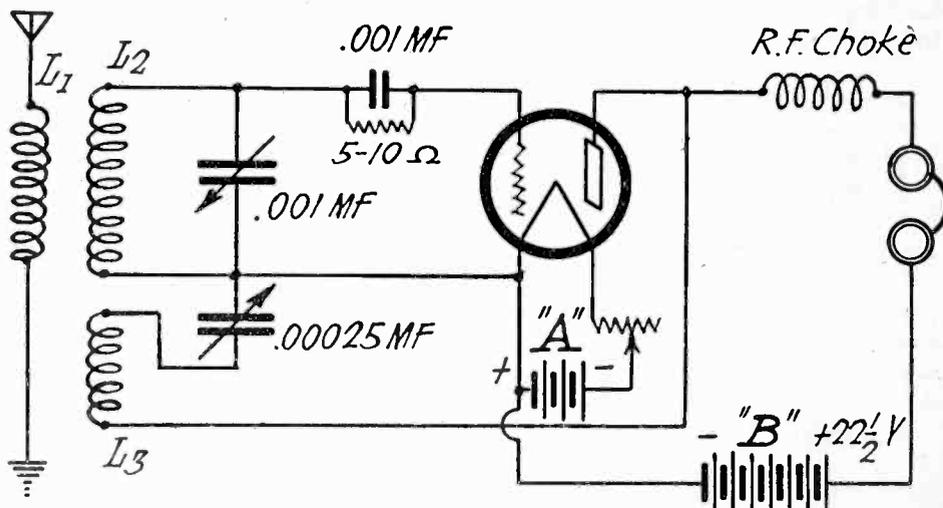
Fig. 1. Circuit Diagram for Short-Wave Receiver.
