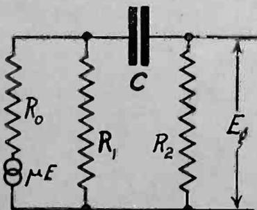
Fig. 1. Circuit Equivalent to Resistance Coupled Amplifier with Stopping Condenser.
