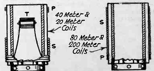
Fig. 2. Coil Winding Details.
