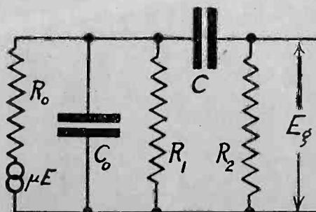
Fig. 2. Circuit Equivalent to Resistance Coupled Amplifier with By-Pass and Stopping Condensers.
