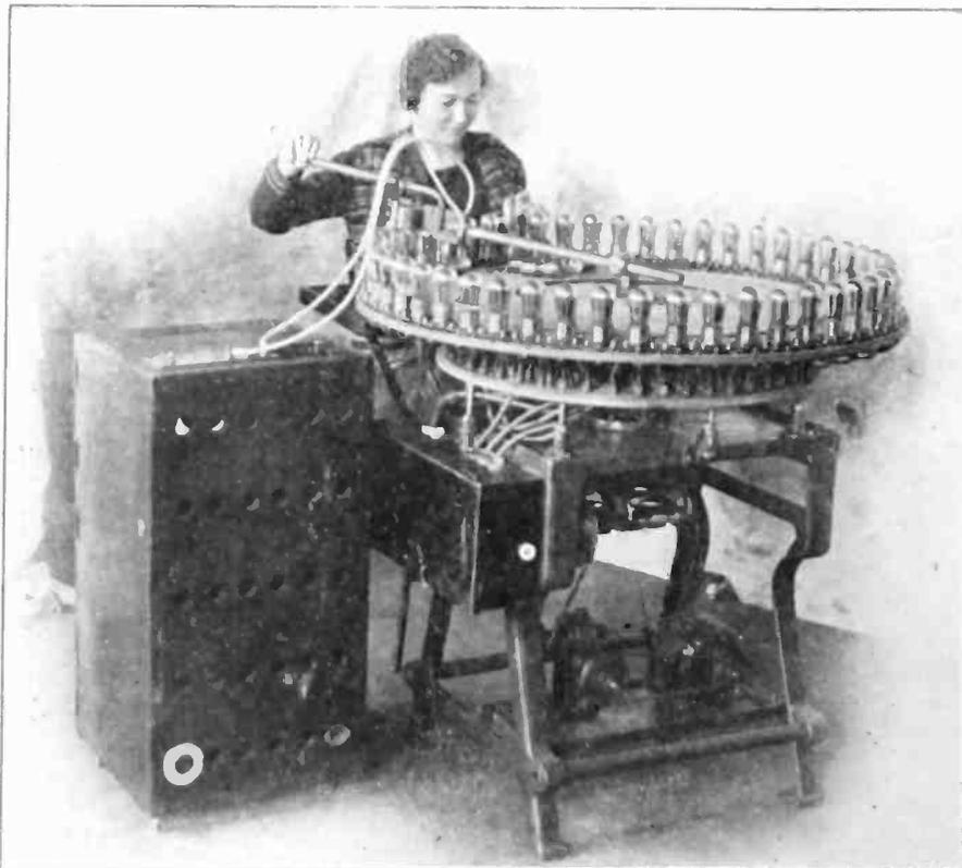
*A Laboratory-Created Tube Ager and Bombarder Which Has Helped to Reduce the Manufacturing Cost of a 201A Tube to 28 Cents.*
