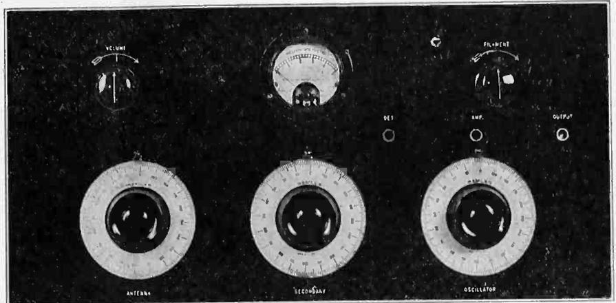
Panel for Superheterodyne With One Stage Tuned R.F. Amplifier.
