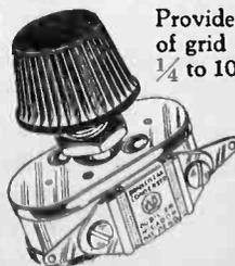
Provides a noiseless range of grid leak resistance from 1/4 to 10 megohms. Assures most effective grid leak resistance value for all tubes. Small grid condenser (0.00025) is separate. Metal parts nickel plated. One hole mounting.
