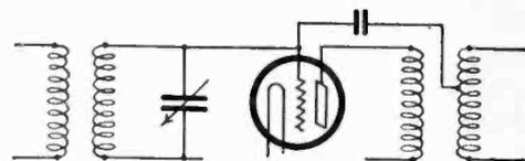
Fig. 8. Hazeltine Method of Neutralization.
