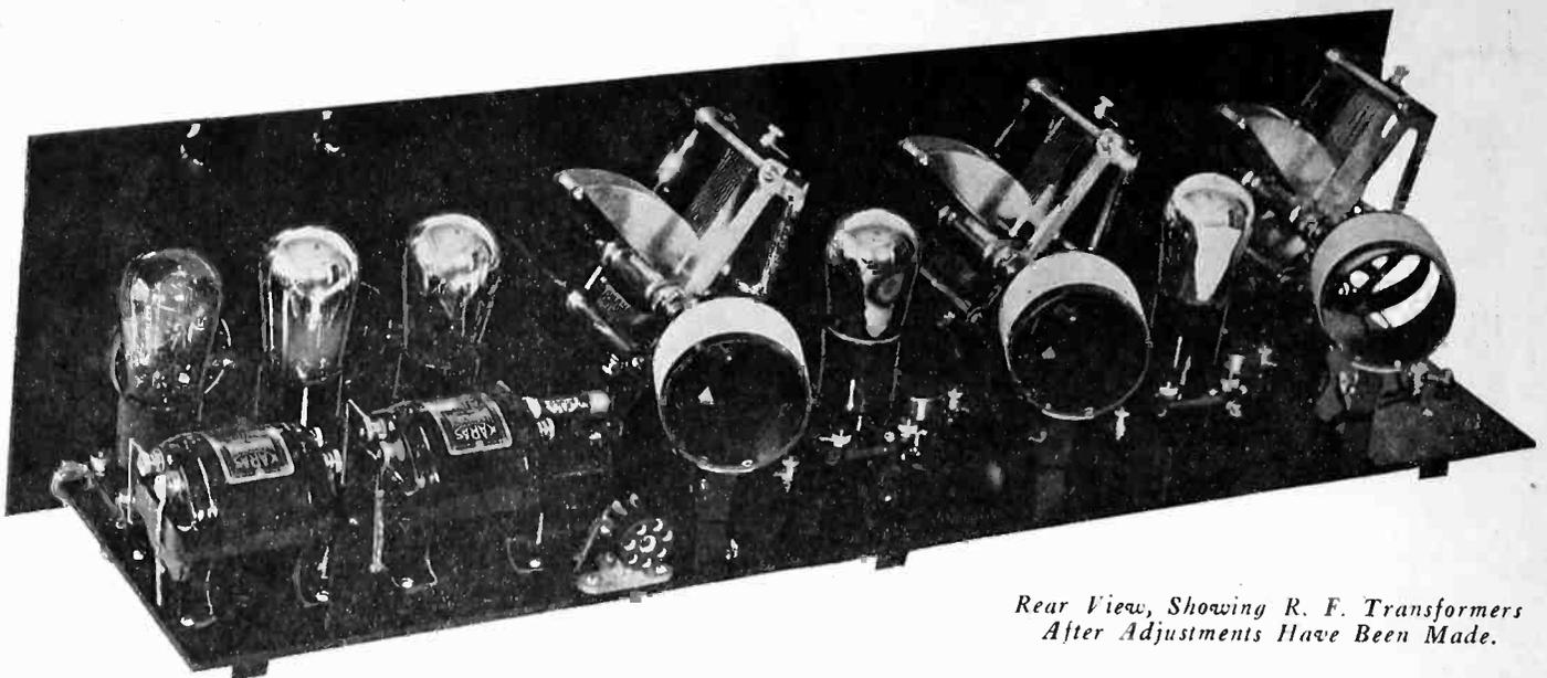
Rear View, Showing R. F. Transformers After Adjustments Have Been Made.
