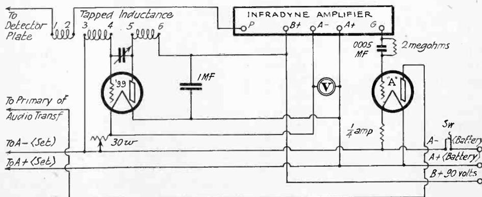
Fig. 1. Circuit Diagram for Infradyne Adapter.
