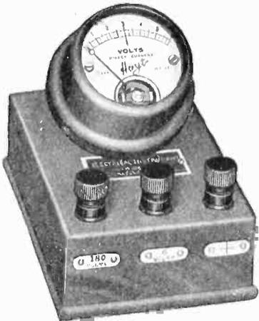
A HOYT 17-B Voltmeter, with high-resistance, moving-coil movement, and a hand-calibrated scale, 0-6 volts, marked in red at 3. Two tips are provided at the rear, for insertion in the panel tip-jacks, provided for the purpose in the R. C. A. Radiolas Nos. 20, 25, 26 and 28, and all the similar sets.
