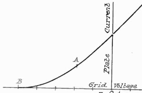
Fig. 1. Relation Between Grid Voltage and Plate Current.
