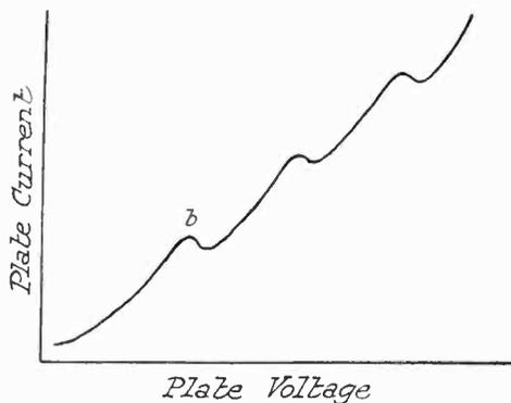
Fig. 3. Characteristic Curve of "Soft" Tube.
