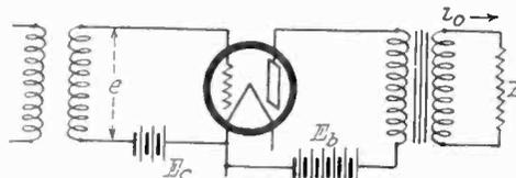
Fig. 2. Detector Tube With Output Transformer.
