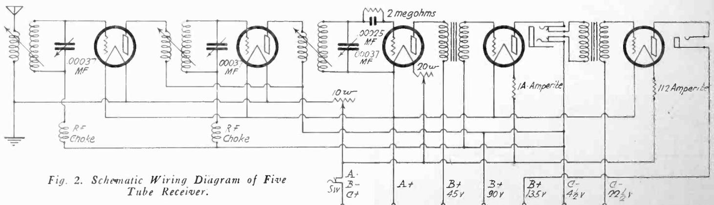
Fig. 2. Schematic Wiring Diagram of Five Tube Receiver.
