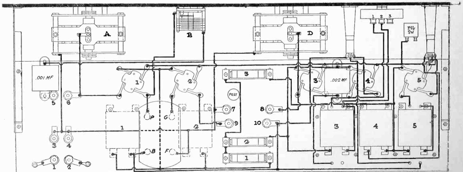
Fig. 2. Pictorial Wiring Diagram Showing Connections as Actually Made.
