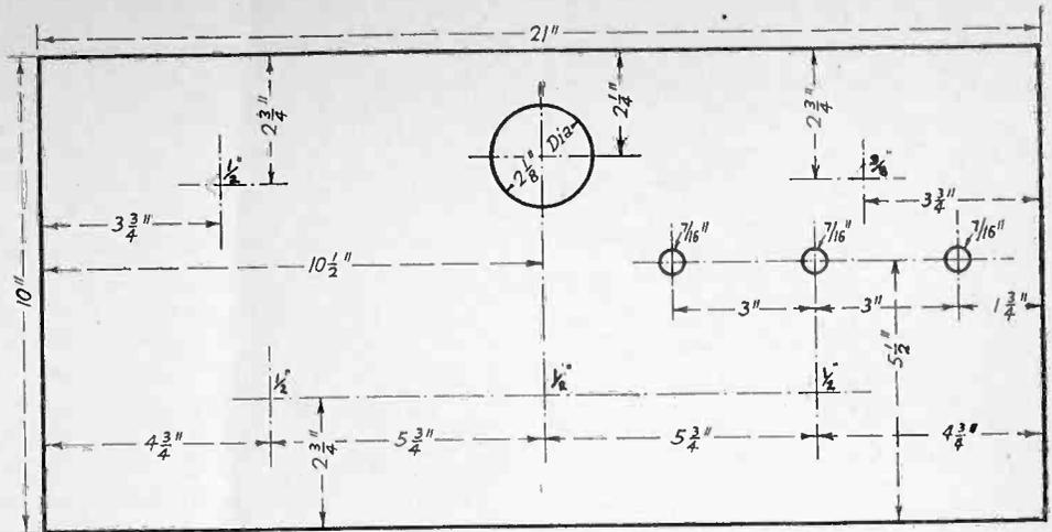
Fig. 2. Panel Layout for Shielded Superheterodyne.
