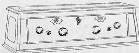
Bottom—The Valleytone Model 52 Radio Receiver. Five-tube, tuned radio frequency. Twodial control. Wired so that use of power tube is optional.
