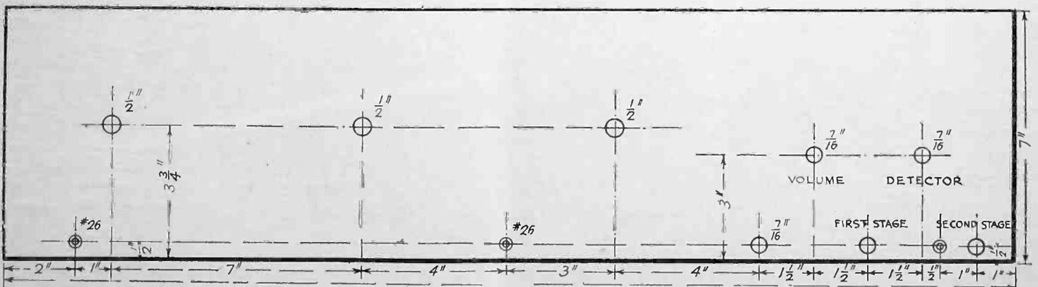
Fig. 3. Panel Drilling Template.
