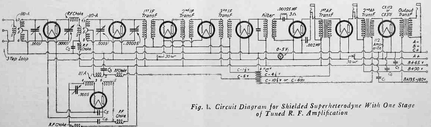
Fig. 1. Circuit Diagram for Shielded Superheterodyne With One Stage of Tuned R. F. Amplification
