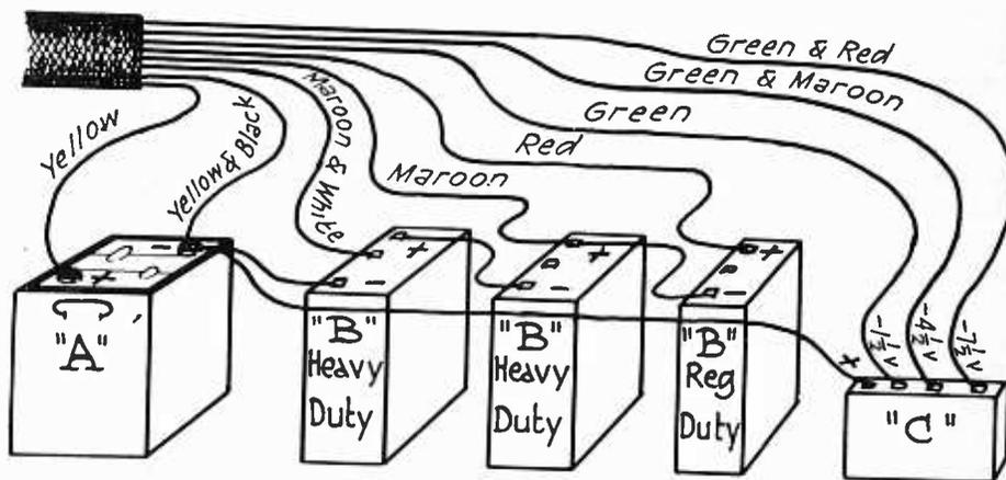
Fig. 3. Arrangement of Battery Cable Connections.
