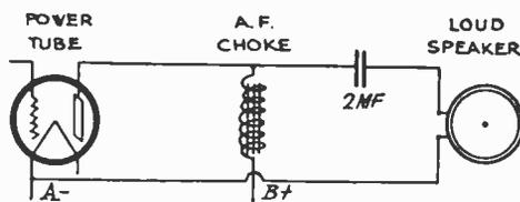
Fig. 1. Impedance Coupling of Loud Speaker.
