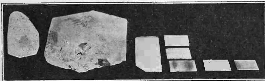
Fig. 1. Various Steps in the Production of a Finished Crystal.
