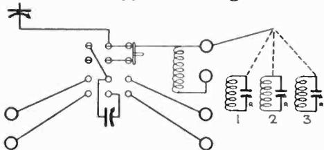
Fig. 2. Connections for Calibrating Single Control Receiver.
