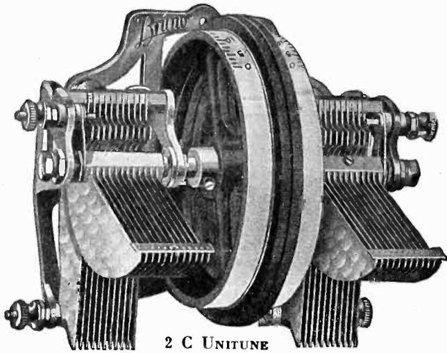
This basic Unit consists of two .0005 mfd. bakelite shaft condensers, controlled by a split drum with graduated scale, mounted in an aluminum frame.
