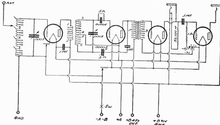
Fig. 3. Circuit of Four Tube Regenerative Receiver.
