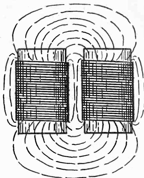
Fig. 2. *Electromagnetic Field of Astatic Pair.*
