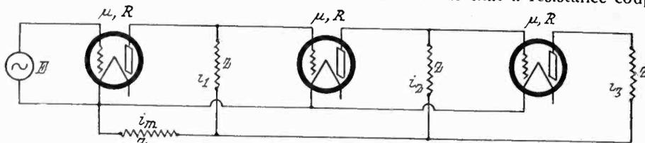
Fig. 2. Three-Stage Direct Coupled Amplifier.
