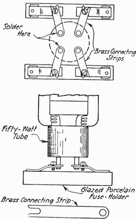
Fig. 1. Home-Made Socket for 50-Watt Tube.
