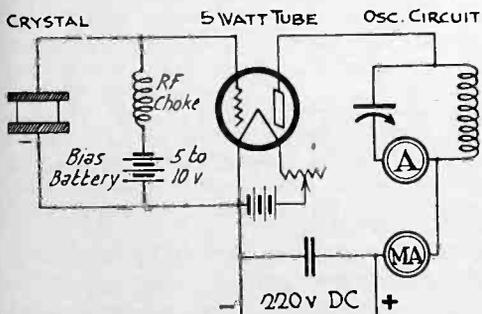
Fig. 6. Crystal Testing Circuit.
