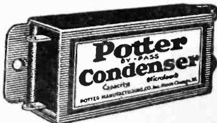
The plates are of tin foil and the insulation is linen paper and wax impregnation, all hermetically sealed in a case fitted with tinned copper terminals.
