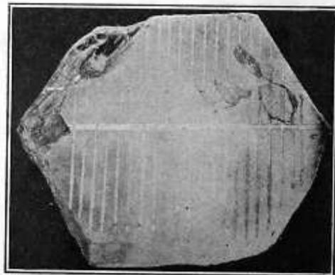
Fig. 5. Position of Electric Axis as Indicated by Heavy Line and Proper Cutting of Slices as Shown by Ruled Lines Perpendicular Thereto.
