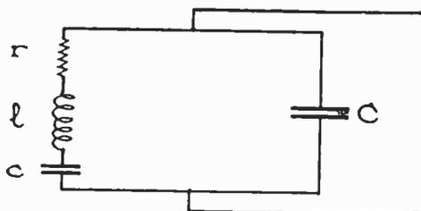
Fig. 4. Electrical Circuit Equivalent to a Thin Vibrating Crystal.
