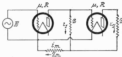
Fig. 1. Two-Stage Direct Coupled Amplifier.
