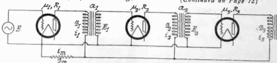
Fig. 4. Typical Audio Frequency Amplifier.
