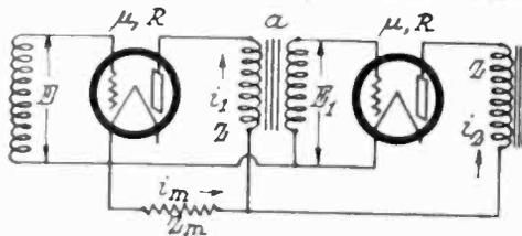
Fig. 3. Two Tubes and One Transformer.
