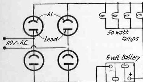
Fig. 1. The Electrolytic Battery Charger Circuit.
