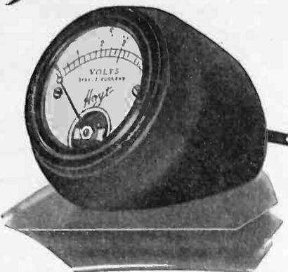
The HOYT "SUPER" Control Meter is a 2-inch, Type 17, moving coil voltmeter, 0-6 volts, marked in red at 3 volts, and fitted with 3-foot silk covered cord-tips for plugging into the tip-jacks on Radiolas Nos. 20, 25 and 28, and all other similar sets with tip-jacks in the filament circuits. Permits exact adjustment of proper filament brightness. Improves reception and insures maximum life of the tubes. It may be placed anywhere on or near set. In polished mahogany case with non-scratch base.
