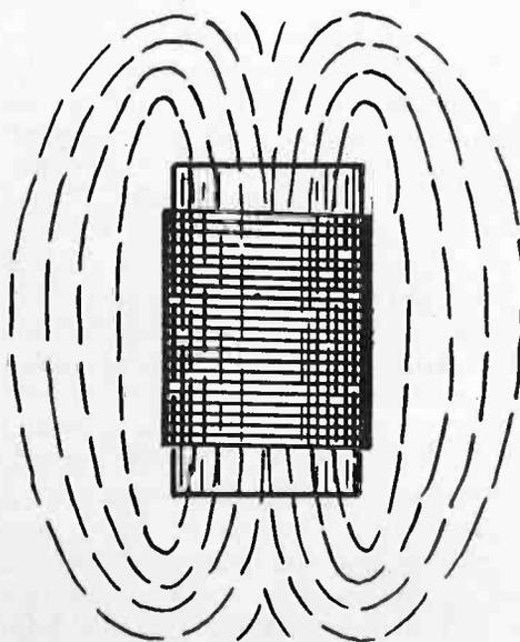
Fig. 1. *Electromagnetic Field of Solenoid.*
