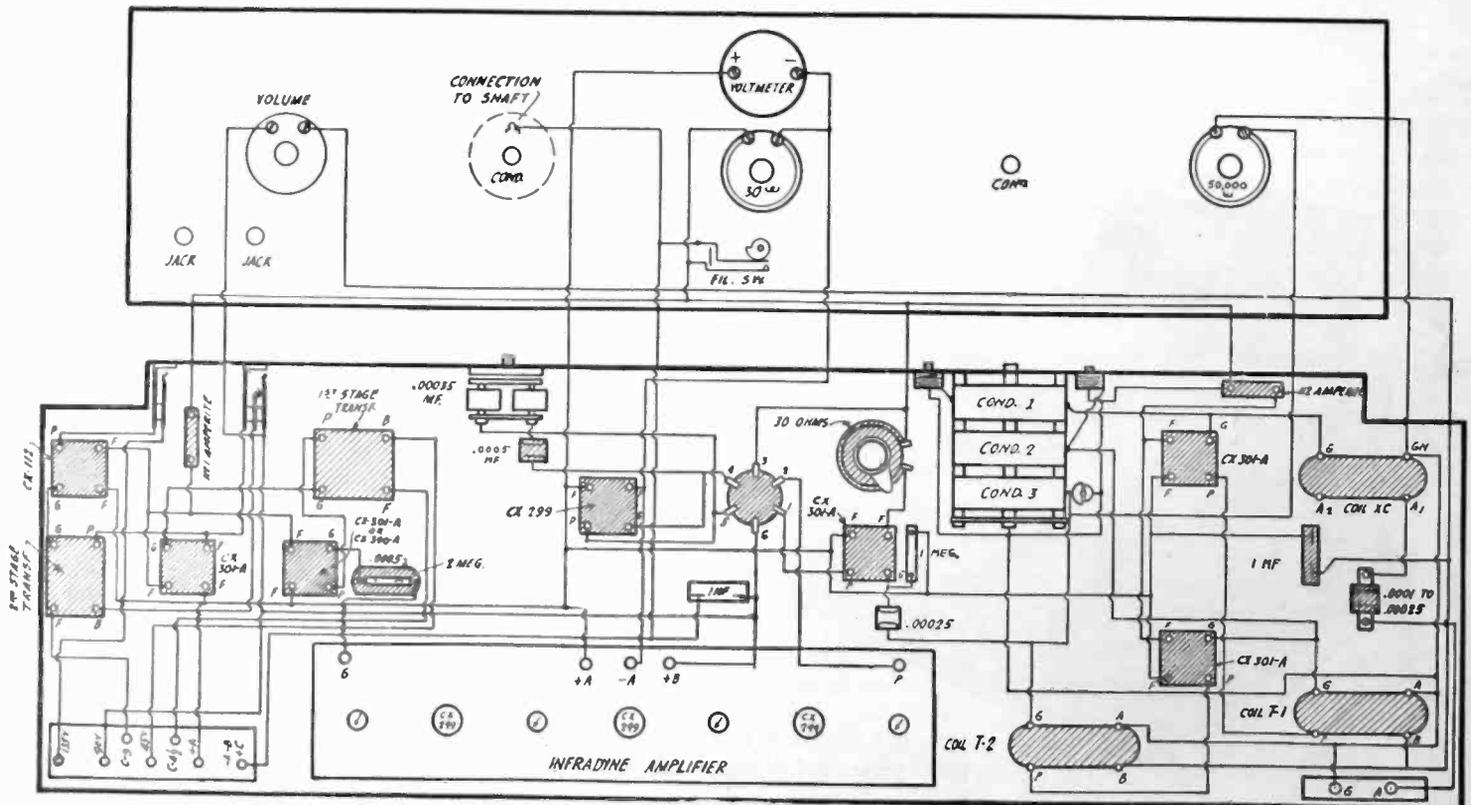
Fig. 5. Pictorial Wiring Diagram.
