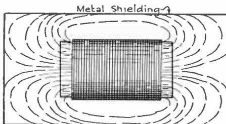
Fig. 5. Shielded Solenoid.
