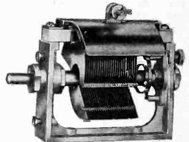
and are guaranteed to be accurate within 1 per cent of their rated capacitances. They are small and compact and built to a tolerance of .001 in. With their one-hole mounting they can be placed either horizontally or vertically. The rotor is grounded.
