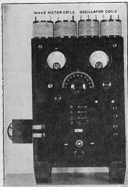
Panel View of Oscillator-Wavemeter.
