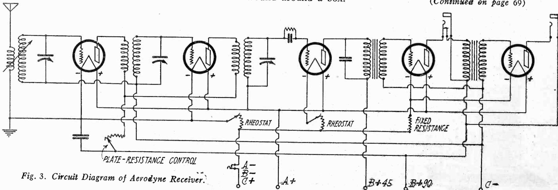
Fig. 3. Circuit Diagram of Aerodyne Receiver.
