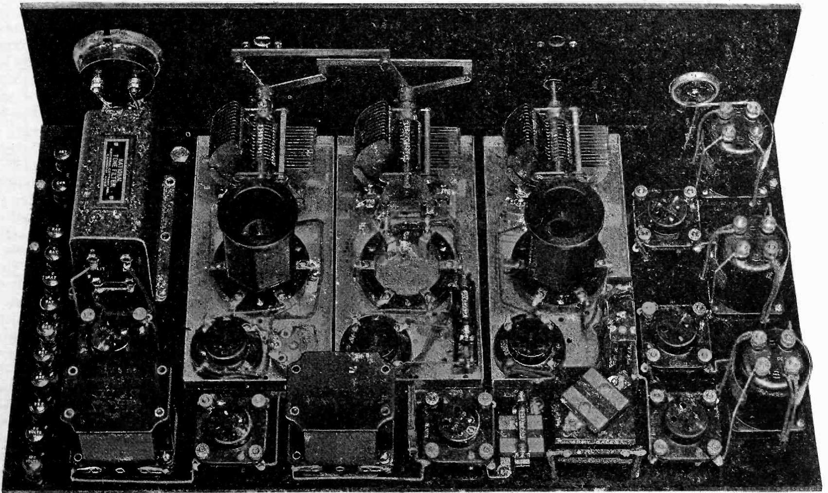
Rear View of Receiver, with Shields Removed.
