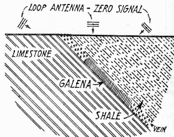
Fig. 3. Effects of Magnetic Field Near Vein.
