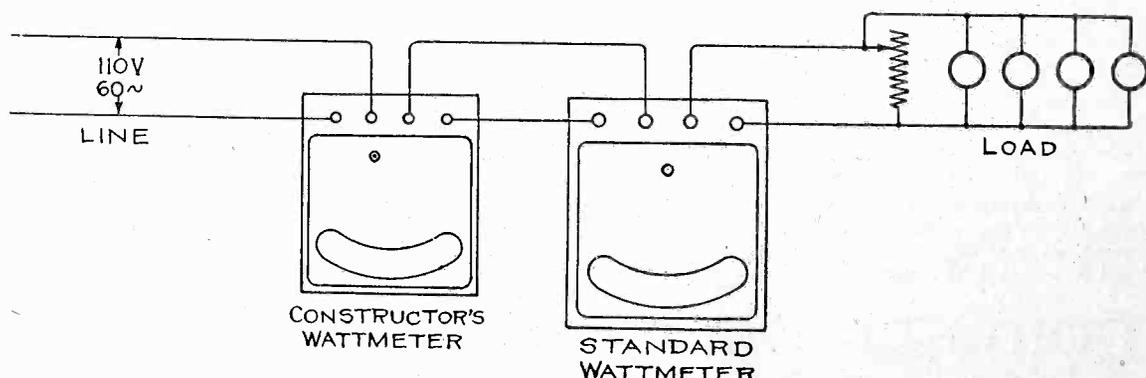
Fig. 8. Calibration Set-up.
