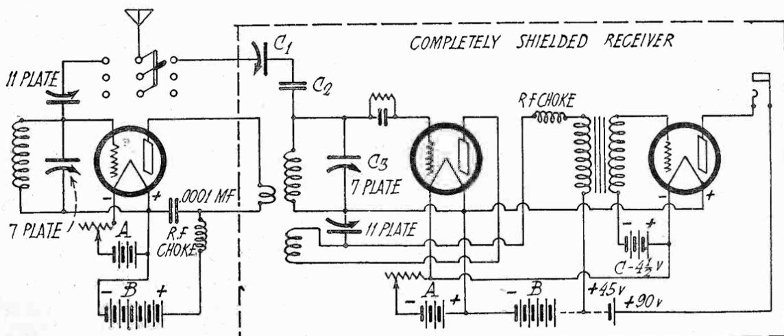
Circuit Diagram for Browning-Drake 30 Meter Receiver.
