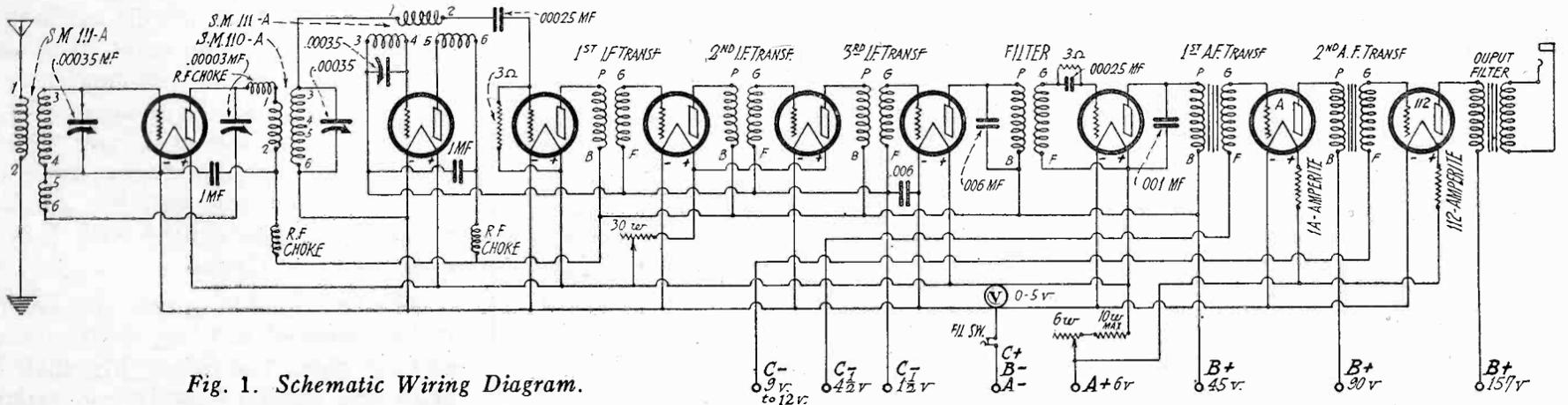
Fig. 1. Schematic Wiring Diagram.
