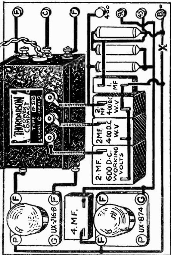
B-ELIMINATOR AND SUPPLY FOR UX-210 POWER AMPLIFIER-
