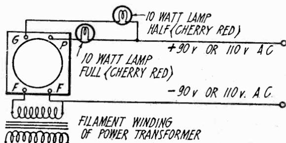
Circuit for Testing Rectifier Tube.
