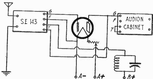
Fig. 2. Adaptation of Superdyne to S. E. 143 Receiver.
