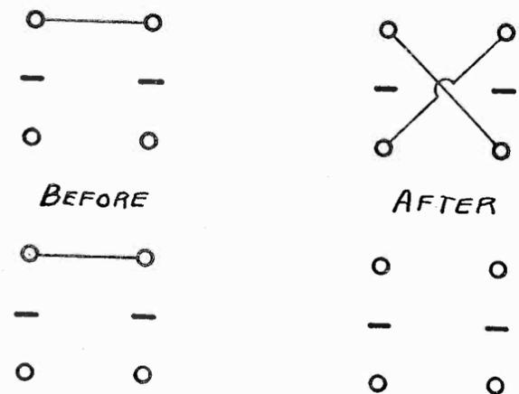
If the connections on the "OSCLR-DET" key switch on the tube control panel are changed as shown in the diagram, this switch may be used to reverse the tickler connections when on the "DET" position instead of cutting out and shorting the tickler coil as it does normally. Simply remove the two wires shown in Fig. 1 and connect the two shown in Fig. 2.
