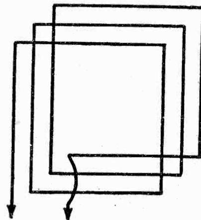
Fig. 2. Solenoid Loop.
