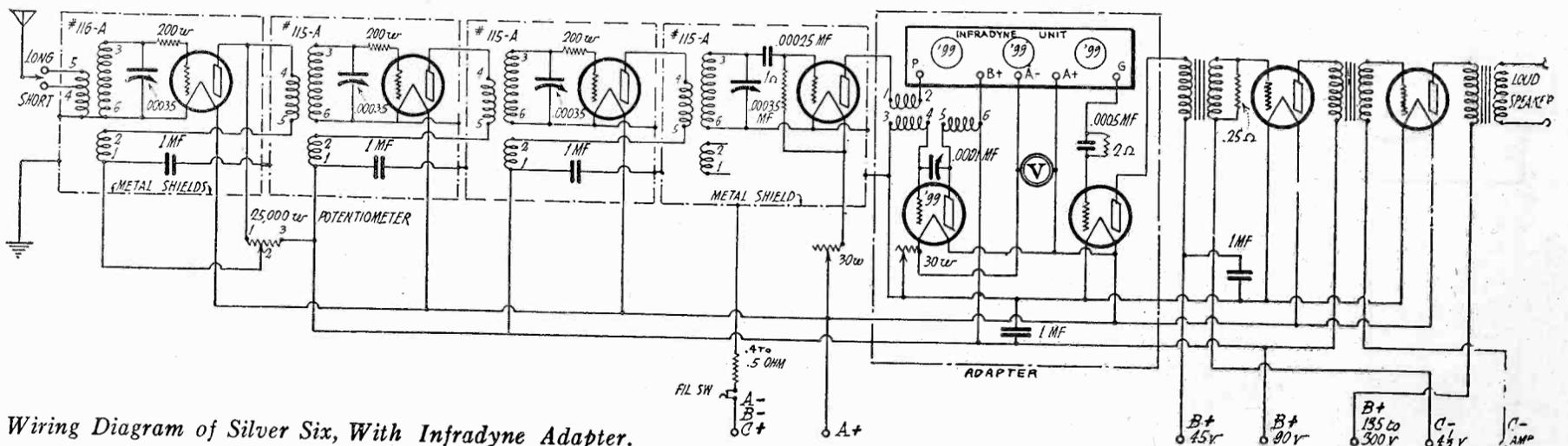
Wiring Diagram of Silver Six, With Infradyne Adapter.
