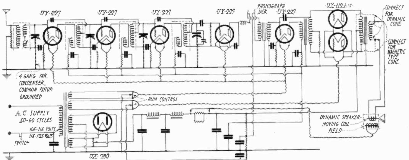
Fig. 2. Circuit Diagram of Model 33 Gilfillan Neutrodyne
