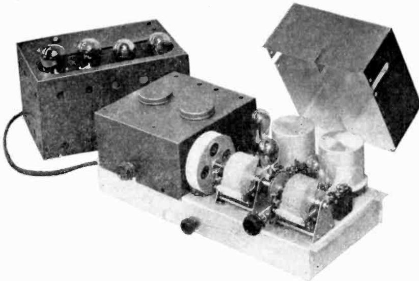
Fig. 1. Chassis for Model 33 Gilfillan Neutrodyne
