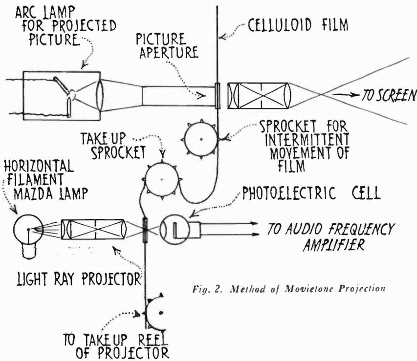
Fig. 2. Method of Movietone Projection
