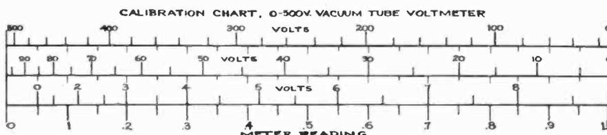
Fig. 7. Chart for Quick Reading of Calibration
