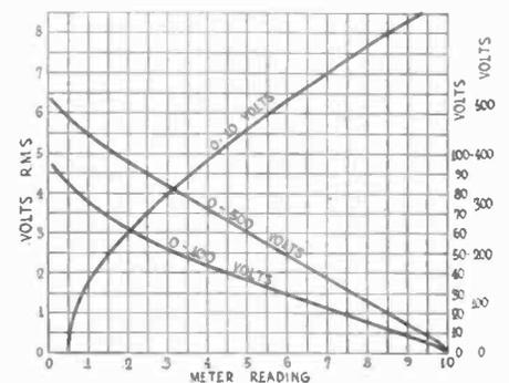
Fig. 6. Calibration Curve of Voltmeter
