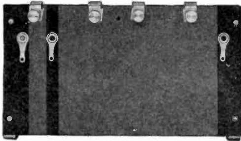
In constructing a plate supply unit eliminate guesswork in the calculation of resistance values. The Type 446 Voltage Divider is wound in two sections, one of 15,000 ohms for the plate supply and one of 1500 ohms for obtaining the bias voltage for a power tube. Each divider is equipped with four adjustable sliders, thus making the voltages easily variable. Price **\$2.75**
