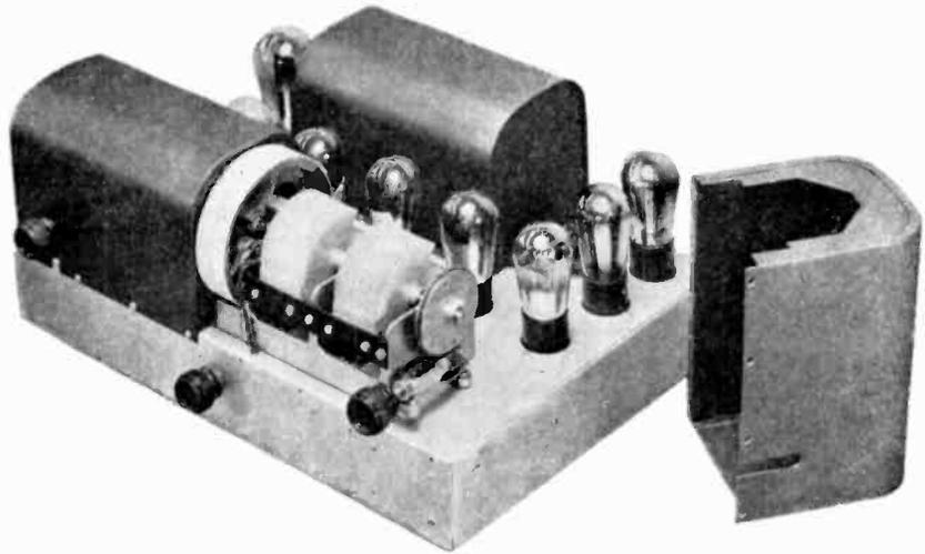
Fig. 3. Chassis of Model 66 Gilfillan Neutrodyne
