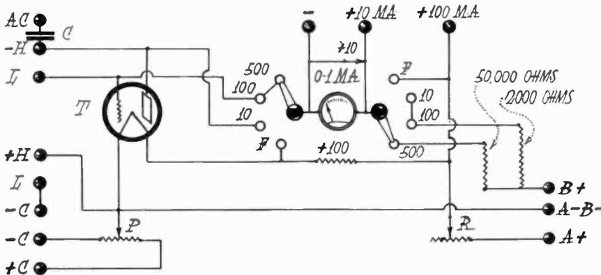
Fig. 1. Circuit Diagram of Vacuum Tube Voltmeter
