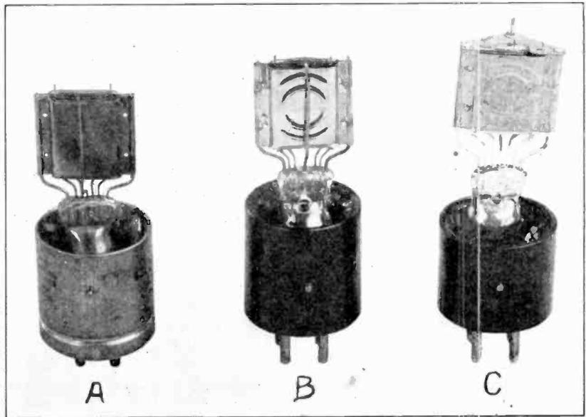
Fig. 2. Changes in Structure of "A" Tube Elements
