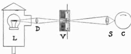
Fig. 2. Optical System Used in Picture Recording
