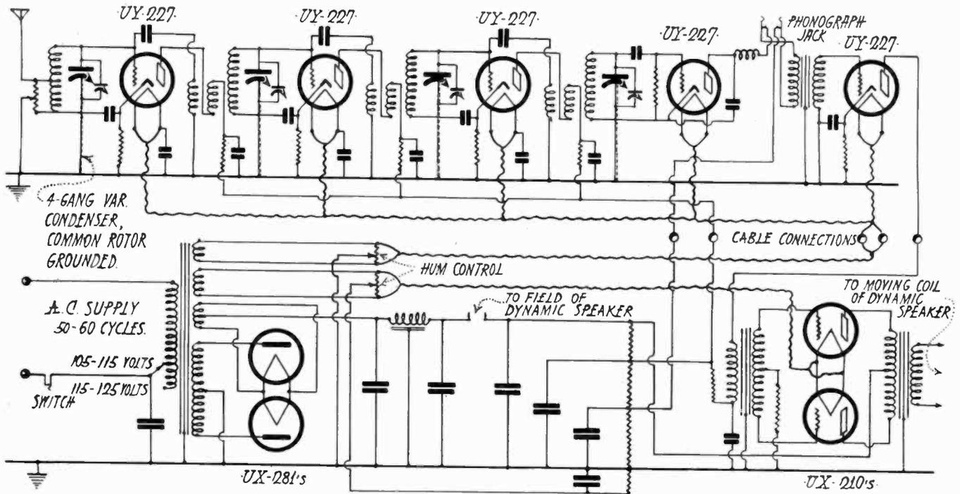
Fig. 4. Circuit Diagram of Model 66 Gilfillan Neutrodyne
