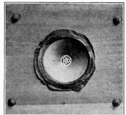
Fig. 3. Cone in Place on Baffle Board
