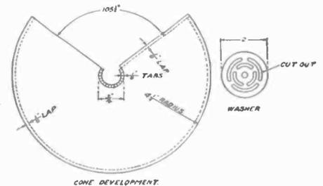
Fig. 2. Layout of Cone and Centering Washer
