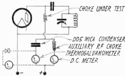
Fig. 1. Circuit for Testing R. F. Chokes
