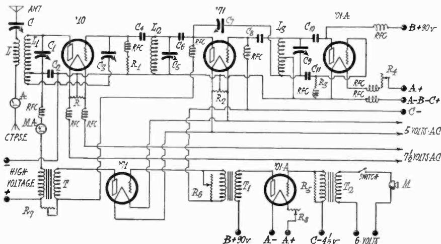
Fig. 1. Circuit of 20-Meter Radiophone Transmitter
