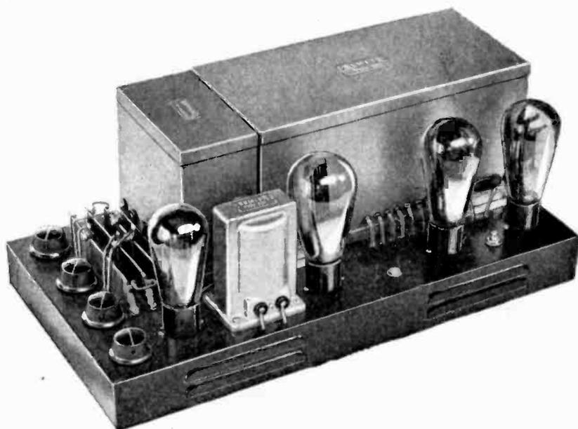
Remler Power Amplifier and B Supply for 350 Tubes and Dynamic Speaker
