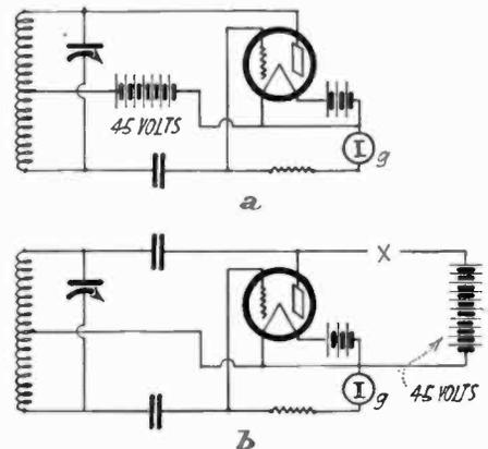
Fig. 2 (a). Series Feed Hartley for Comparison Test
