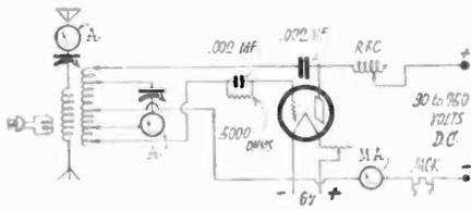
Fig. 1. Circuit Diagram of 80-Meter Phone Transmitter
