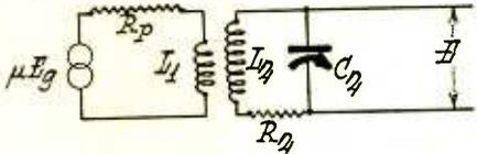
Fig. 5. Equivalent of A.C. Circuit of Screen-Grid Tube With Tuned R.F. Transformer
