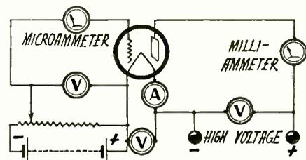
Fig. 1. Circuit for Measuring Gas Content of Vacuum Tube
