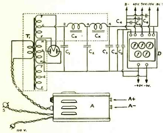
Fig. 1. Wiring Diagram for "A," "B" and "C" Unit
