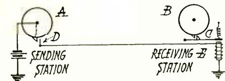
Fig. 3. "Stop-Start" Method of Synchronism
