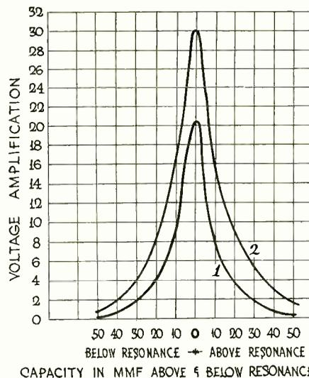
Fig. 7. Resonance Curves of a Tuned R.F. Transformer (1) and a Tuned Impedance (2)
