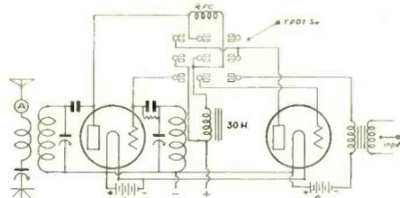
Scheme for Converting from CW to Phone
