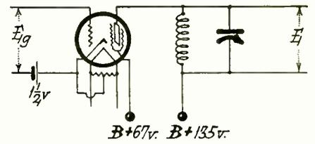
Fig. 8. Circuit of Screen-Grid Tube With Tuned Impedance
