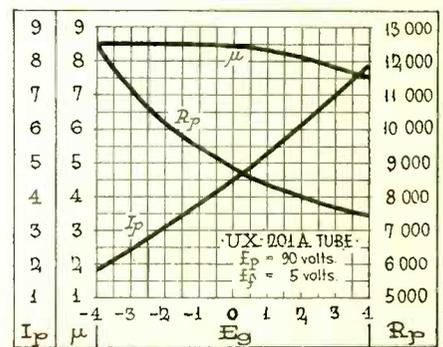
Fig. 3. Amplification and Plate Resistance of '01-A Tube
