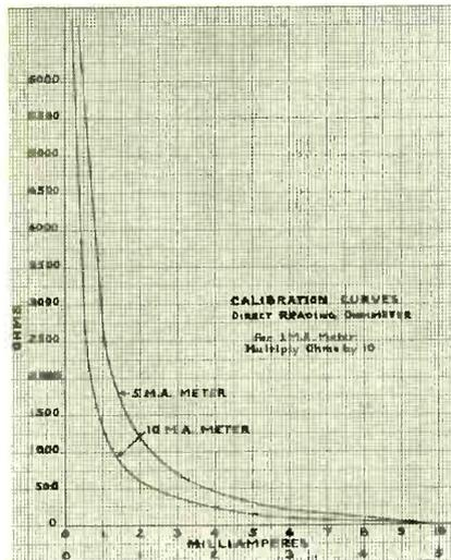
To obtain a calibration curve, values of  $i$  are chosen, which are scale divisions of the meter, and these values are inserted in the equation. A number of points are thus obtained from which a curve may be plotted. A handier method than a calibration chart is to make a new scale for the meter with the resistance values on it so the instrument is direct reading. A reproduction of the
