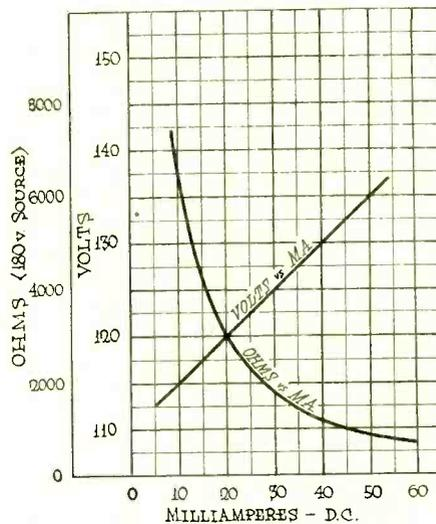
Fig. 6. Value of Current-Limiting Resistance and Internal Impedance
