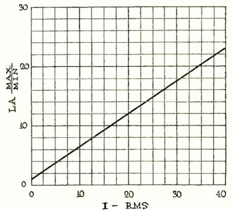
Fig. 3. Variation in Brightness With Change in Alternating Current
