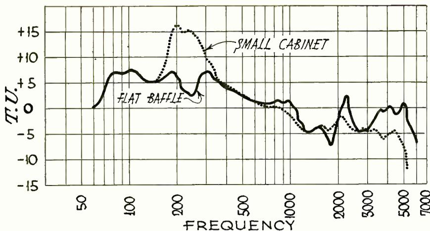
Fig. 2. Response Curve for Small Cabinet and Flat Baffle, Measured 5 Ft. from Speaker
