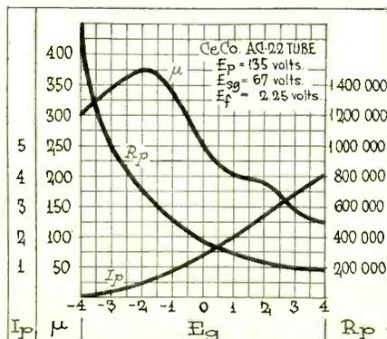
Fig. 2. Amplification and Plate Resistance of A.C. Screen-Grid Tube
