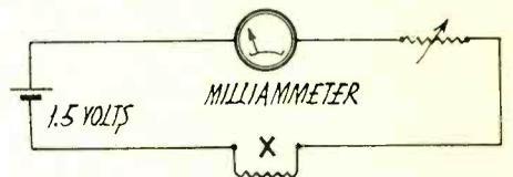
Circuit Diagram for Direct Reading Ohmmeter
