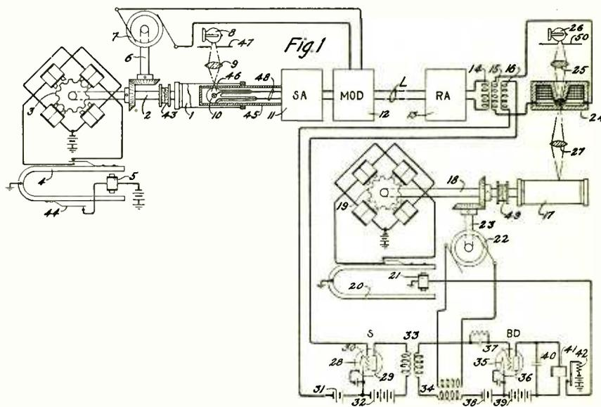
Fig. 4. Tuning Fork Method of Synchronism
