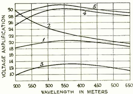
Fig. 6. R.F. Gain With Various Tubes and Tuned Circuits
