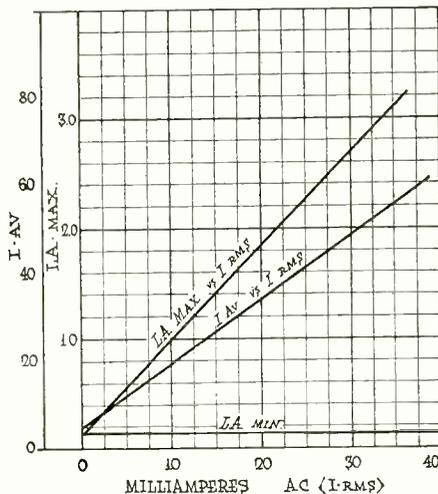
Fig. 2. Relation of I-RMS and of Brightness to I-AV
