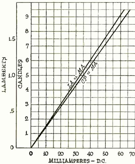
Fig. 1. Relation of Light Output and Brightness to D. C. Current
