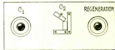
Fig. 1. Panel Mounting of the Strip Holder
