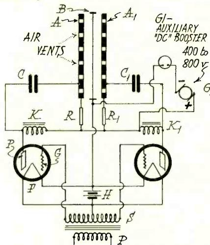
Fig. 6. Diagram of Connections for Bilateral Speaker
