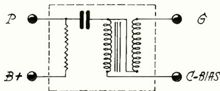
Fig. 3. "Resonated" Transformer
