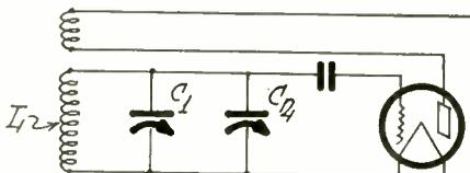
Fig. 3. The Tuning Condenser and the Auxiliary Condenser Are Paralleled
