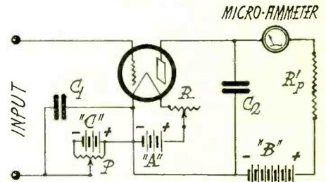
Fig. 5. Circuit Diagram of Vacuum Tube Voltmeter
