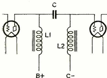
Fig. 2. Tuned Double Impedance System
