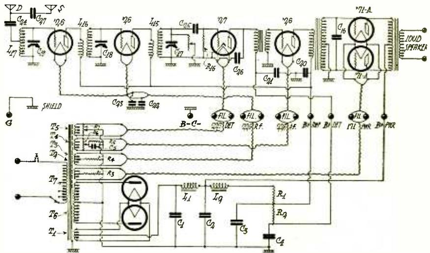
Circuit Diagram of Federal Type H Ortho-Sonic Receiver
