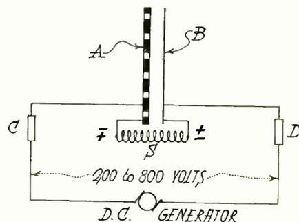
Fig. 3. Method of Applying Polarizing Voltage to Unilateral Speaker
