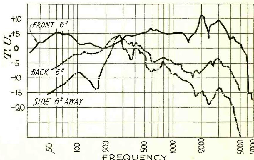
Fig. 1. Response Curve of Dynamic Speaker in Small Cabinet, Measurements Taken 6 In. from Front
