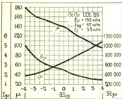
Fig. 1. Amplification and Plate Resistance of D.C. Screen-Grid Tube
