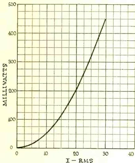
Fig. 5. Relation of Current Output to Power Output
