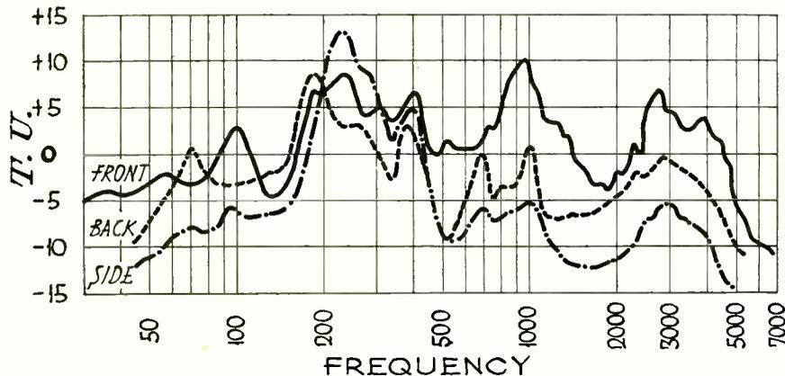
Fig. 3. Response Curve for Small Cabinet, Sound Measured 5 Ft. from Speaker
