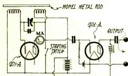
Fig. 1. Magneto-Striction Oscillator
