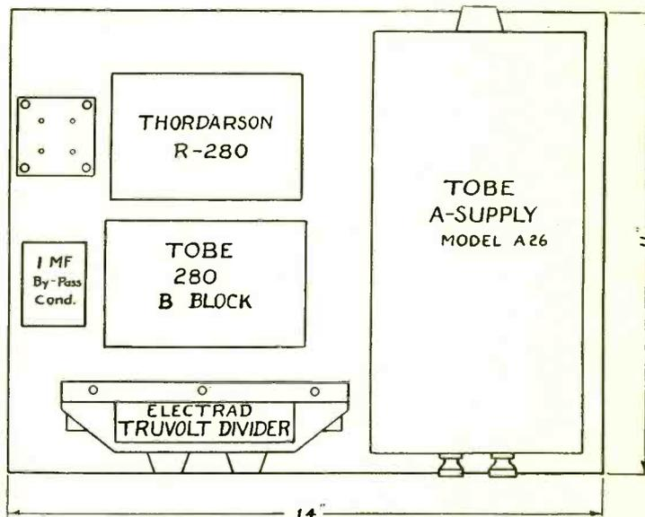
Fig. 2. Placement of Parts in Unit
