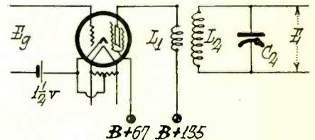
Fig. 4. Circuit of Screen-Grid Tube With Tuned R.F. Transformer
