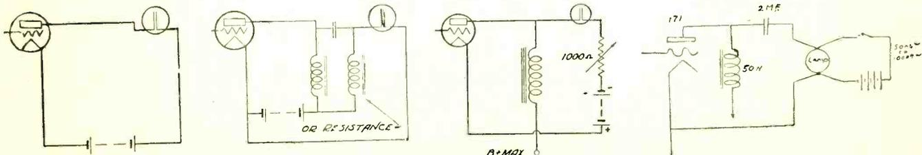
Fig. 7. Methods of Coupling Lamps in Circuits
