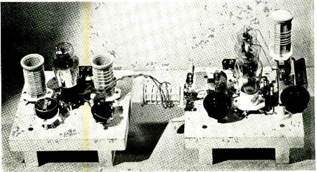
**The Push-Pull 807 Amplifier with 10-Meter Coils. Being Driven by the Special 6L6 Exciter Described Elsewhere in This Issue.**
