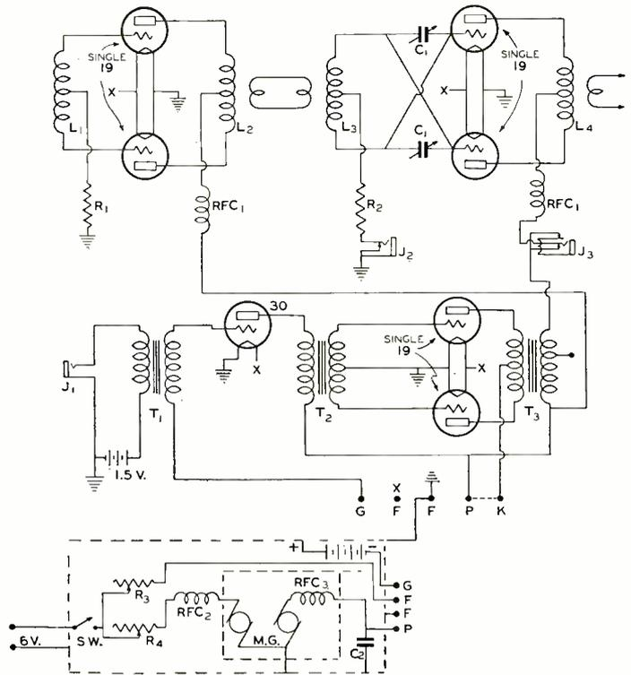
The Portable-Mobile 5-Meter M.O.P.A. Transmitter
