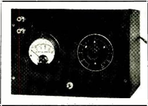
The Vacuum Tube Voltmeter Described in the Text.
