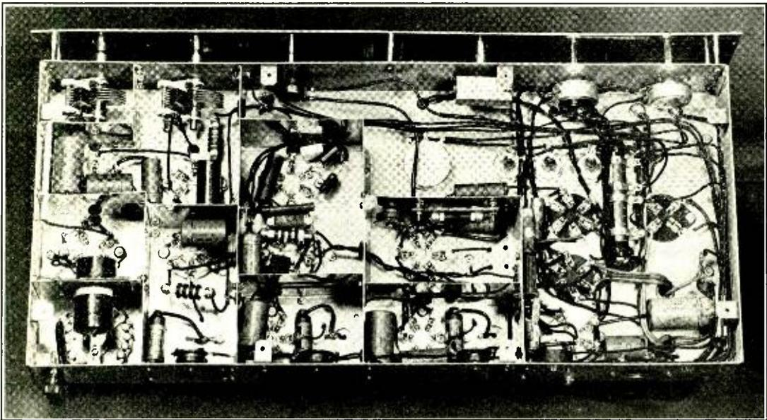
Under Chassis View. Note Shield Partitions and Many By-pass Condensers. Resulting in Good Circuit Isolation.
