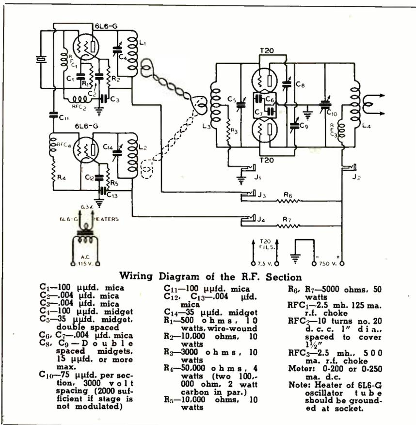
only necessary to move the final grid link from the oscillator tank to the doubler tank to change from 7 or 14 to 28 Mc. It is advisable, however, to remove the 28 Mc. doubler tube from its socket when this band is not being used. This reduces the load on the oscillator stage in addition to cutting down unnecessary drain on the power supply.
