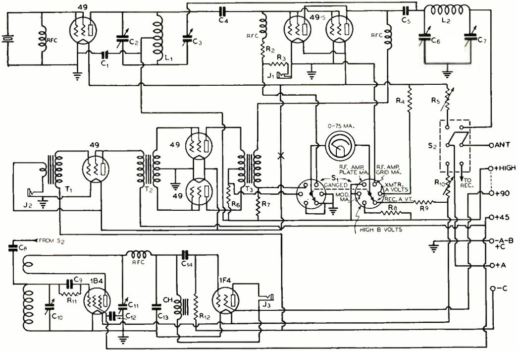
Wiring Diagram of the Portable Unit
