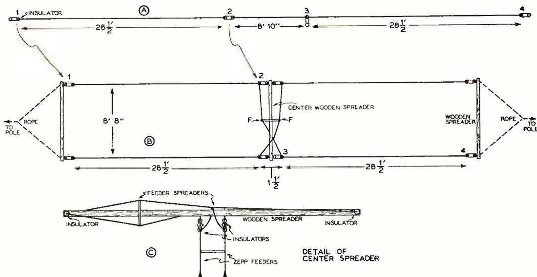
Figure 1: Dimensions of the Flat Top at W8JK. For Ten Meters Divide by 2, for 40 Multiply by 2, Etc.
