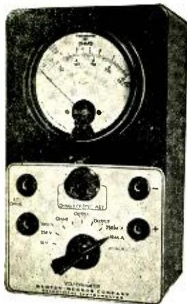
It has a large three-inch meter with two-color scale and accurate D'Arsonval movement with knife-edge pointer and zero adjuster. The d.c. milliamper scale reads 0-1, 0-10, and 0-250. Two output scales are provided, one for the voice coil circuit, the other has a blocking condenser. The two-ohm scales are direct reading: "lo-ohms" from 1/2 to 500, "hi-ohms"
