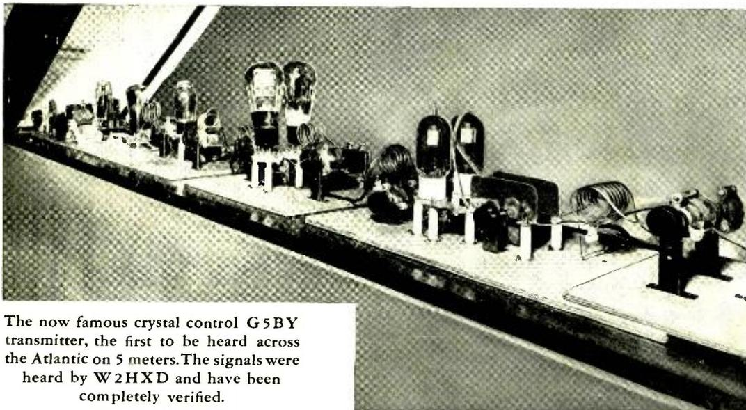
The now famous crystal control G5BY transmitter, the first to be heard across the Atlantic on 5 meters. The signals were heard by W2HDX and have been completely verified.
