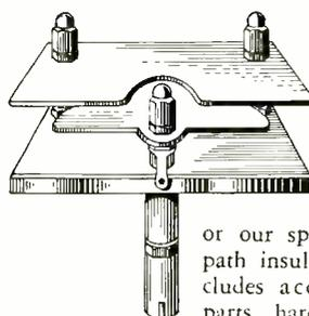
Construct a REAL neutralizing condenser! Adjustable for voltage and capacity range. ('03A, 50T, HF-100, 150T, etc.) Vitrolex insulation
