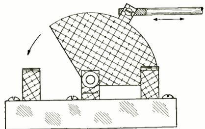
are at each end of the dowel, a cheap means of simultaneously switching antenna, receiver B voltage, and transmitter plate voltage can be had. The blade can be made in a variety of shapes to suit the mounting position or throw length wanted, but the above is satisfactory for most uses. The idea is not new, being used quite extensively back in the spark days when the transmitting antenna was always used for the receiver as well.—W6FFF.
