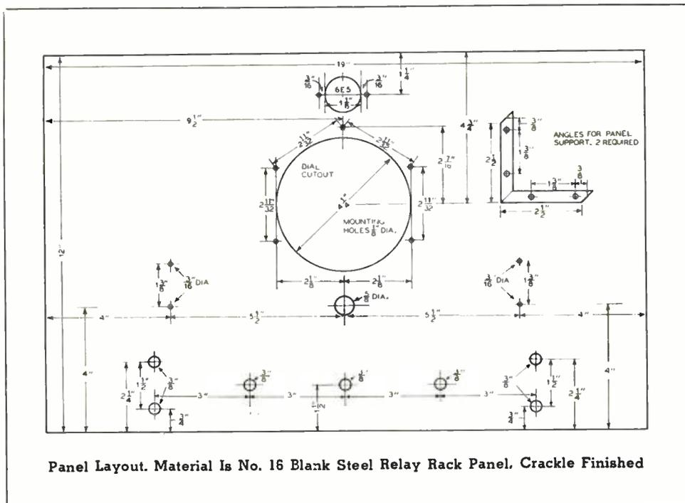
Panel Layout. Material Is No. 16 Blank Steel Relay Rack Panel. Crackle Finished
