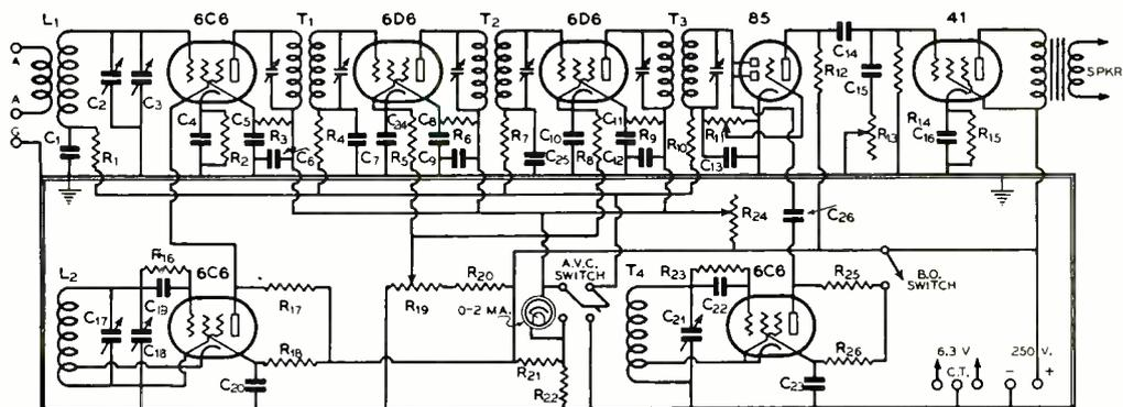
Wiring Schematic of the Superheterodyne
