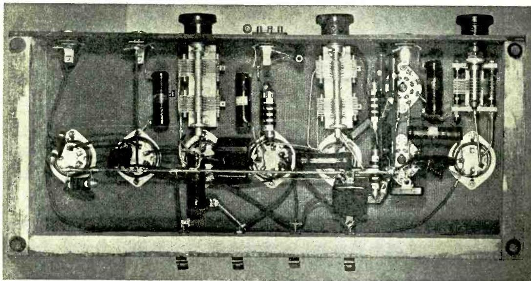
Under-Chassis View of the Exciter. Note the Small Parasitic Choke Between the Lower 6L6 Socket and the Final Coil Socket.
