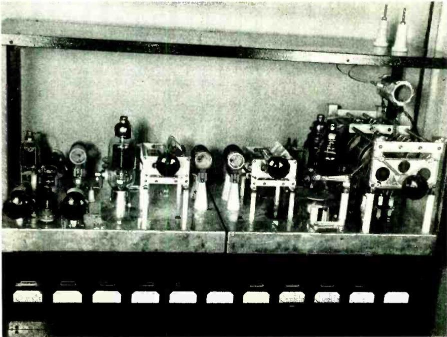
The r.f. section with front panel removed. Note the very neat and efficient mechanical construction for which Brownie is famous.
