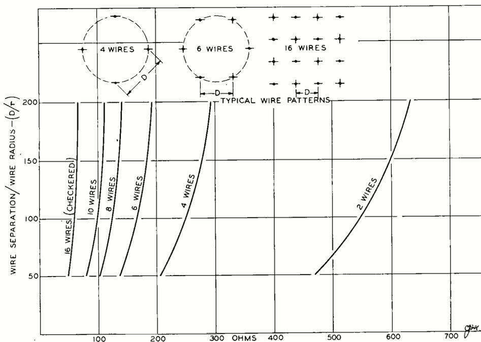
FIG. 1 SURGE IMPEDANCE OF M.C. TRANSMISSION LINE
