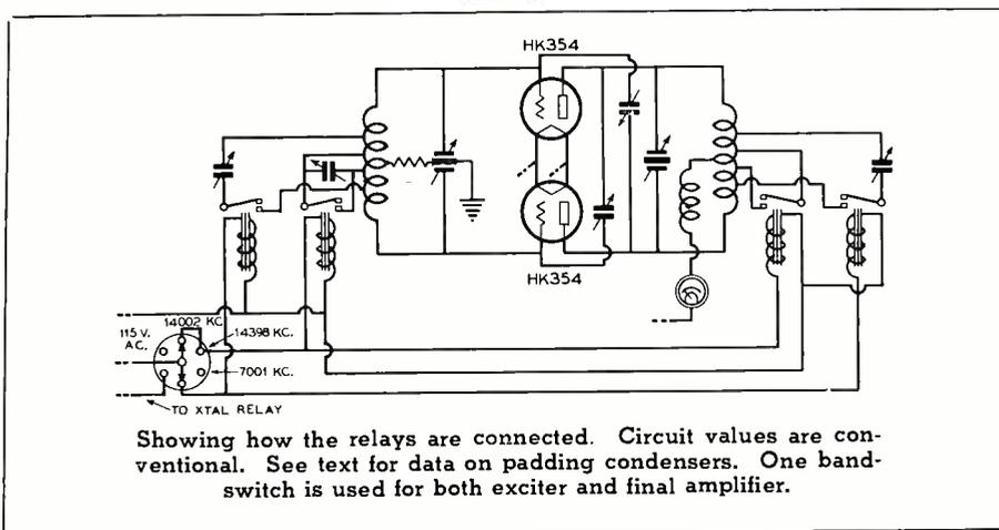
Showing how the relays are connected. Circuit values are conventional. See text for data on padding condensers. One band-switch is used for both exciter and final amplifier.
