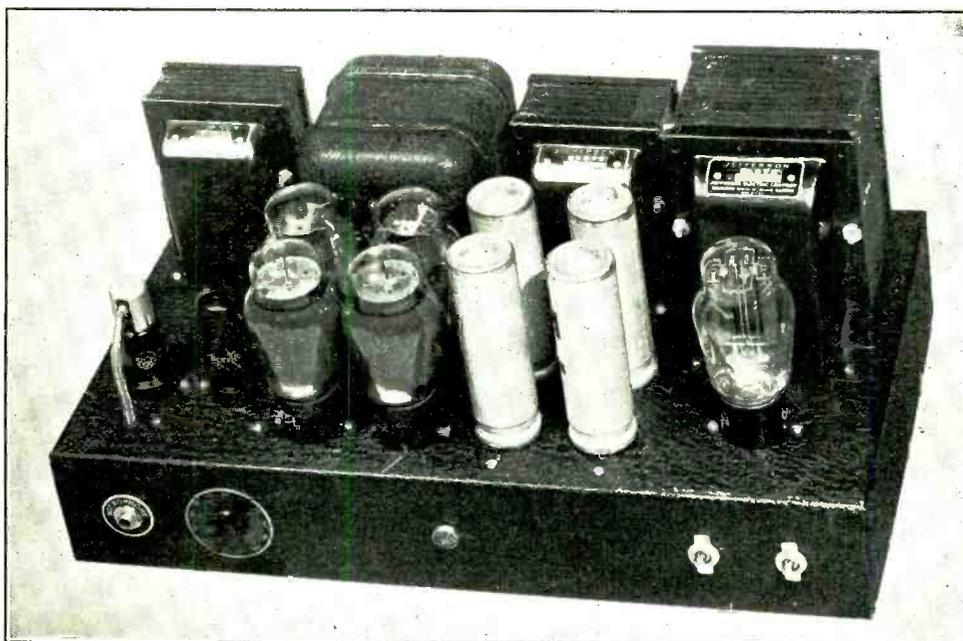
a plate-to-plate load of about 4000 ohms. This value of load was found to give the best output consistent with low distortion. The chart that is furnished with the transformer lists a whole series of loads that the transformer will match with any plate-to-plate load on the primary. In this case (with 4000 ohm primary) output can be obtained at most any impedance
