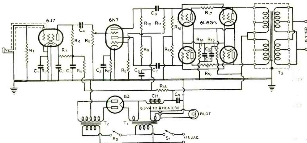
General Wiring Diagram of the Amplifier-Modulator
