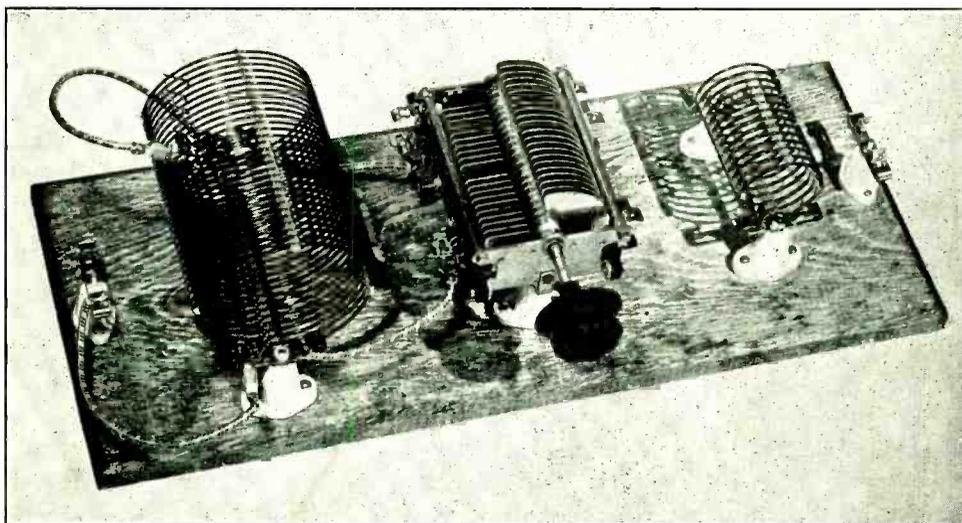
The "Simplex" antenna coupler. It has an infinite number of uses, and is inexpensive to construct.
