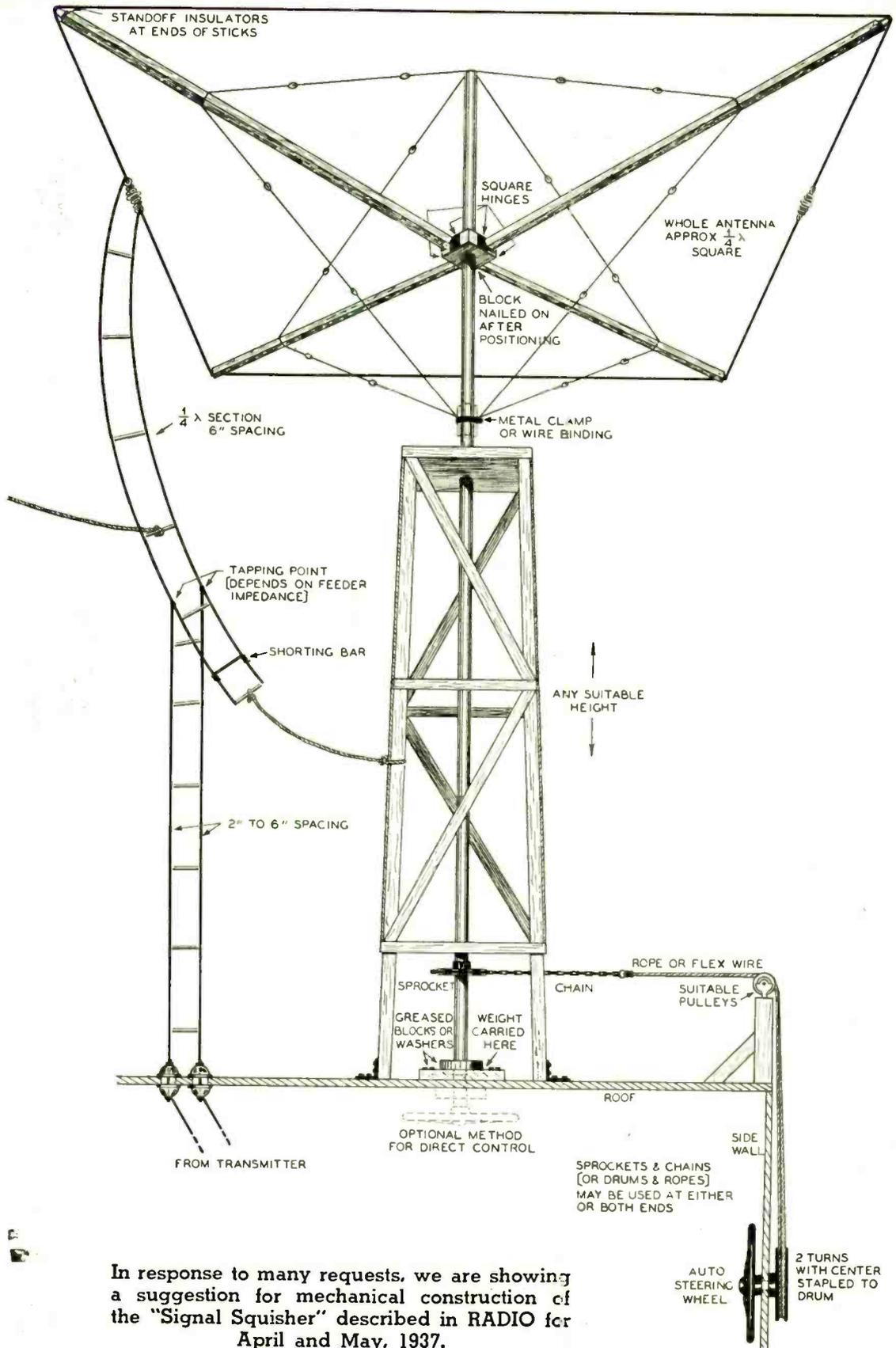
In response to many requests, we are showing a suggestion for mechanical construction of the "Signal Squisher" described in RADIO for April and May, 1937.
