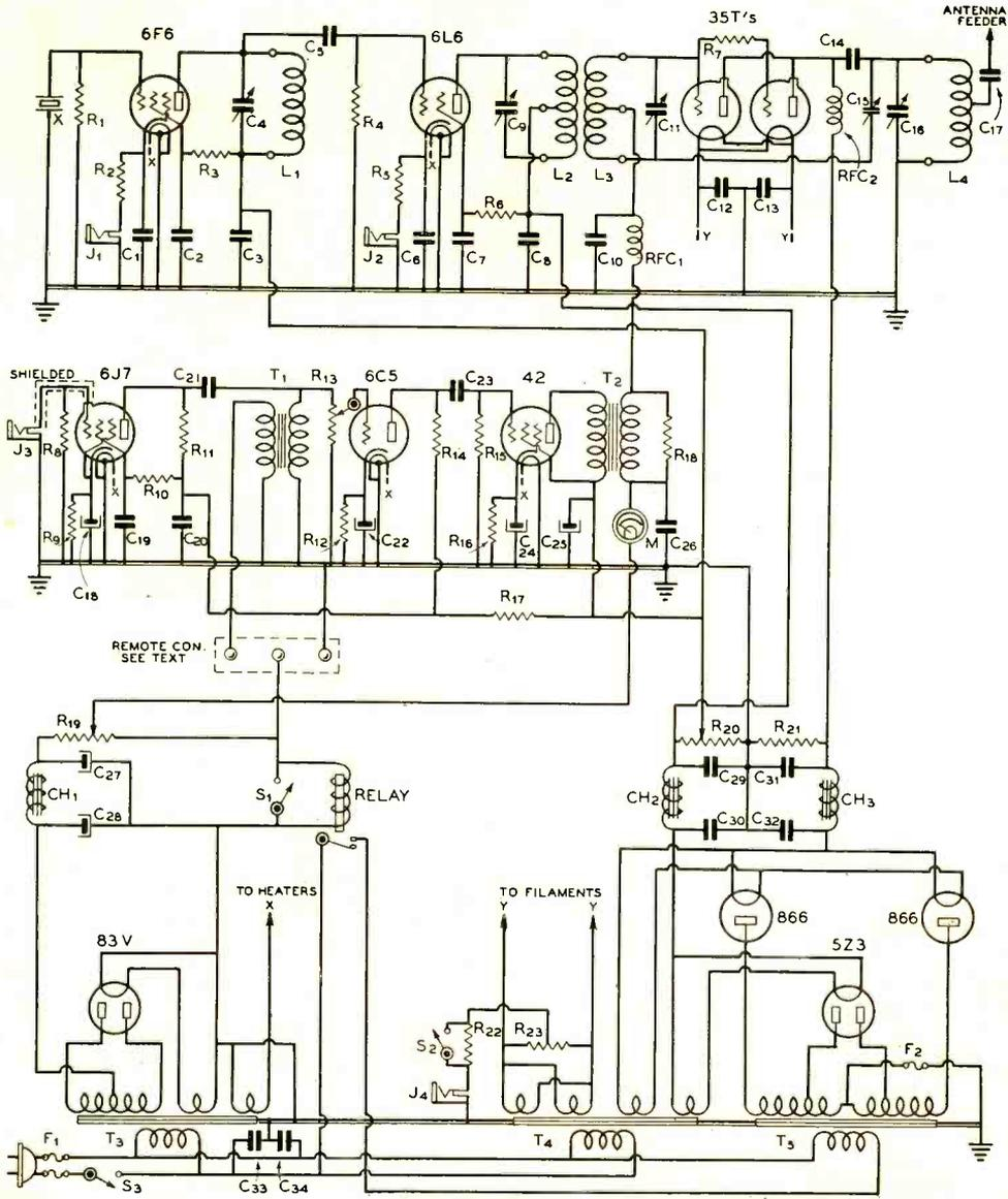
General wiring diagram of the complete transmitter.
