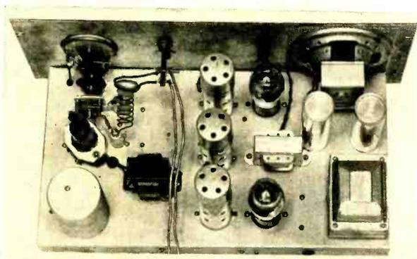
Top view of the improved RC superhet. The can in the lower left corner shields the tuned r.f. choke which is incorporated to increase the i.f. selectivity.
