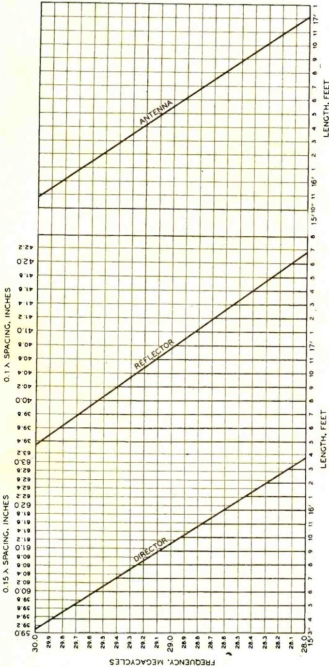
**Dimension Chart for Three-Element Close-Spaced Array.**
