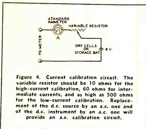
Figure 4. Current calibration circuit. The variable resistor should be 10 ohms for the high-current calibration, 60 ohms for intermediate currents, and as high as 500 ohms for the low-current calibration. Replacement of the d.c. source by an a.c. one and of the d.c. instrument by an a.c. one will provide an a.c. calibration circuit.
