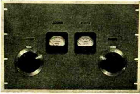
Figure 1. This neat appearing amplifier operates with high efficiency on all bands from 5 to 40 meters, with inputs up to 500 watts.
