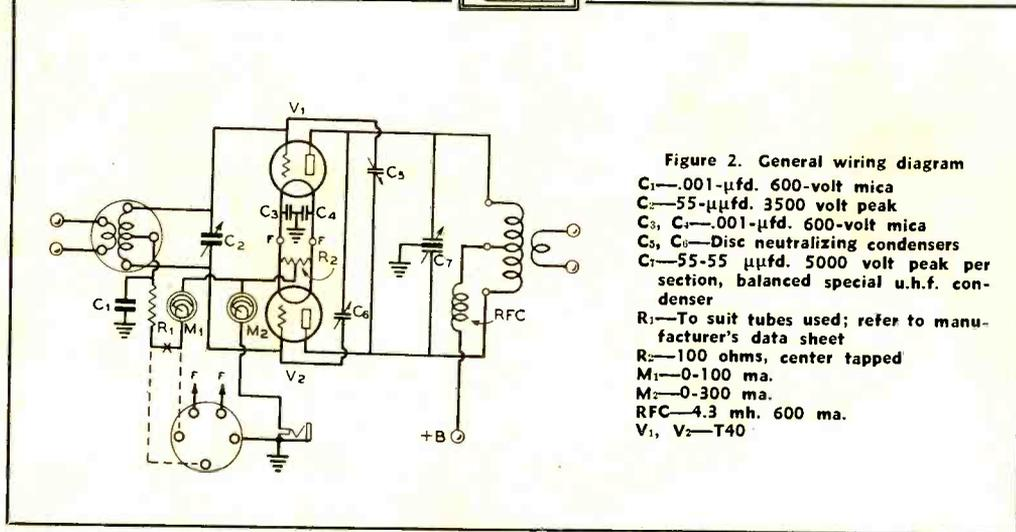
Figure 2. General wiring diagram
