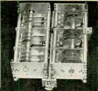
Electrical bandspread at its best results from use of this special 3-gang, triple-section condenser connected in parallel with the 3-gang, double-section main-tuning condenser. Ceramic insulation used for dependability, strength.
