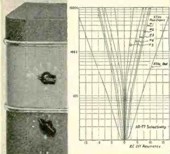
Selectivity is variable in six steps. Curves show degree of selectivity for each step. Note that step #6 has a bandwidth at "two times down" of less than 100 cycles!
