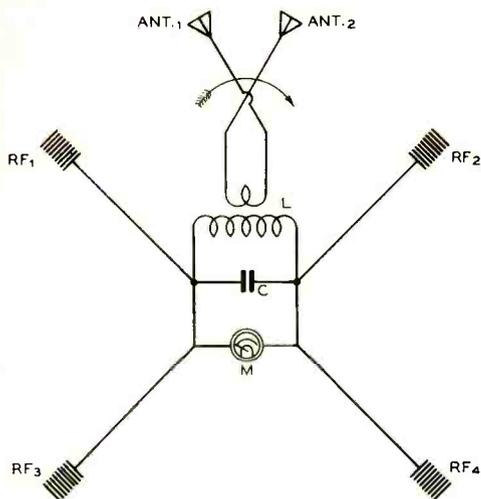
Wiring diagram of the dialogue meter.
