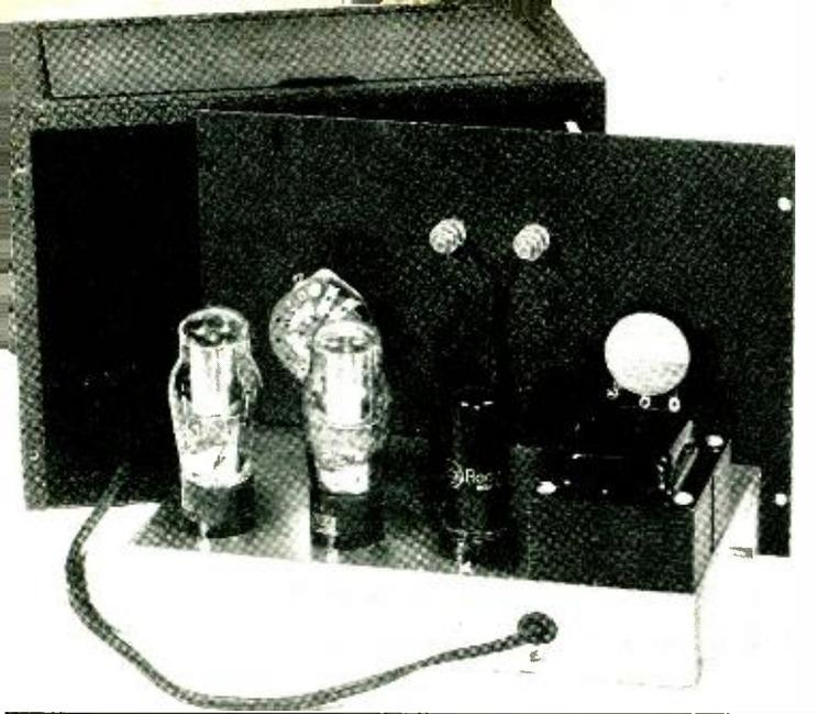
The v.t.v.m. removed from its cabinet. The power transformer, metal rectifier and the two voltage regulator tubes are in a line, from right to left across the rear of the chassis. Rubber grommets are used to insulate the meter terminals where they pass through the panel.
