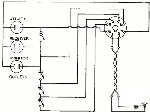
Figure 3. Schematic of the wiring at the operating position.
