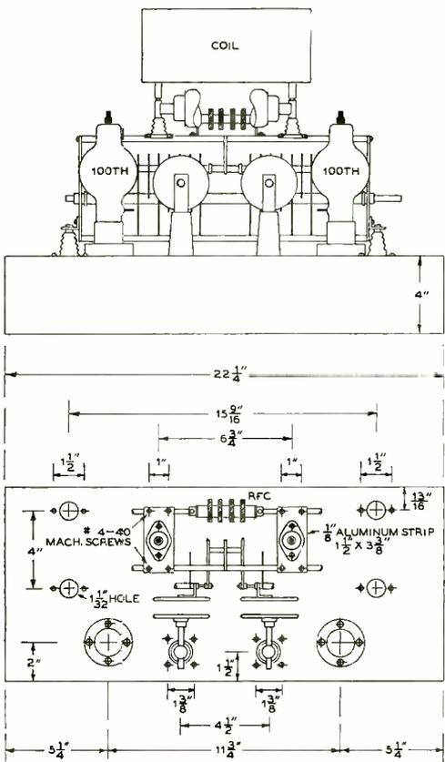
Schematic layout diagram of the final amplifier stage, indicating placement of the various components.
