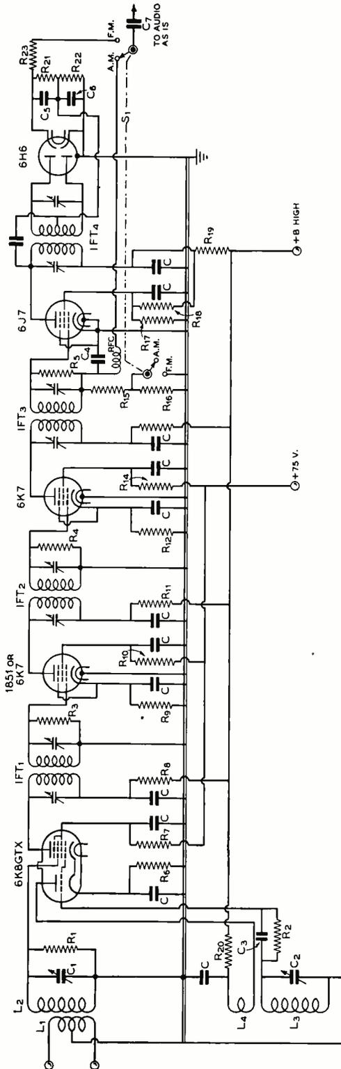
Wiring diagram of the r.f., i.f., and discriminator portion of the receiver.
