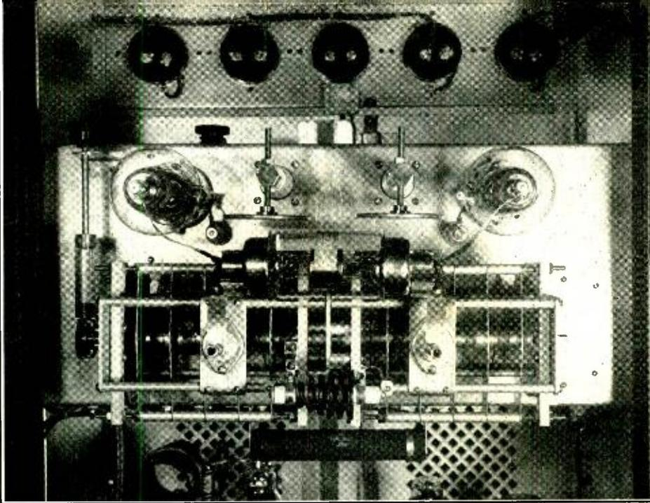
Looking down upon the final amplifier stage with its plate coil removed. In this photograph the amplifier itself has been removed and turned upon edge on the shelf brackets.
