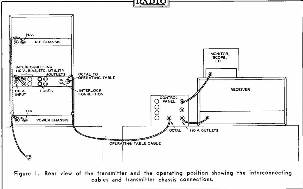
Figure 1. Rear view of the transmitter and the operating position showing the interconnecting cables and transmitter chassis connections.
