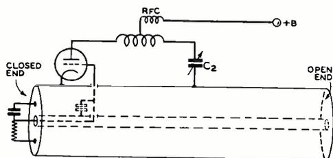
Figure 1. Semi-schematic of the coaxial-line oscillator.
