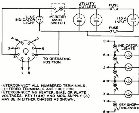
Figure 2. Simplified schematic of the interconnecting wiring at the transmitter.
