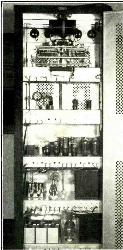
Rear view of the transmitter with the doors opened. Power supplies occupy the lower decks, the modulator and control relays are on the second shelf, with the speech equipment and a low-voltage power supply on the third shelf.
