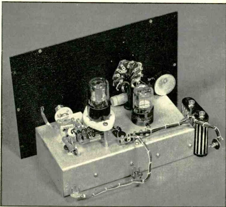
Looking down on the transceiver with cabinet removed. The flexible lead terminated in a solder lug must be unfastened from the lower antenna feed-through insulator before the unit can be slid out of the cabinet.
