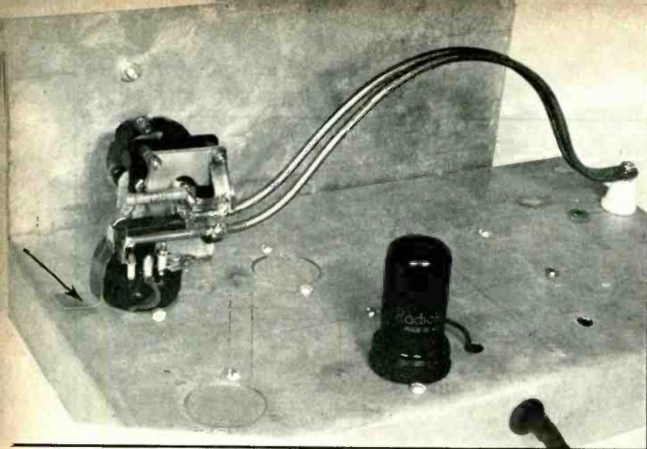
Figure 1. Rear view of the experimental model superregenerator. Arrow points to the balancing capacity discussed in the text.
