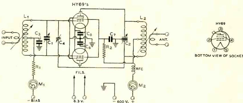
$C_1$ —100- $\mu$ fd. tuning condenser, 0.030" spacing
