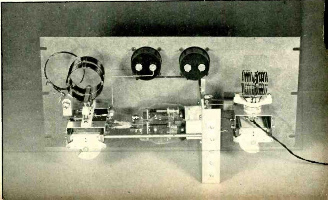
her acted as a very good t.p.t.g. self-excited oscillator. After making several tests it was ascertained that the gain of the amplifier was so high that the very low residual grid-to-plate capacity of the HY-69's was great enough to cause self-oscillation.
