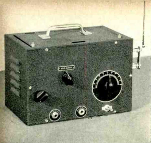
All ready to go for a walk. From a good vantage point, this little self-contained 112-Mc. transceiver has a range of several miles. The vertical rod radiator is supported as shown. Two bolts are soldered to the front lip supporting the hinged lid, and by removable thumb screws the lid either may be held down tightly for carrying by the handle or opened for access to the "works".
