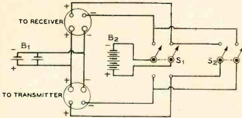
Connections inside the portable battery box.
