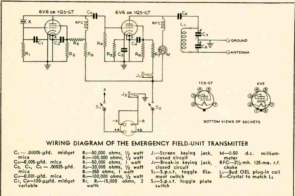
WIRING DIAGRAM OF THE EMERGENCY FIELD-UNIT TRANSMITTER
