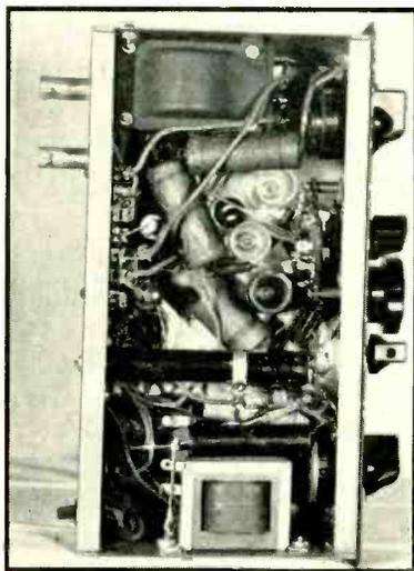
Figure 3. Underchassis view. The bleeder resistor is mounted away from the chassis on metal brackets. The filter choke is mounted under the power transformer with the filter condensers tucked on top. The audio transformer is mounted on the other end of the chassis.
