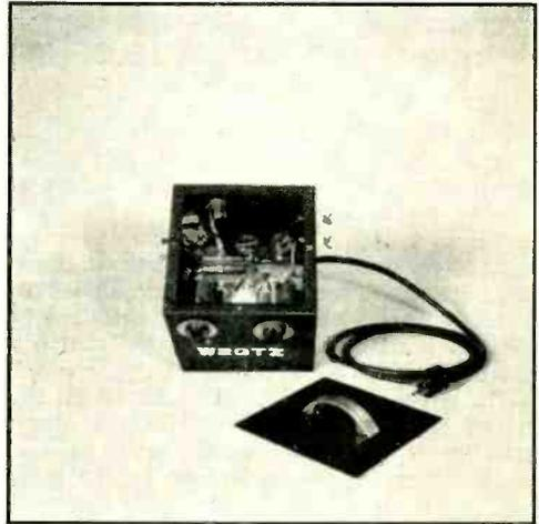
Figure 4. Looking down into the battery-power field transmitter. The bottom plate of the cabinet housing this transmitter is also removable to allow changing of the coil and crystal.
