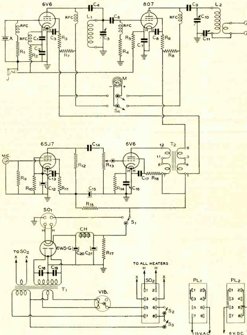
WIRING DIAGRAM OF THE UNIVERSAL A.C.-D.C. 'PHONE-C.W. TRANSMITTER
