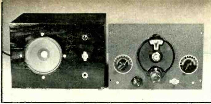
This simple 20-160 meter superheterodyne may be constructed for about \$20, and will give excellent results. The power supply and speaker are housed in a plywood box of the same approximate size as the receiver proper.
