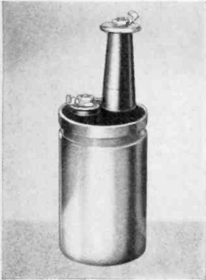
the standard Aerovox Type '12 round-can barrier-cap units, except that one terminal is a short screw post. The other is a tall insulator post with corona shield at top. The cover assembly is a one-piece ceramic cap, with the can top spun over a rubber gasket and the cap for a perfect hermetic seal. The arrangement of terminals, corona shield and ceramic cap minimizes surface leakage, corona losses and probability of voltage breakdowns even at extreme altitudes.
