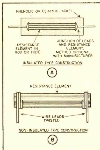
Fig. 1. Resistor construction
