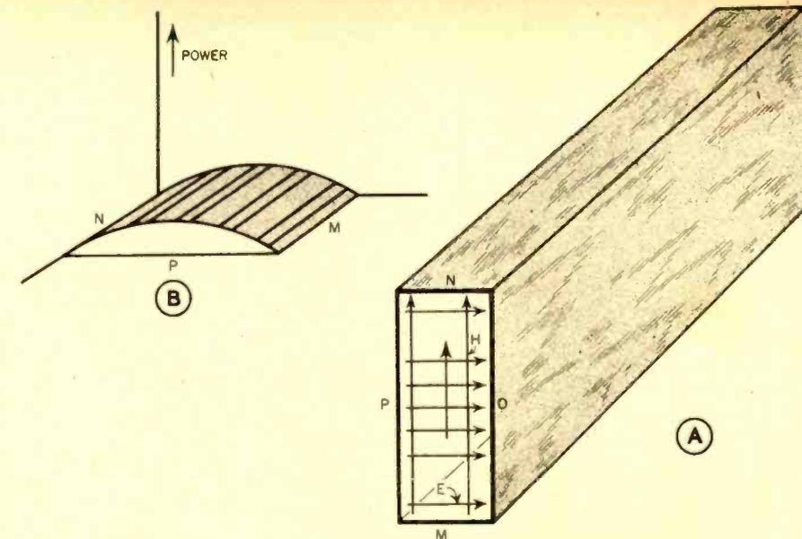
Fig. 4. Instantaneous values of  $E$  and  $H$  fields at exit of an open-ended wave guide operating in the  $TE_{1,0}$  mode
