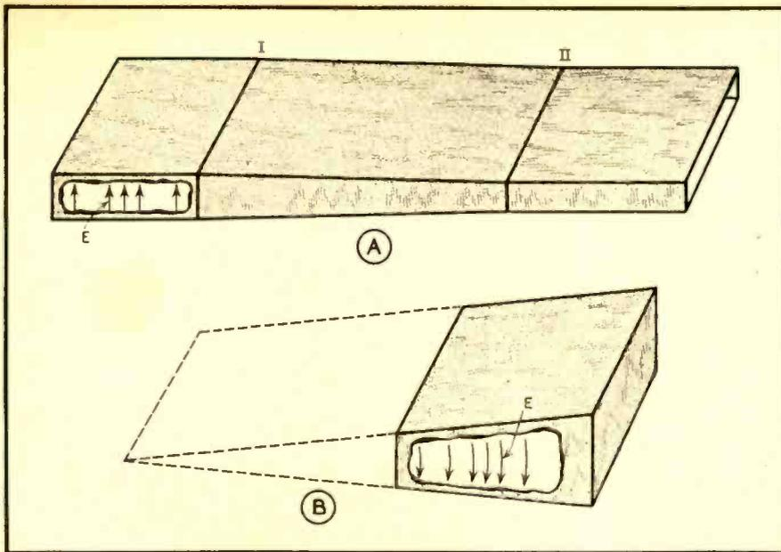
Fig. 5. Tapered section to connect wave guides of different sizes
