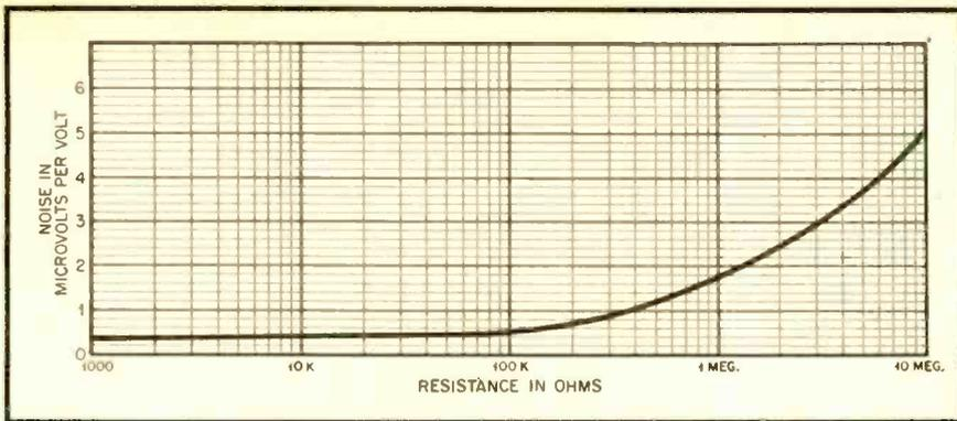
Fig. 5. Noise characteristics of typical 1/2-watt resistor
