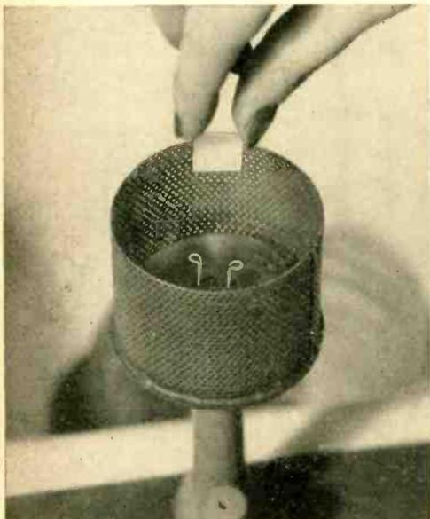
THIS is an actual photograph of the centrifugal air drier, or "spinner," used in Bliley production to facilitate clean handling of crystals during finishing and testing operations. Quartz blanks are dried in 5 seconds in this device which is powered with an air motor and spins at 15,000 r.p.m.
