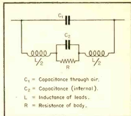
Fig. 6. Equivalent circuit of composition resistor at high frequencies
