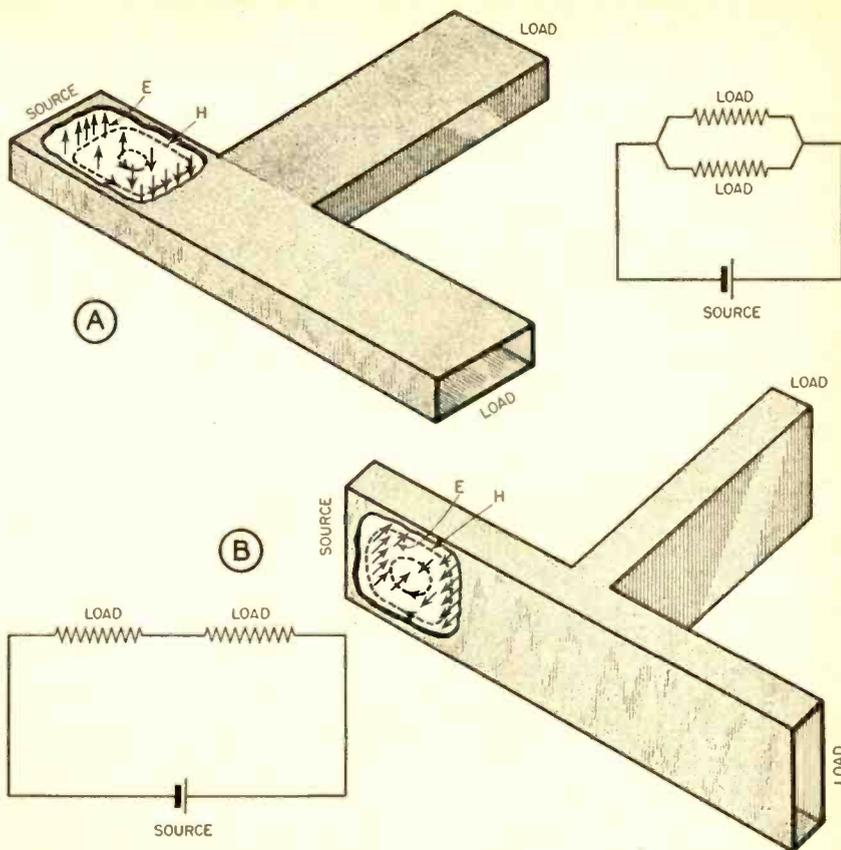
Fig. 1. Shunt and series wave-guide-connected loads across a single source
