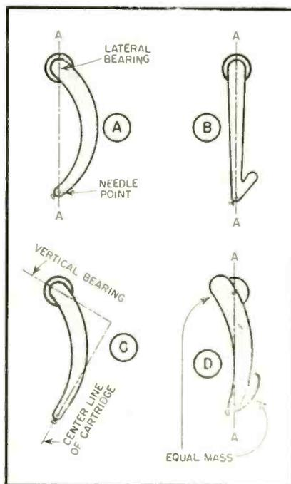
Fig 3. Typical manually-operated tone arm designs. See text
