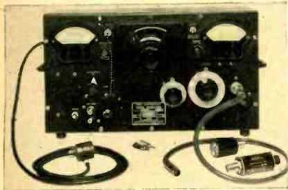
accurately calibrated attenuator network which allows control from 1 microvolt to 20,000 microvolts.
