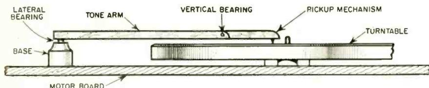
Fig. 1. Side view of manually operated tone arm design
