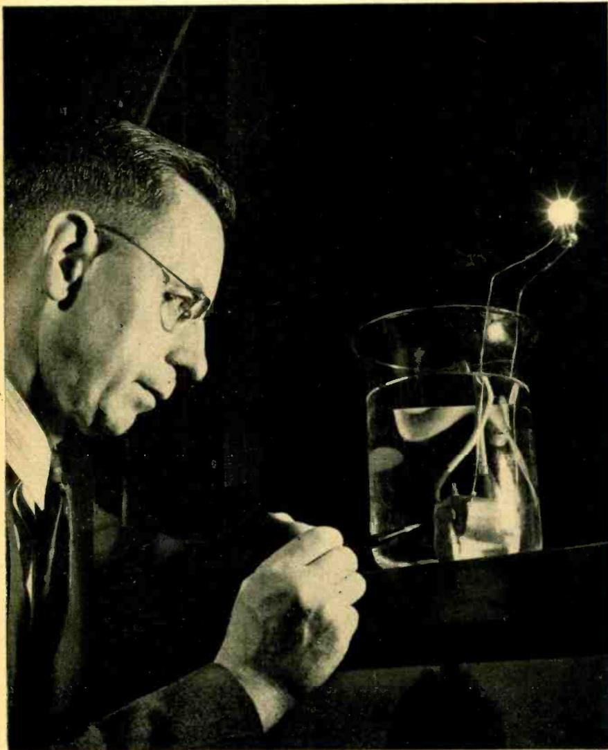
Power to operate the glowing lamp is supplied by a submerged transformer, impregnated with Fosterite. Demonstrated by Dr. C. F. Hill of Westinghouse
