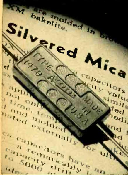
• Aerovox silvered mica capacitors are designed for the most critical applications requiring precise capacitance values and extreme stability. Silver coating applied to mica and fired at elevated temperatures. Unit encased in molded XM low-loss red bakelite for silvered-mica identification.
