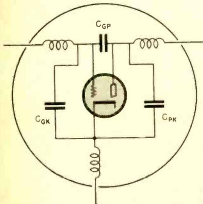
Fig. 12. Equivalent circuit of triode when operated at uhf. Capacitances and lead inductances must be kept low
