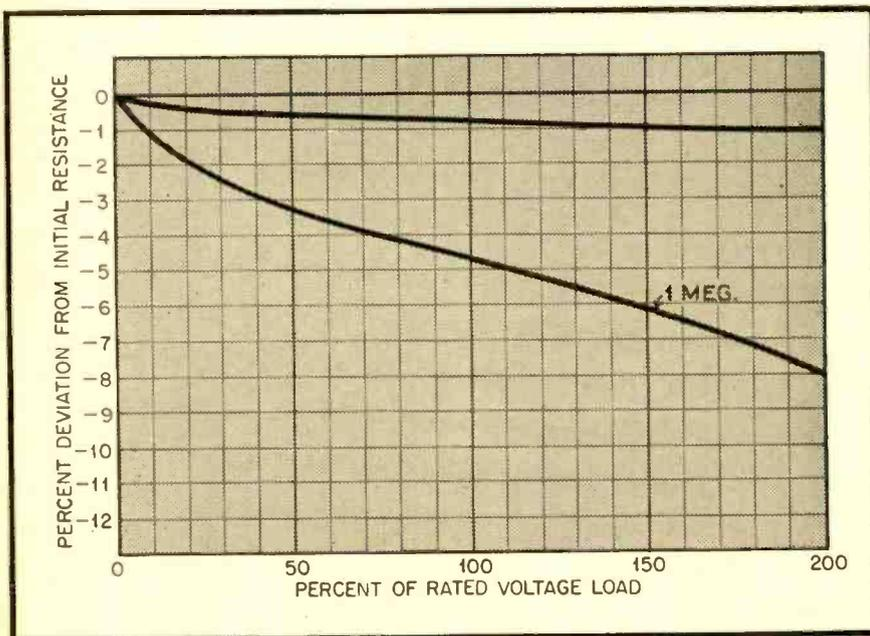
Fig. 4. Voltage characteristics of ½-watt, 10,000-ohm resistor (upper curve) and 1-megohm resistor expressed as percentage resistance deviation
