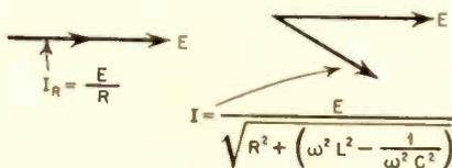
Phase angle of current in series tuned circuit
