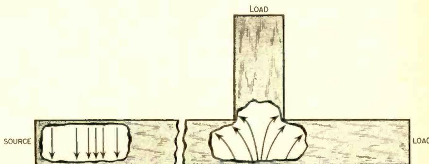
Fig. 2. Simplified illustration of a series T wave guide junction, showing how the electric field is distorted at the junction
