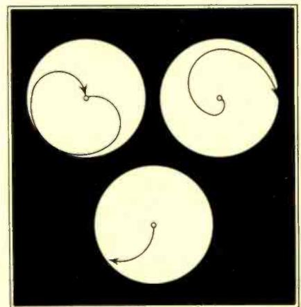
Fig. 13. The electron stream in a magnetron describes a curved path which varies with anode potential and magnetic field strength
