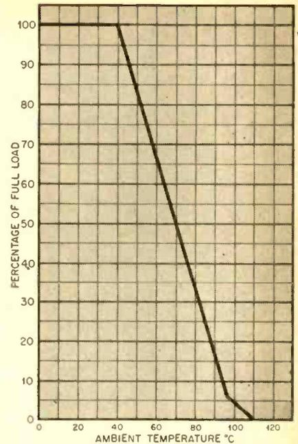
**Fig. 2.** Graph showing proper derating for operation of composition resistors at elevated temperatures
