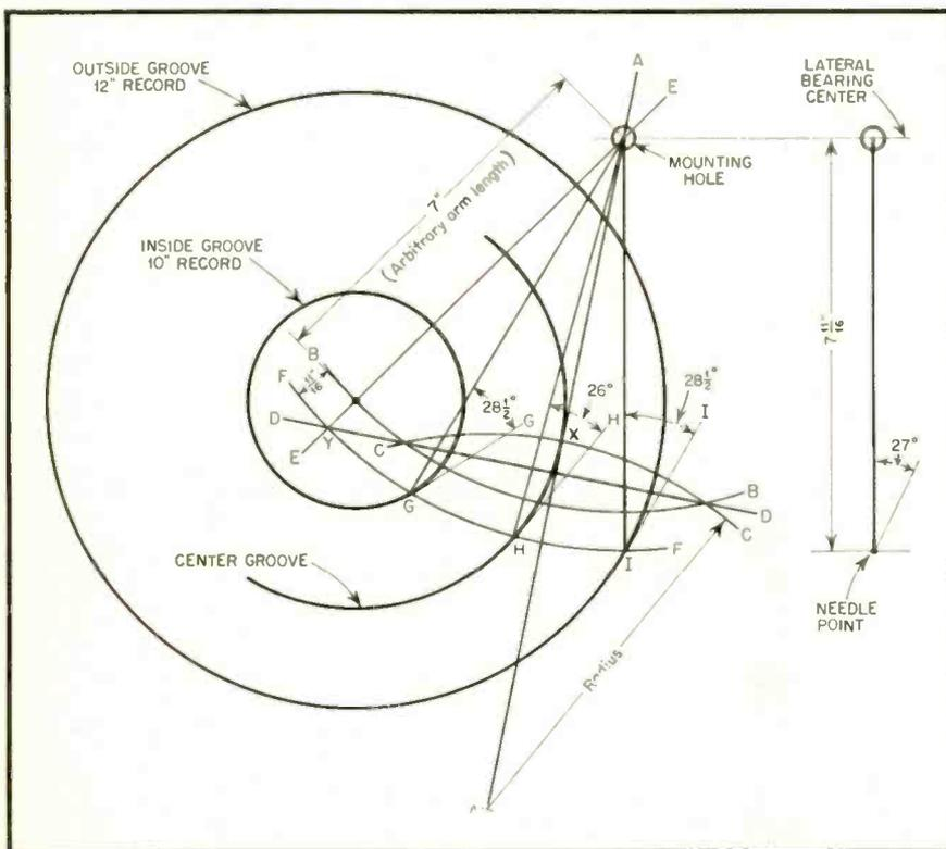
Fig. 4. Method of laying out tone arm mounting. See text
