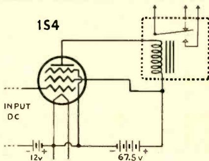
★ The book says a 1S4 should operate into a 5,000 ohms plate load when used with a 67.5 volt plate supply. Bear in mind that we wish to put as much power as possible into the relay under conditions of minimum signal.
