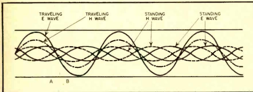
Fig. 3. A section of a wave guide or other type of transmission line carrying a traveling wave and a standing wave. The curves represent the field strength in the guide by their distance above or below an imaginary center line. As a function of time, the traveling waves move to the right; the standing waves take on successive values between the extremes shown
