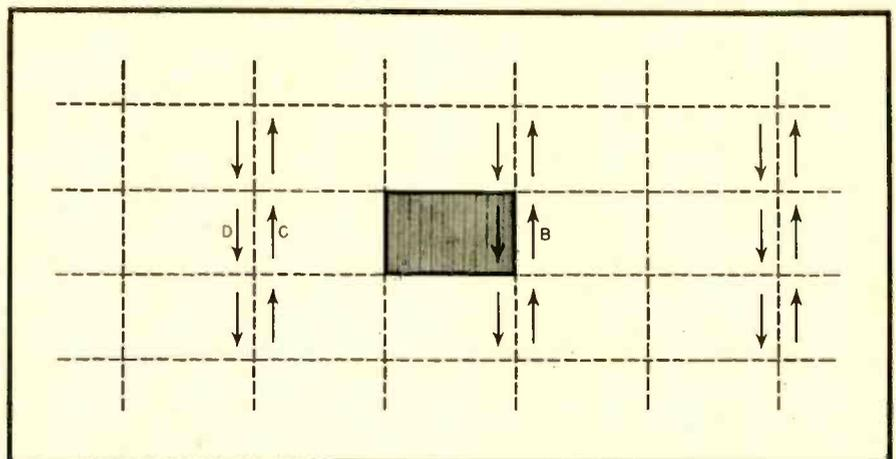
Fig. 8. Image array to simulate field in a rectangular wave guide arising from excitation by a single electric dipole
