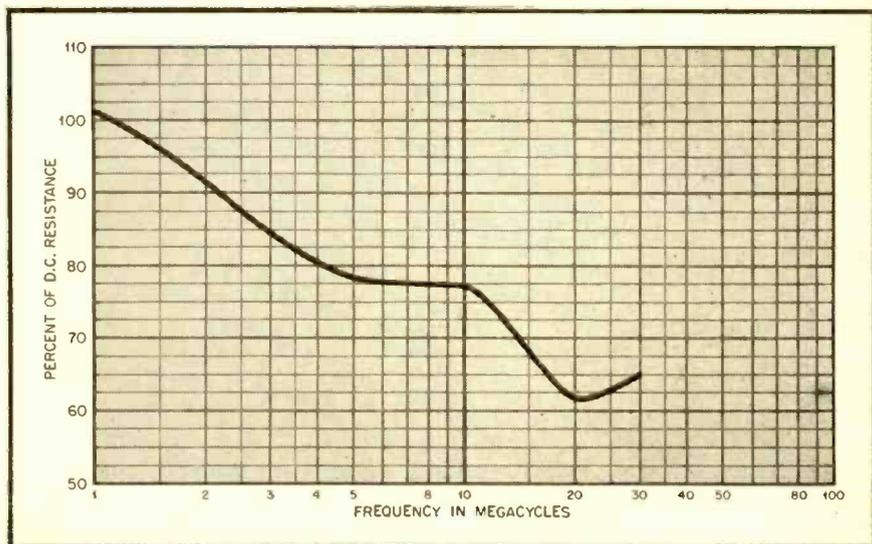
Fig. 7. Frequency characteristic of 0.1-meg., 1/2-watt resistor
