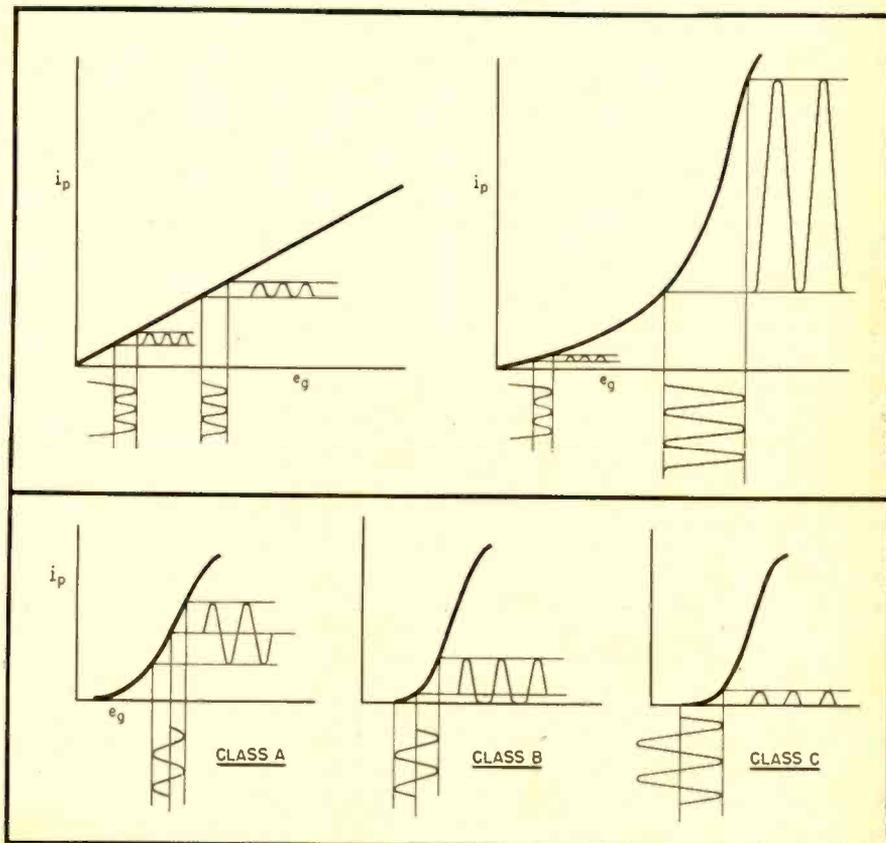
Fig. 10 (above). Comparison of linear and square law detectors and, below, (Fig. 11) operating points for class A, B, and C amplification
