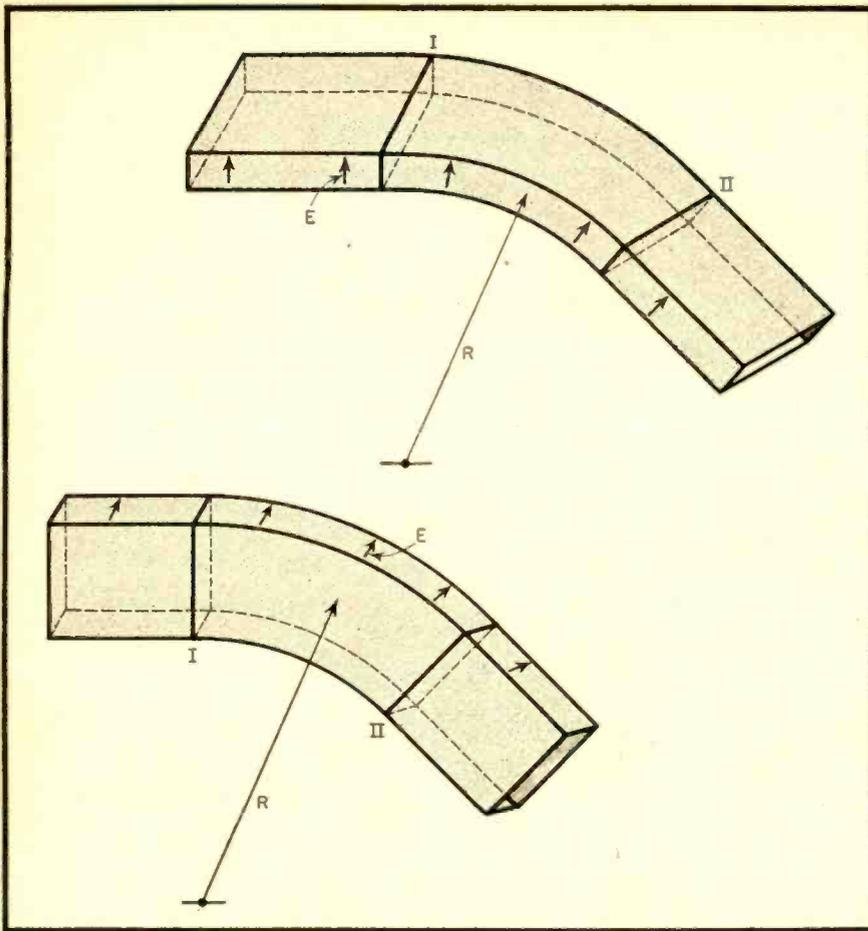
Fig. 6. E and H bends in a wave guide
