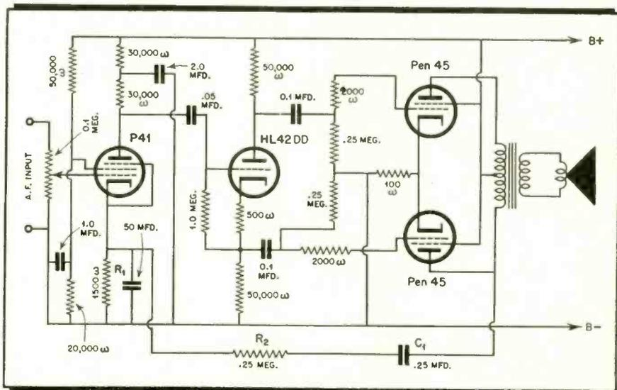
Fig. 4 Negative feedback amplifier
