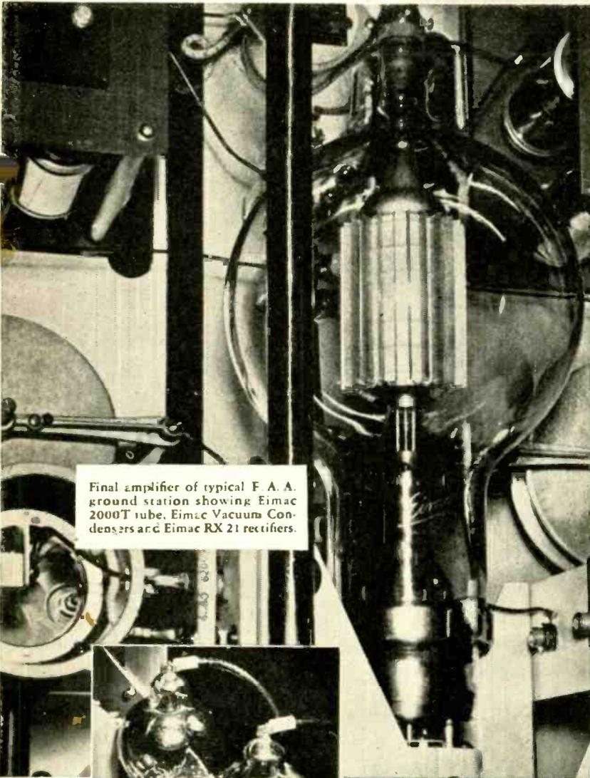
Final amplifier of typical F. A. A. ground station showing Eimac 2000T tube, Eimac Vacuum Condensers and Eimac RX 21 rectifiers.
