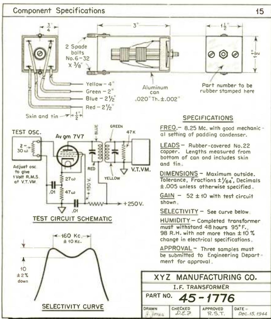
Fig. 1 Representative specification sheet
