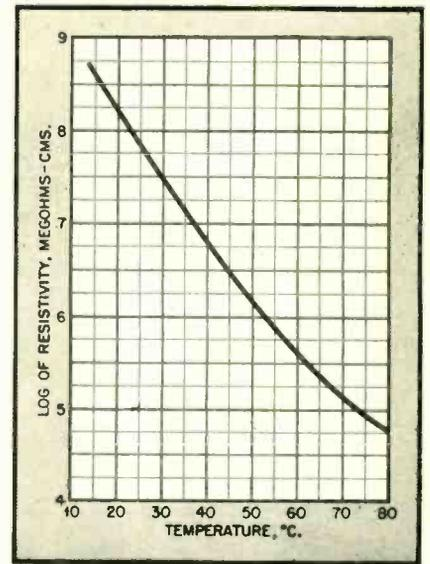
Fig. 5 Temperature insulation resistance characteristics of polyvinyl chloride
