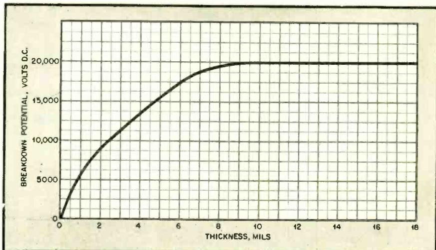
Fig. 1 Breakdown potential is a function of thickness
