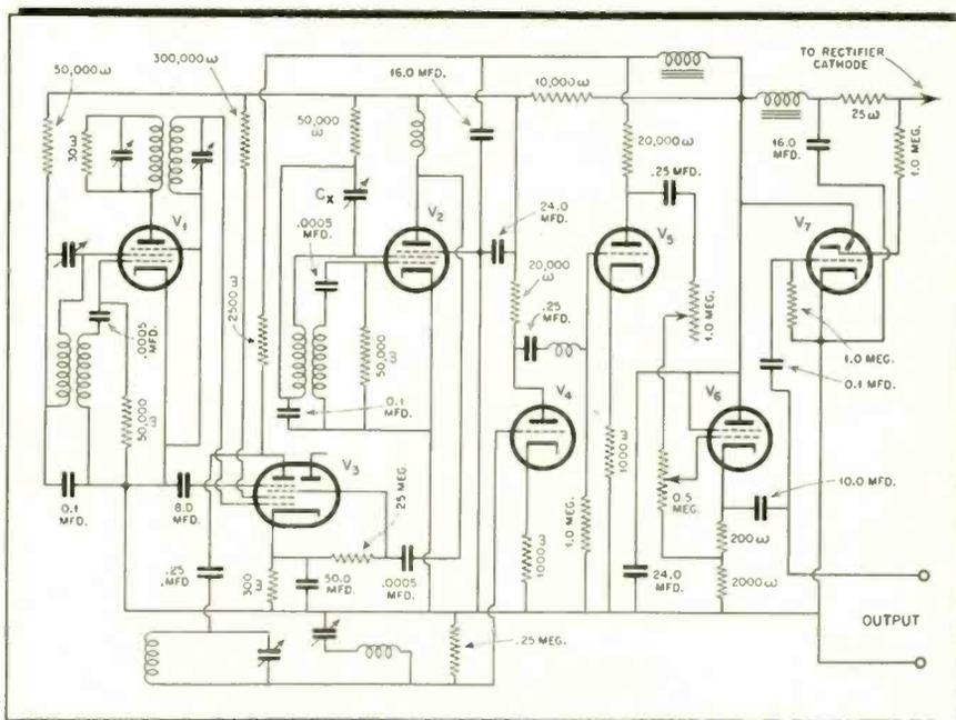
Fig. 5 Audio frequency oscillator
