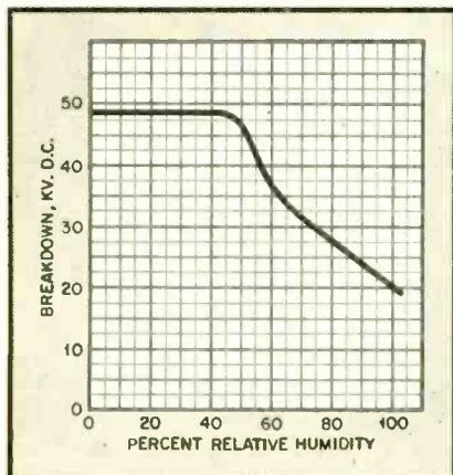
Fig. 4 Breakdown as a function of humidity
