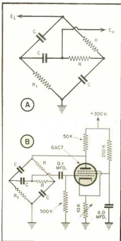
Fig. 1 In (a), typical fundamental circuit, and (b) application to unbalanced bridge oscillator
