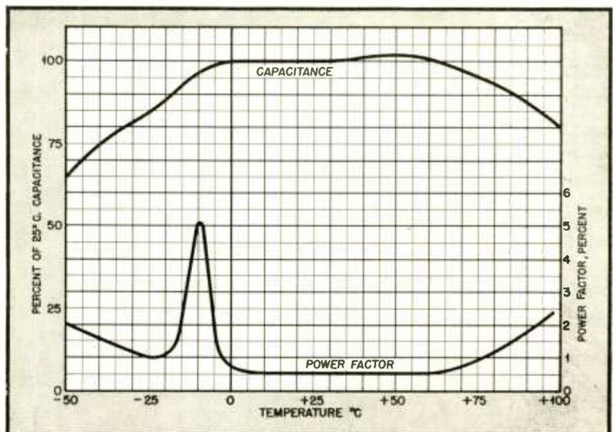
Fig. 8. Variation of dielectric constant (capacitance) and power factor at various temperatures, using a typical capacitor impregnant
