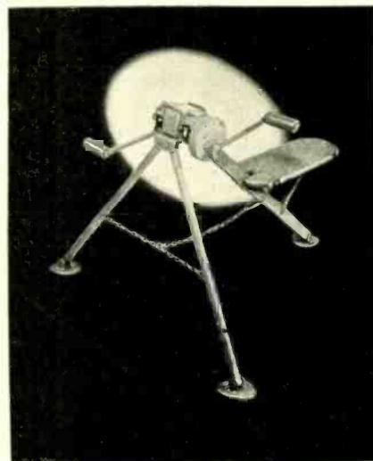
One man, seated on the seat which folds up when not in use, turns two cranks (of special construction to prohibit their being detached through anti-axial strains) which are immediately demountable with no tools required. Drive is by means of a gear train, one of which is bakelite to create a smoother and quieter operating unit.
