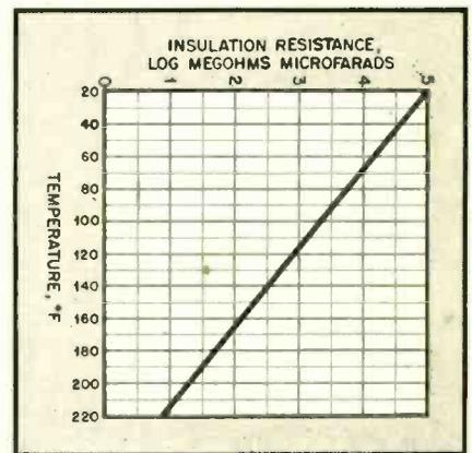
Fig. 6 Insulation resistance-temperature characteristics of mineral oil capacitors from American War Standard C75.16)
