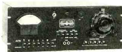
circuits are provided, one at 600 ohms for audible program monitoring, and the other a high-impedance circuit that gives a faithful reproduction of the audio envelope for distortion and noise measurements. The linear rectifier is designed for use at a low power level, so that the problem of coupling to the transmitter is greatly simplified. The required r-f power input is only 0.5 watt, far less than that necessary to operate pre-war modulation monitors.
