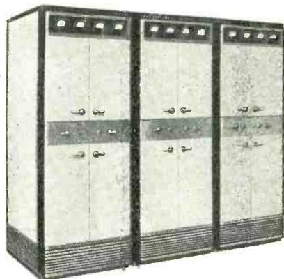
The basic unit of Federal's new FM Broadcast Transmitters is the exciter which generates the initial radio frequency power, in itself, a complete 250 watt transmitter. In this unit are included the frequency modulation system, center frequency stabilization system, and the radio frequency multiplier and output stages. The 250-watt output of the exciter unit is stepped up to 1, 3, 10, or 50 kilowatts by a Power Amplifier Unit or series of such units.
