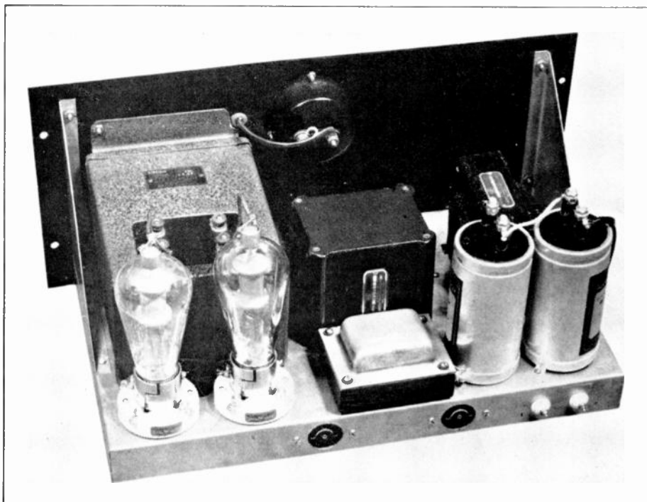
High and low voltage transformers, H.V. choke and H.V. condensers are mounted on the lower deck.
