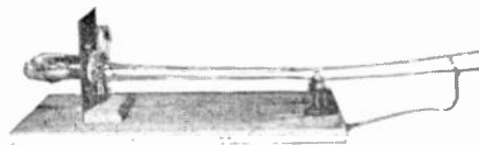
Fixed tune high-C oscillator with tuned-line plate tank
