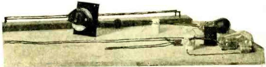
Arrangement of Parallel Wire Apparatus.
