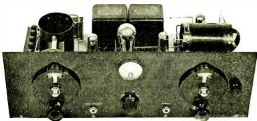
Panel View of Browning-Drake Receiver.
