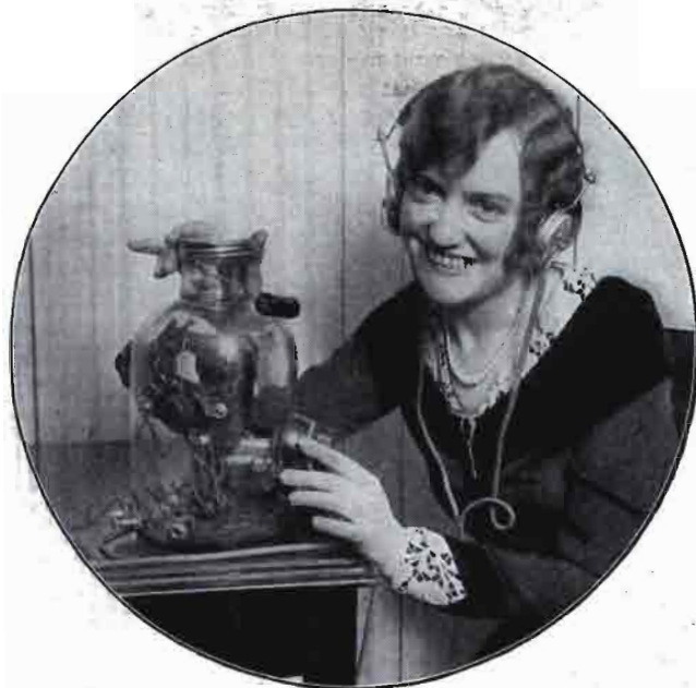
A radio set built in a glass jar containing one tube. The set was submitted by Harry De La Force, of Montreal, Canada, and exhibited at the Chicago Radio Show.
