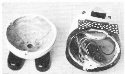
The two halves of the case can be clearly seen, the bottom half showing the wire frame. Photograph (right) shows a close-up of the wiring inside the top half of the case.
