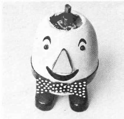
Two screws remove the brim and free the potentiometer.
