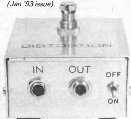
(Below) Black rub-down lettering applied directly on the aluminium box and covered with protective, clear varnish - Soft Distortion Unit (Jan '93 issue).
