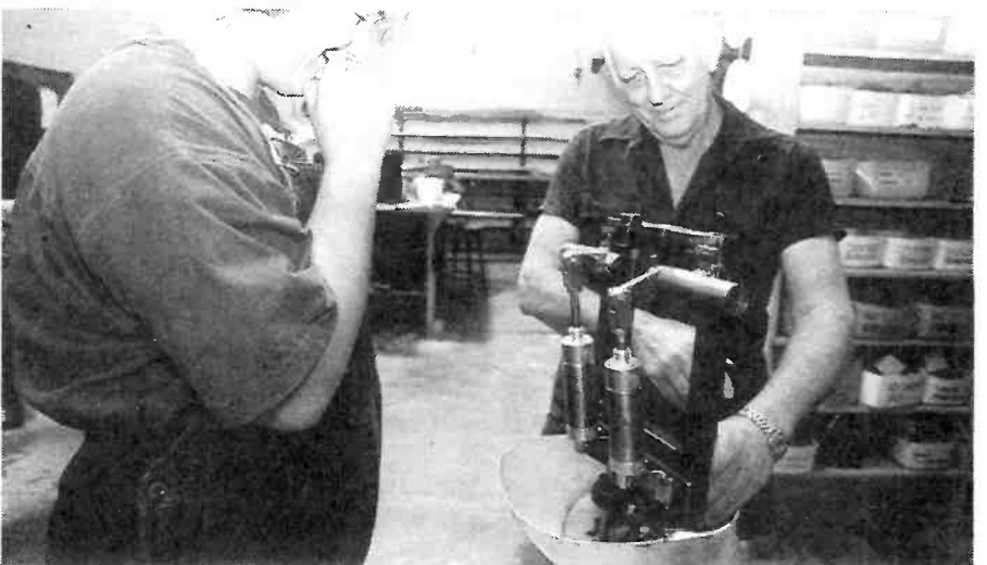
An internal armature for an animatronic puppet being built at the Sally plant.
