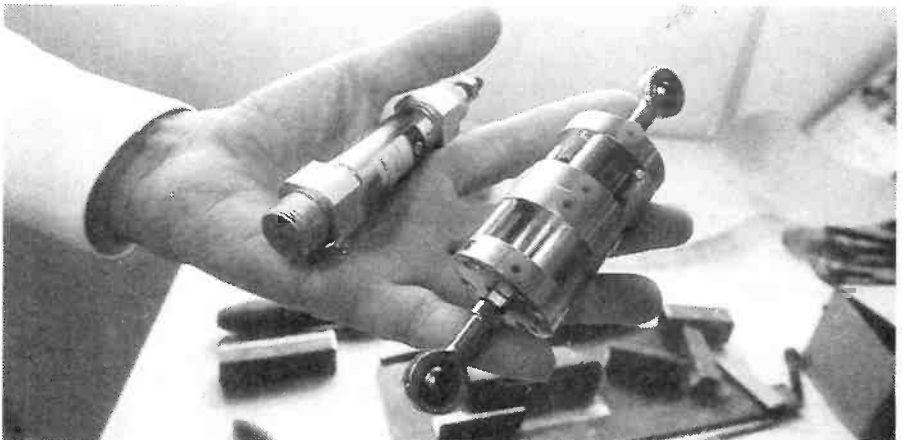
Readily available, standard pneumatic parts are used in the construction of animatronic puppets.
