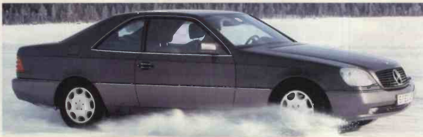
Fig. 1. A car travelling on ice at 45mile/h is kept steerable and stable by the new Electronic Stability Program from Mercedes-Benz.
