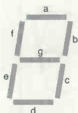
Figure 2: the segments of the LED display
