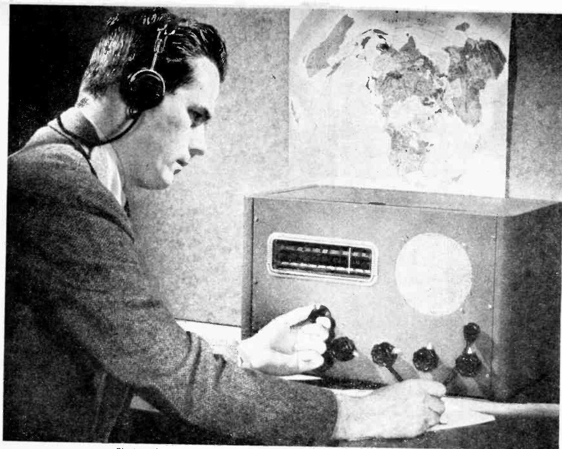
Elusive short-wave signals often come in best at night, so headphones are built into this two-band superheterodyne for midnight DX listening. Flicking a couple of switches, however, brings in the full broadcast band at loudspeaker volume.
