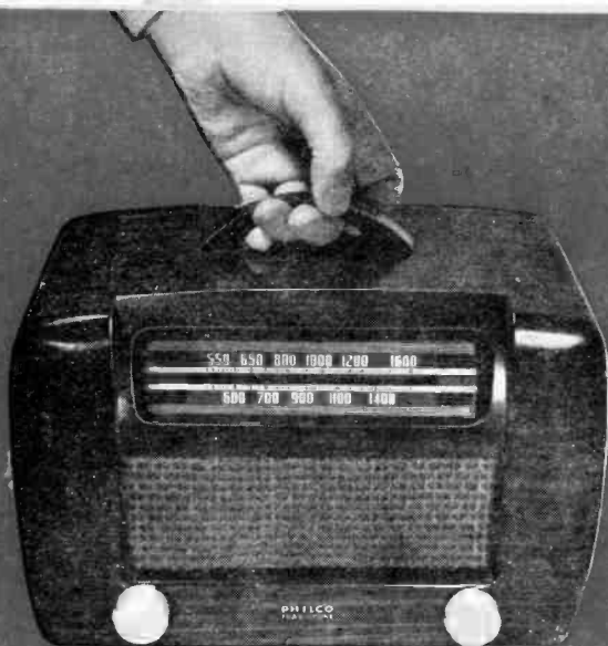
New tubes and some minor changes turn this midget radio into a self-powered portable—and back again.
