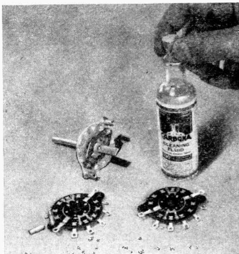
Dirty wave-band switches often cause intermittent reception. Clean them with carbon tetrachloride.
