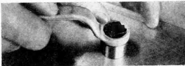
Drawing up the bolt with a wrench brings the cutter and die in contact with the chassis and shears out a clean, precise socket opening.
