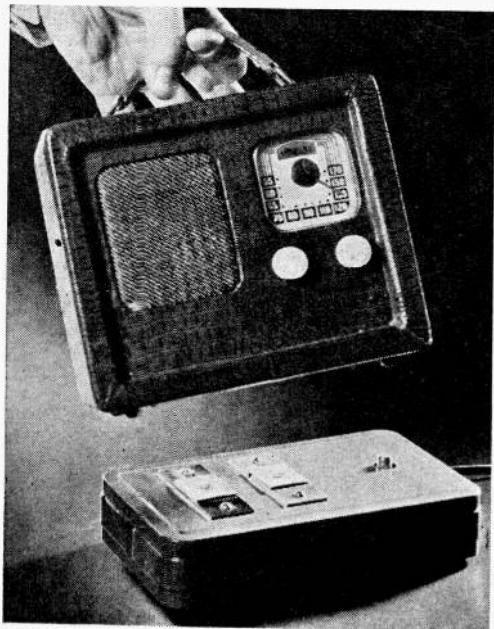
Listen all you want without draining those expensive batteries. The little box supplies B voltage; weight of the portable turns it on.
