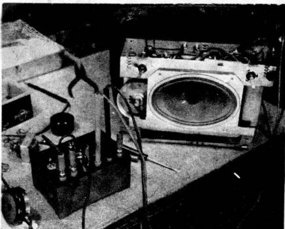
The pocket laboratory quickly tracked down the fault in this receiver. Used for stage-by-stage checking, it's a valuable service tool.
