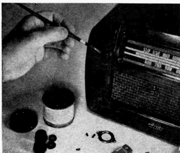
Paint the inside of the opening black to give greatest definition to the tube pattern. The decorative bezel (foreground) goes on last.
