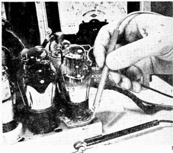
2. Test-point adapter, easily made from wafer tube socket, allows you to check voltages at the tube instead of turning chassis over.
