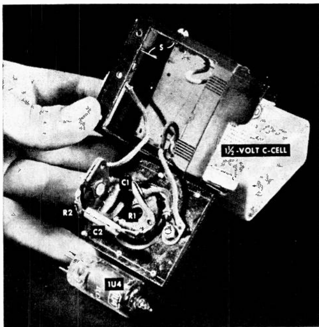
Layout and wiring of the parts is simple. The thing to watch for is clearance of the tube and socket in the 2"-wide opening in the case.
