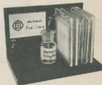
Hitachi's experimental model portable methanol fuel cell
