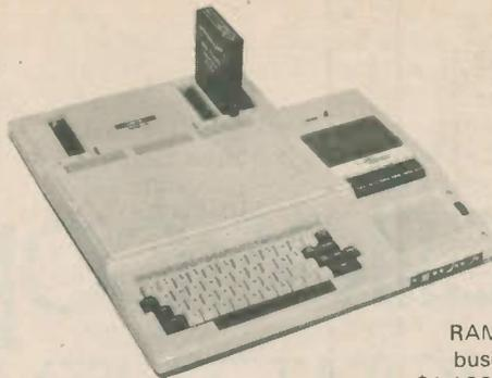
The Imagination Machine II with 27K RAM, 14K ROM, is a small business system with r.r.p. \$1,199. It features up to eight video colours, sound synthesiser, BASIC or 6800 m/c, object orientated and point resolution graphics. Photo shows floppy interface module inserted. *Courtesy of APF Electronics.*
