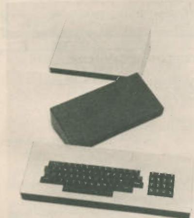
The consoles are of all aluminium construction and incorporate ventilation slots in both rear and bottom panels with a gasket fitted between the panels to reduce vibration.
