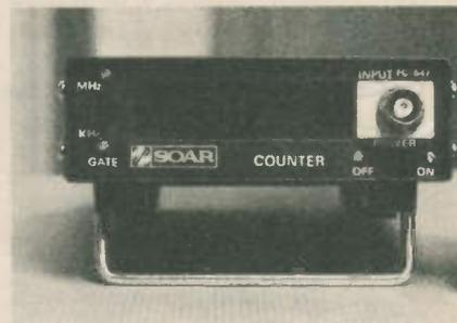
The unit which measures only 100x32x120mm has a frequency range of 10Hz to 50MHz and can measure up to 500MHz with a prescaler. Powered by either 4 penlight batteries or an external d.c. supply (8 to 11V) the instrument has a 4 digit display and a resolution of 10Hz/10kHz with a maximum input of 20V.
