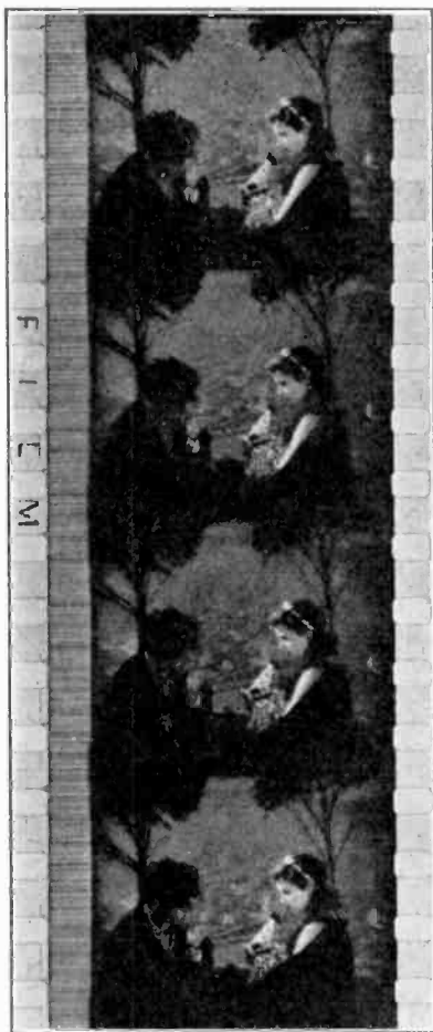
Fig. 1. Section of Movietone Film
