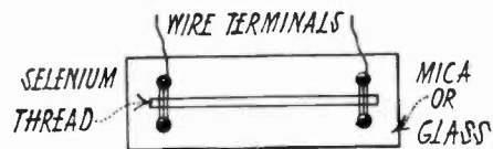
Fig. 1. Construction of Selenium Cell
