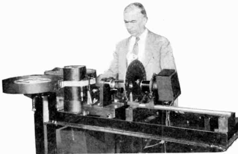
Radio Movie Projector as Operated by Frank Conrad
